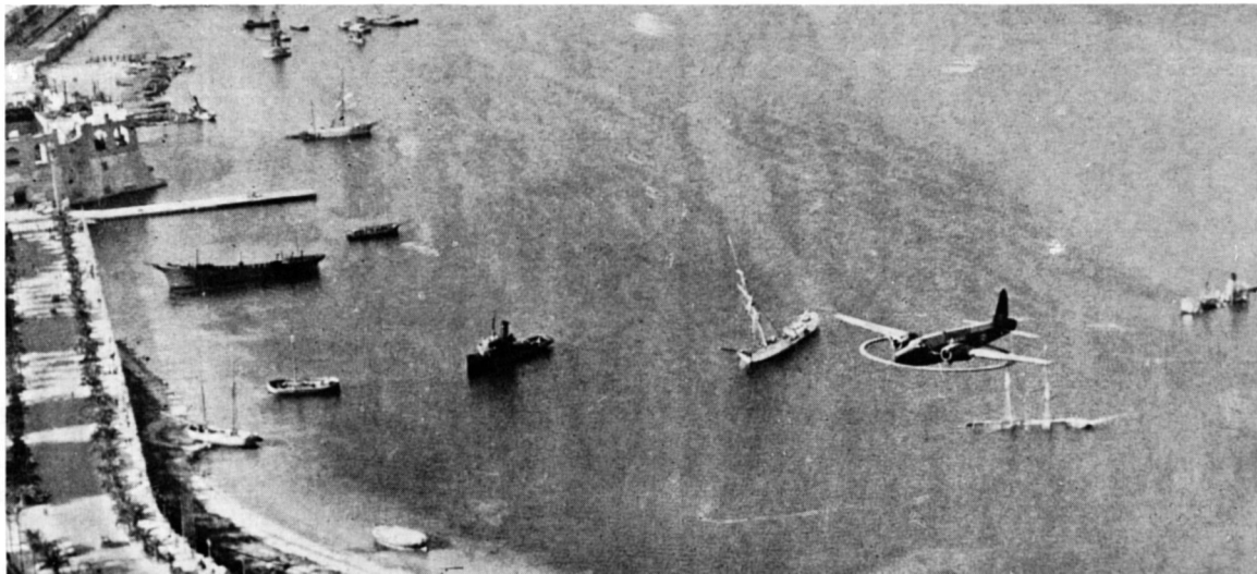
Mk. I, HX682, one of several machines fitted with a 48-foot dural hoop energised by an auxiliary motor mounted in the fuselage. Appearing in January 1940, this modification was intended to detonate magnetic mines when the aircraft flew at a low altitude over mined channels. It was highly successful.
