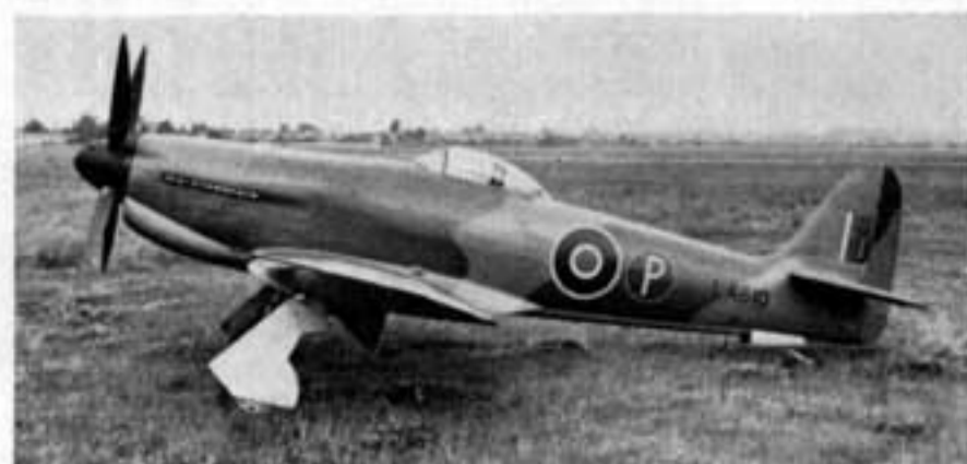
LA610 finally acquired a Sabre VII engine and, with a top speed of 485 m.p.h., was the fastest Hawker piston-engine aircraft until the advent of the American racing Sea Fury conversions of 1966. (Photo: Hawker Aircraft Ltd., Neg. No. IFG3)
