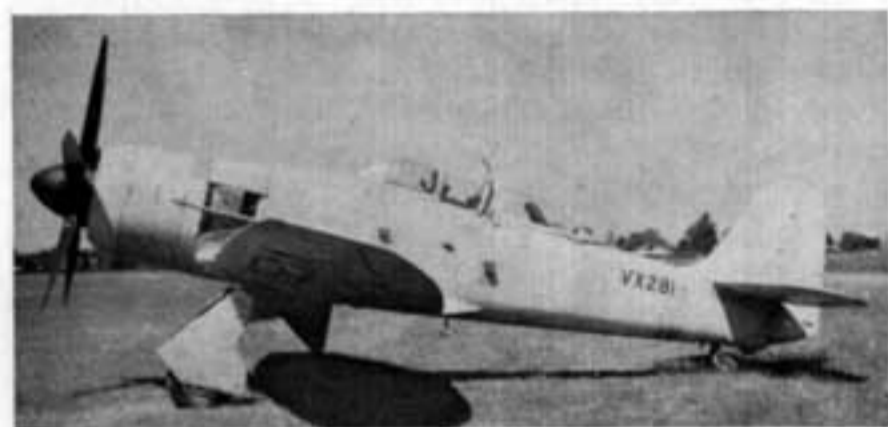
The second production Sea Fury 20, VX281, in overall pale green factory finish, sans hook but with Hawker periscopic sight added.
