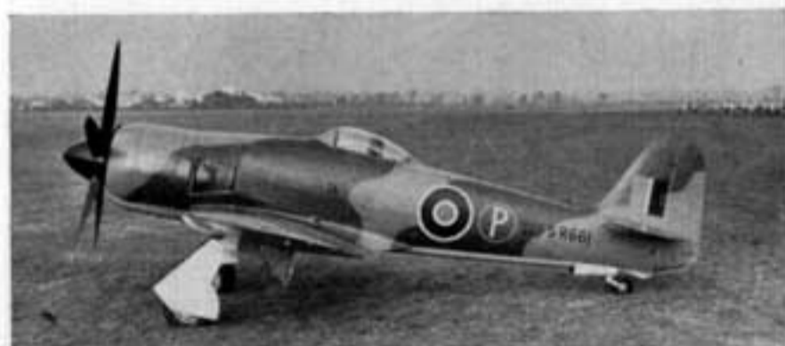
SR661 with full-size fin and rudder. (Photo: Hawker Aircraft Ltd., Neg. No. SFG8)
