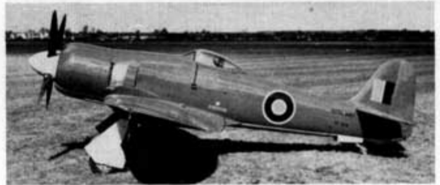
Early production Sea Fury Xs were characterised by 4-blade Rotol propeller and short hook. (Photo: Hawker Aircraft Ltd.)
