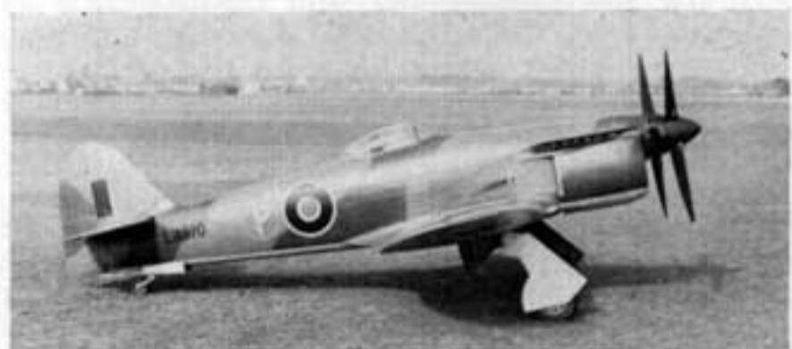
Third F.2/43, LA610, was initially powered by a Rolls-Royce Griffon 85 driving Rotol contraprops. This was something of an insurance against further shortcomings of the Centaurus and Sabre engines. (Photo: Hawker Aircraft Ltd.)
