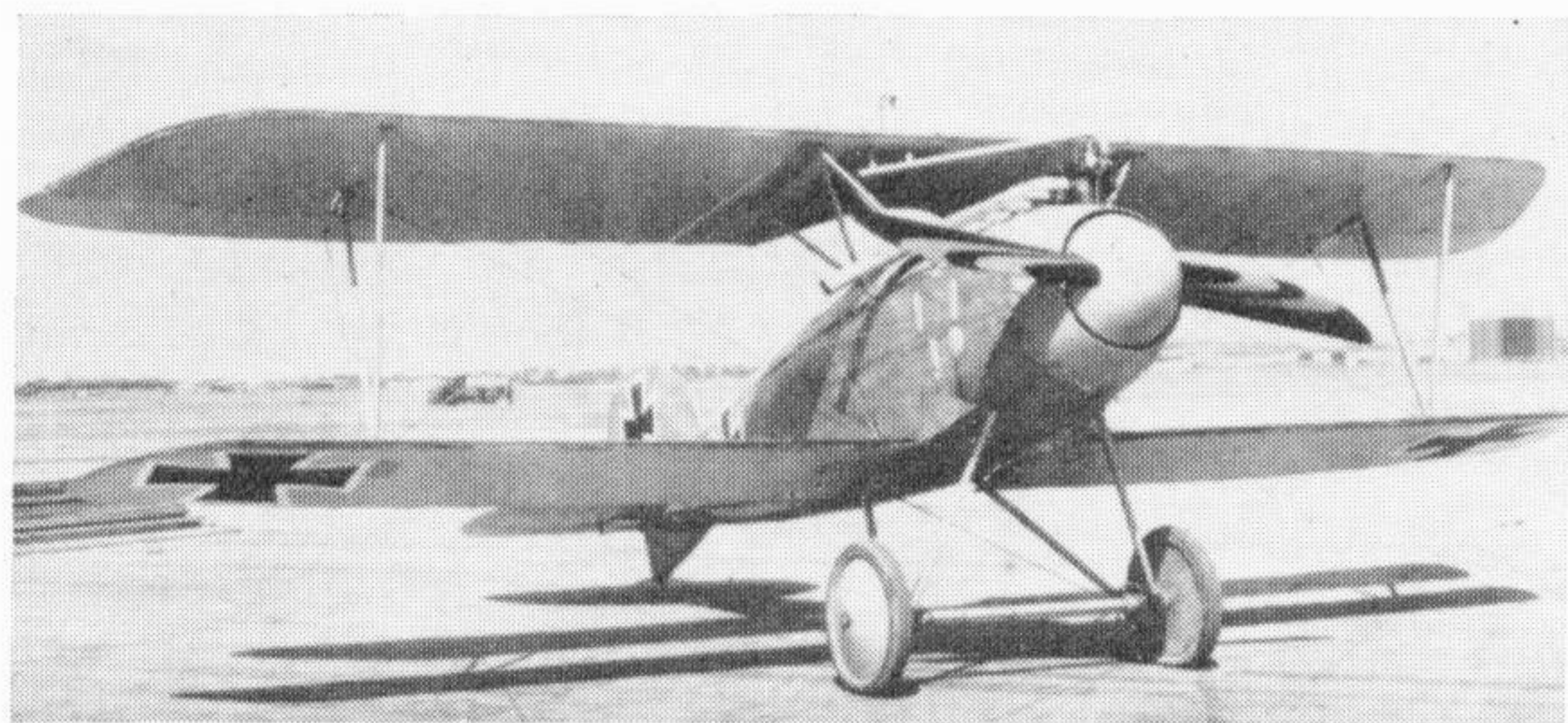
Late production Albatros D III with D V type rudder. The contrast of the airscrew laminations is clearly shown.
