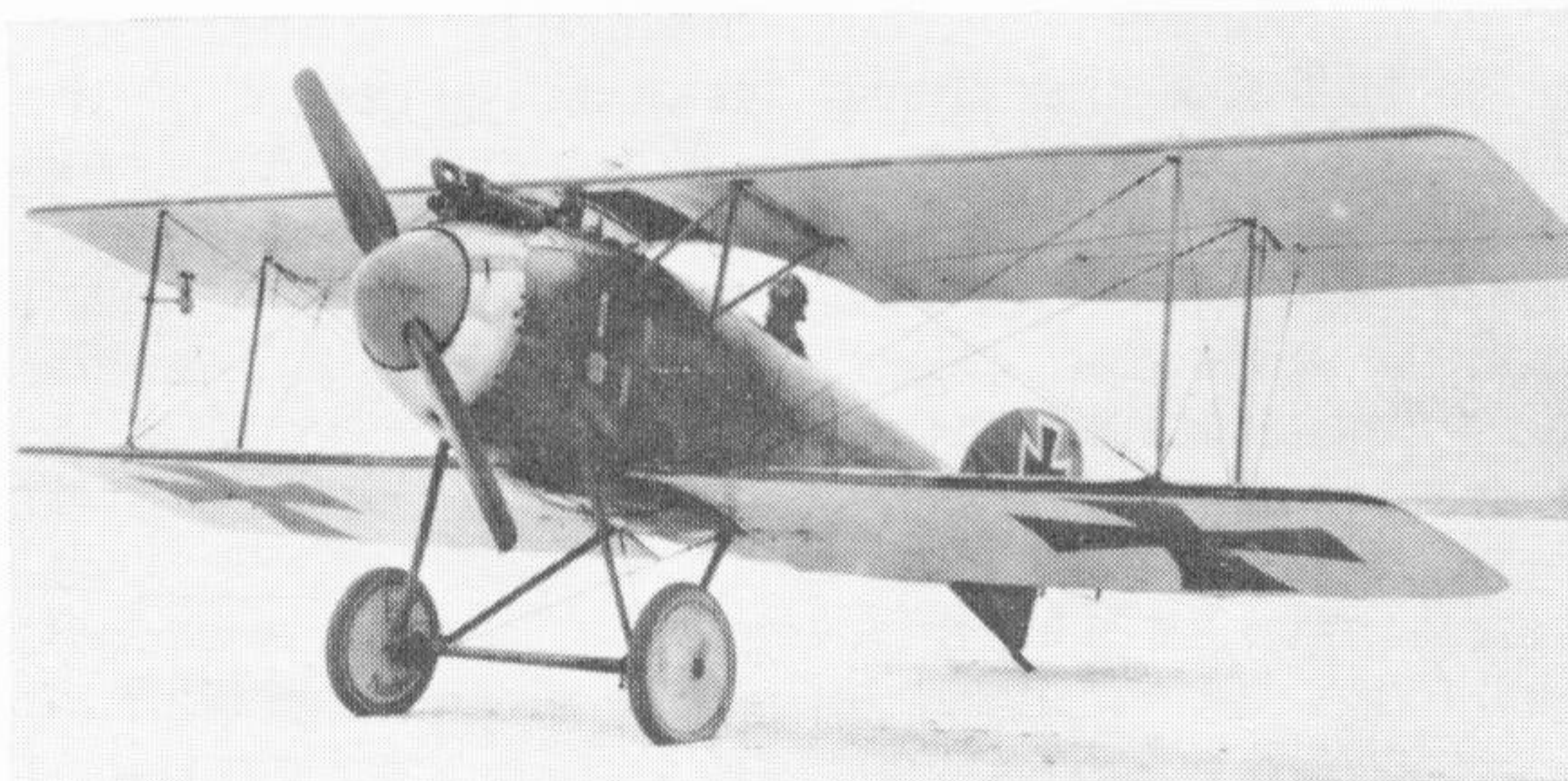
Later type of Albatros D II with flush radiator in centre of upper wing. The racier appearance resulting from the reduced gap is noticeable when compared with the D I. (Photo: Egon Krueger)
