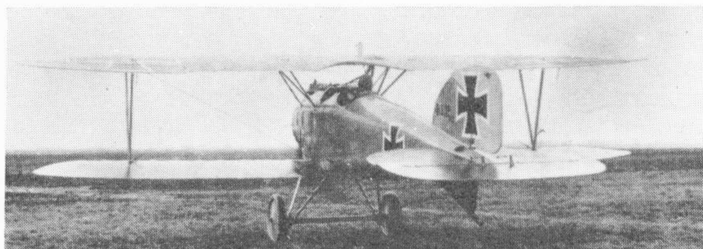
Albatros D III D 632/17; an excellent view of the aircraft taking off. The modicum of "down" elevator to lift the tail off the ground and the slight starboard rudder to correct swing are noteworthy. (Photo: Egon Krueger)
