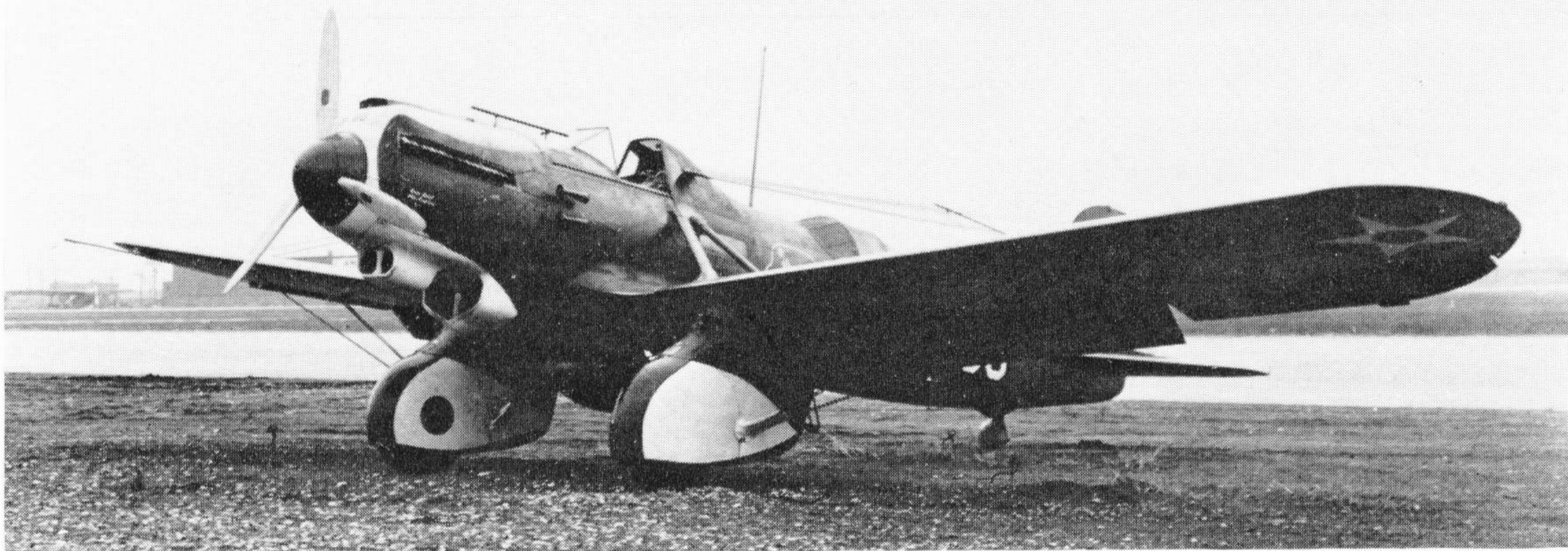
Curtiss Y1A-8 of the 13th Attack Squadron. Aircraft number, "60", is atop spinner and on rear fuselage.
