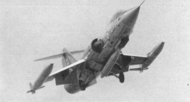
Fine take-off study of CF-104 (12739) of the R.C.A.F.'s No. 3 Wing; note emblem of 4th A.T.A.F. on intake, and training weapons container on centreline station.
