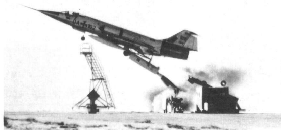
A Luftwaffe TF-104G and (above) a ZELL take-off during tests by Lockheed at Edwards A.F.B., California.
