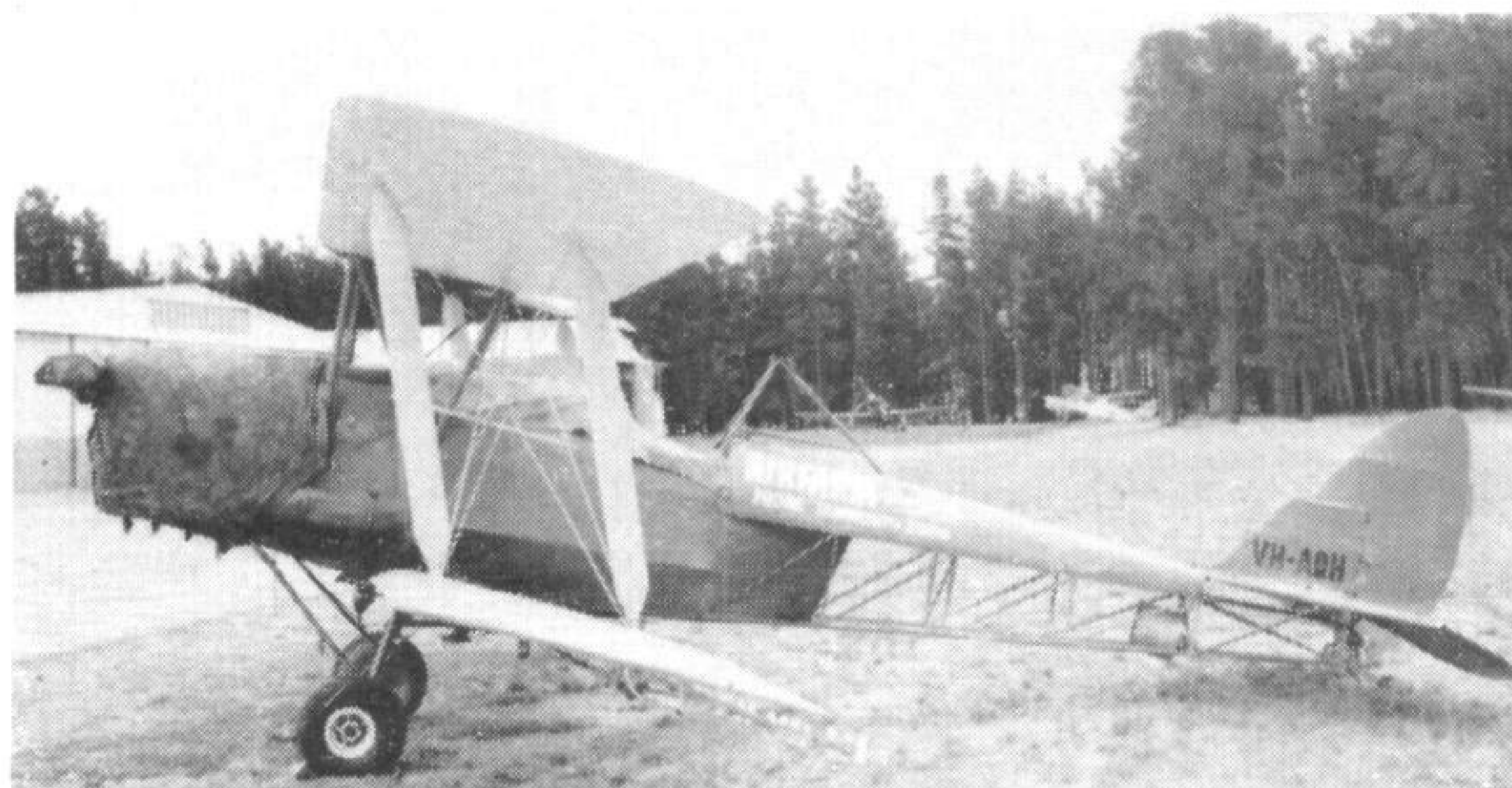
Left: Airfarm's VH-ADH, ex A17-680, operates with stripped rear fuselage. Right: Bain Bros.' ZK-AIN, ex NZ775, with wind driven pump and under-wing spray bar.
