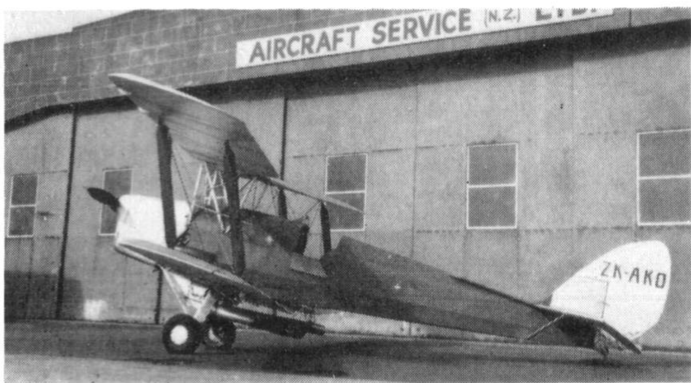
James Aviation's ZK-AKO, ex NZ1419, fitted for top dressing with large diameter phosphate ejection pipes.
