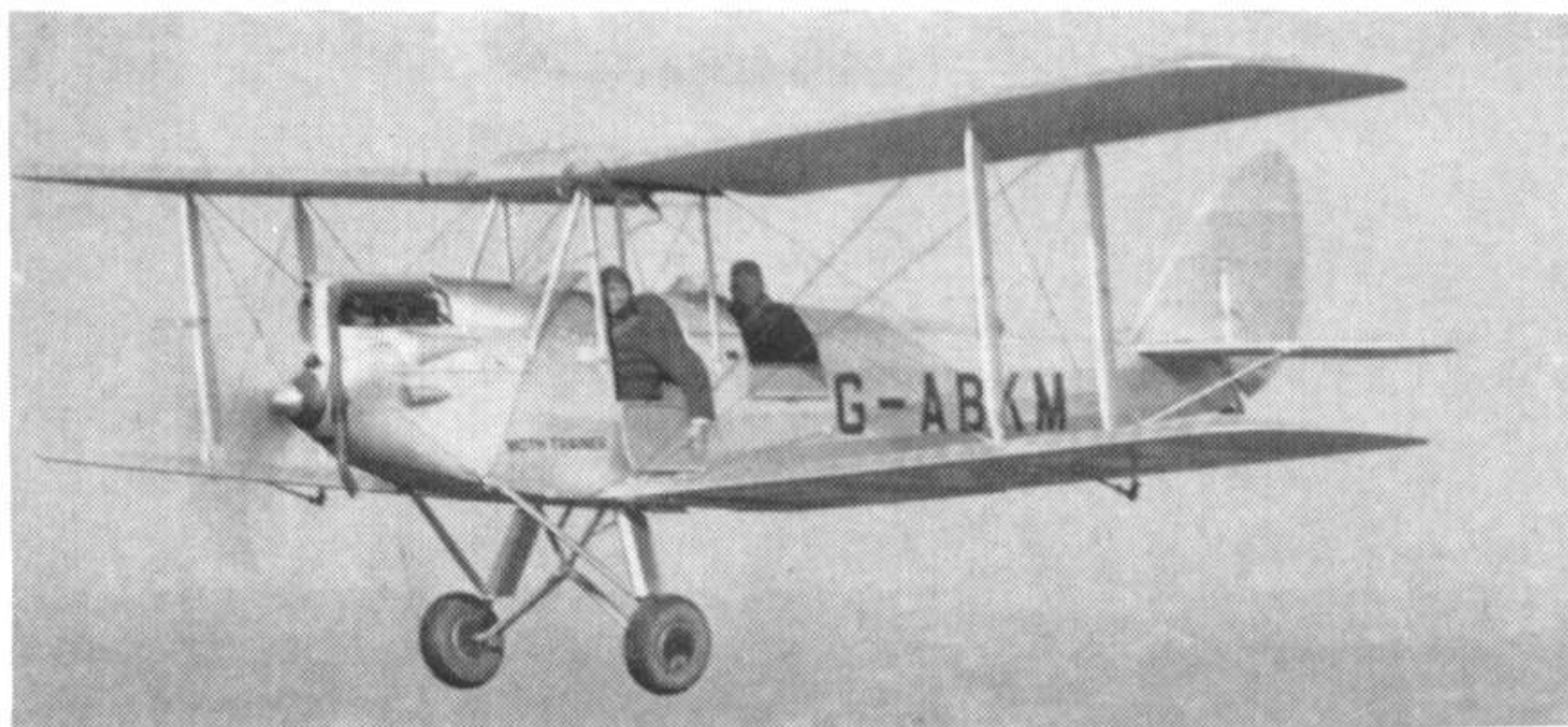
The second production D.H.60T Moth Trainer G-ABKM showing the large doors and repositioned flying wire anchorage.
