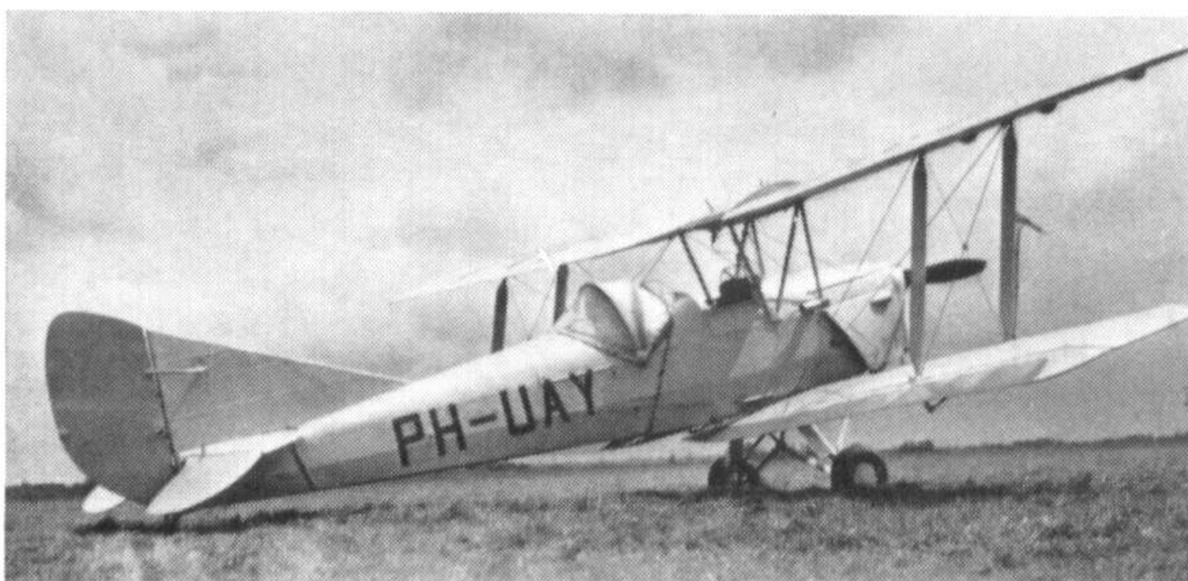
Tiger Moth PH-UAY of the Dutch National Flying School, Ypenberg with elongated fin and mass balanced rudder. Formerly G-ACDG, it flew with the D.H. School 1933 and Marshall's, Cambridge 1946-47.
