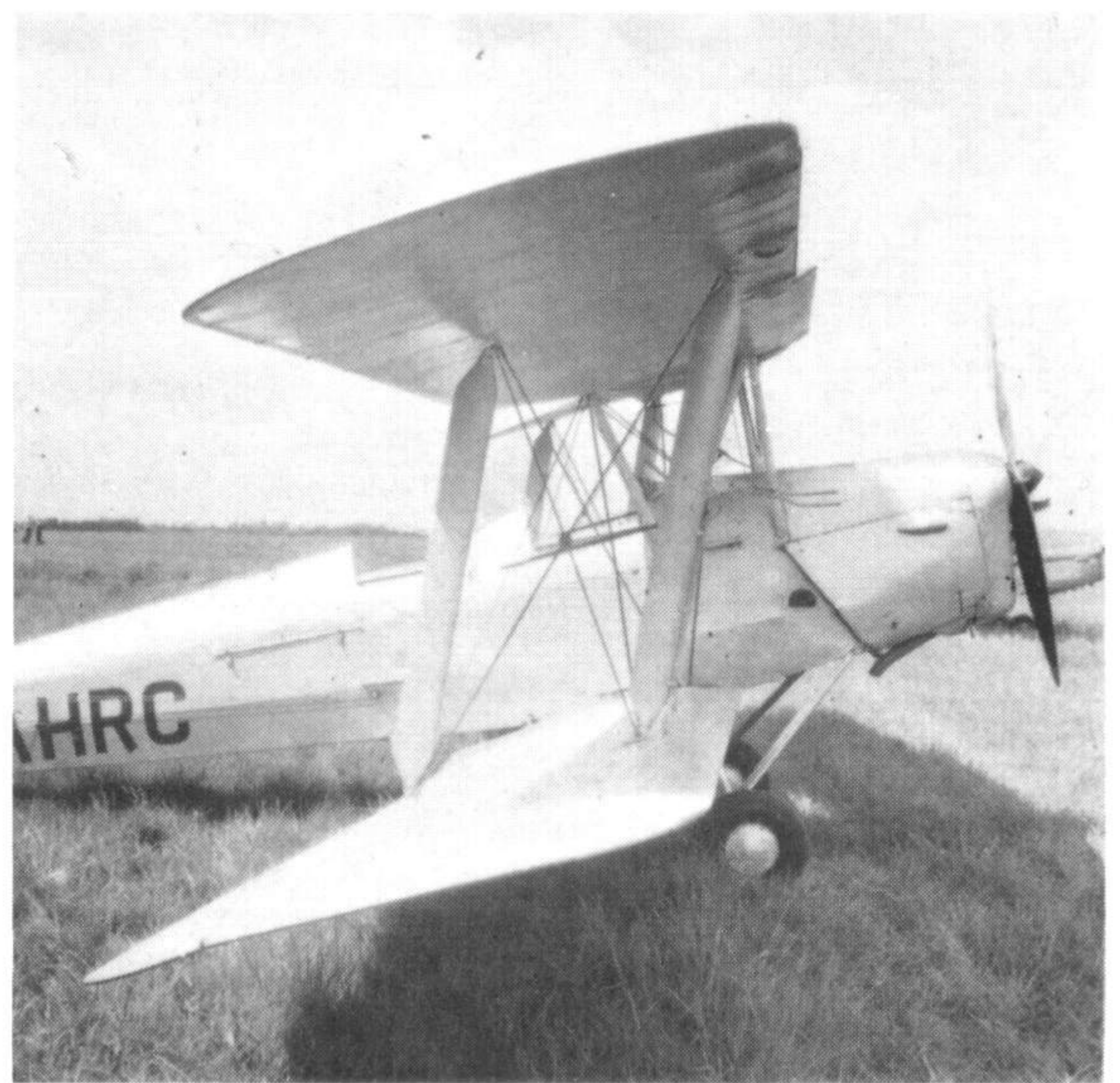
J. W. Tomkins' Tiger G-AHRC, ex T6064, with extended wing leading edges for inverted flying.
