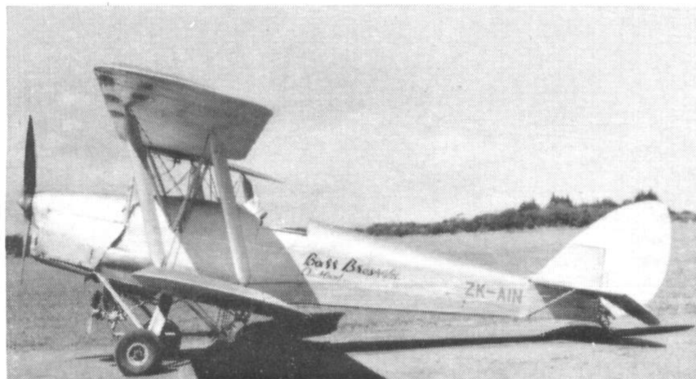
Left: Airfarm's VH-ADH, ex A17-680, operates with stripped rear fuselage. Right: Bain Bros.' ZK-AIN, ex NZ775, with wind driven pump and under-wing spray bar.
