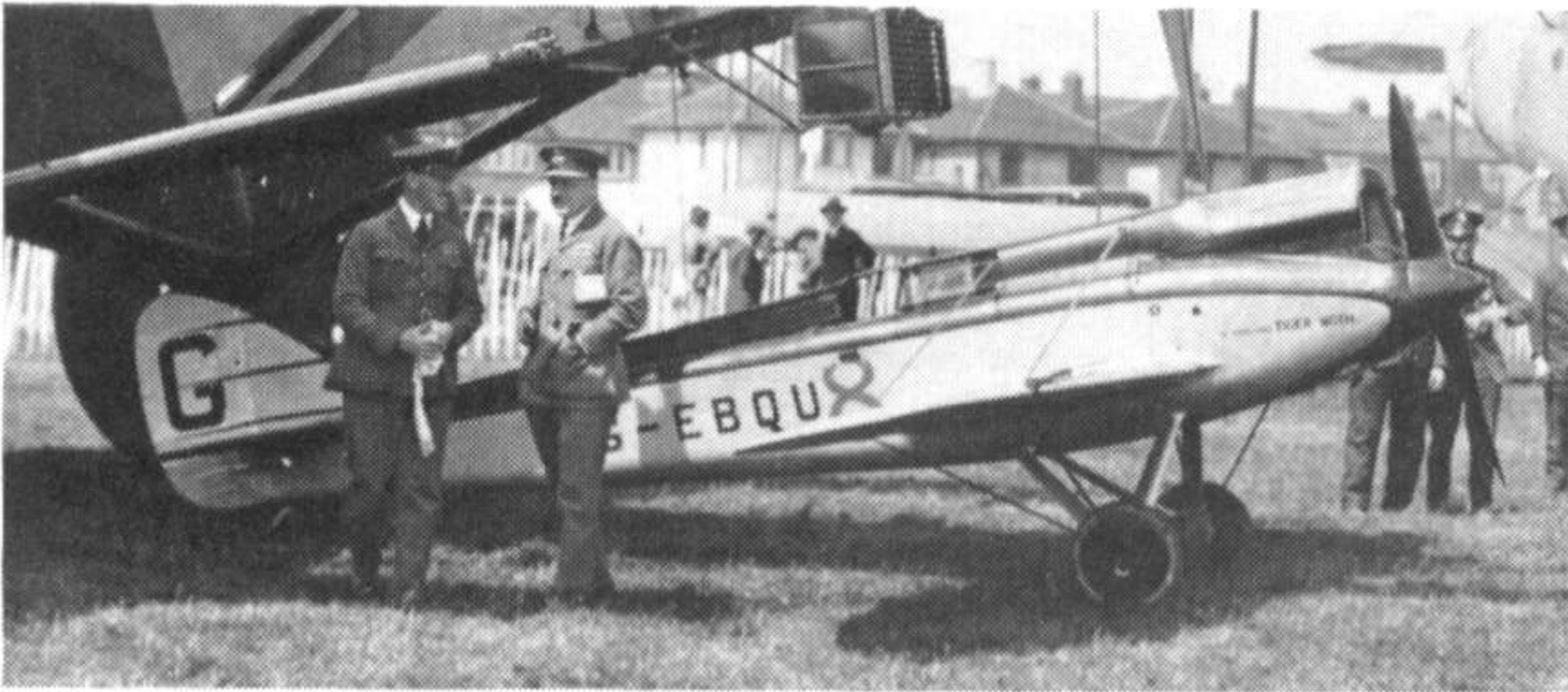
G-EBQU, first of the two D.H.71 Tiger Moths, with prototype Gipsy engine.
