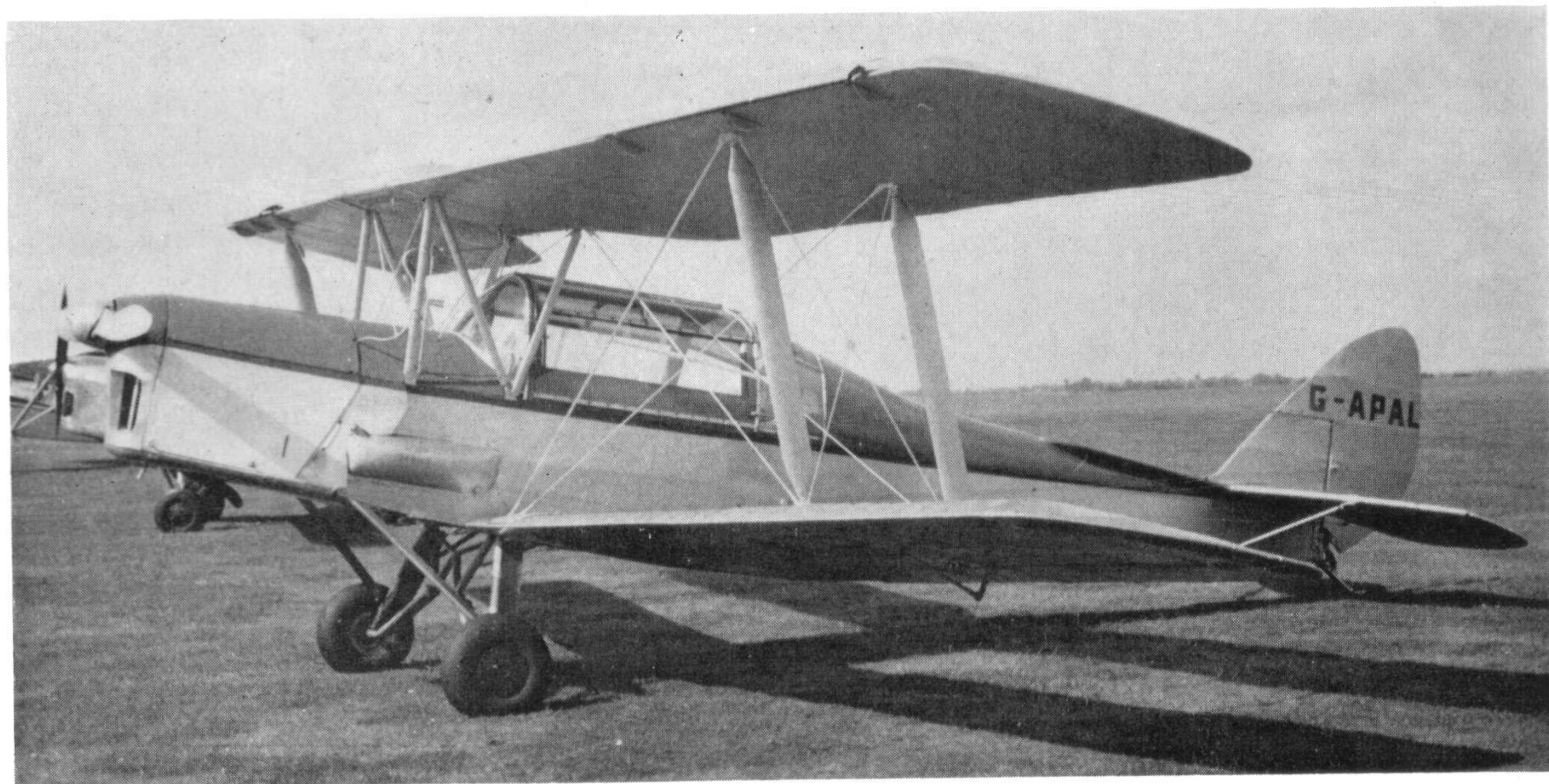
Jackaroo G-APAL, first flown in 1959, was a conversion of Tiger Moth N6847.
