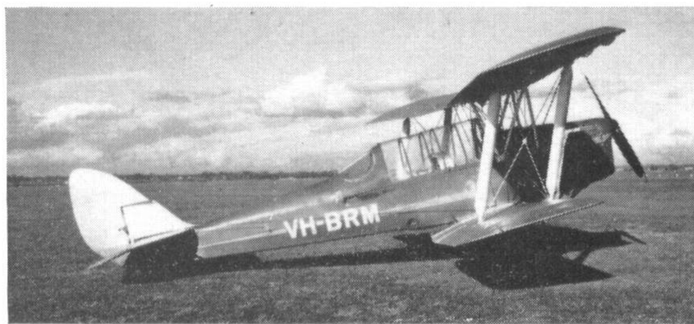
Australian-built Tiger Moth VH-BRM, ex A17-752, with the sliding canopy from a Commonwealth Wackett Trainer.
