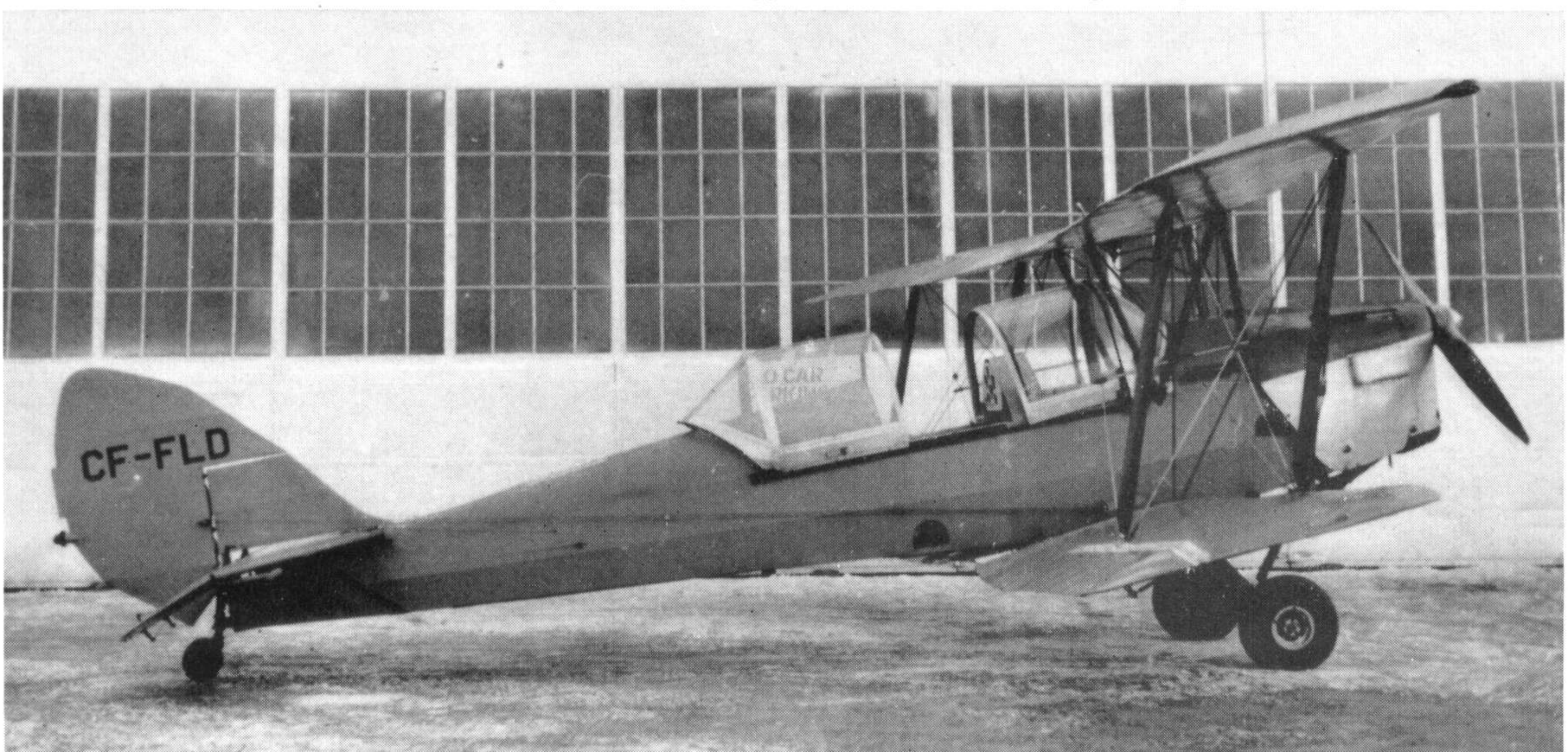
The Canadian built D.H.82C CF-FLD showing the sliding canopy and strut and undercarriage modifications.
