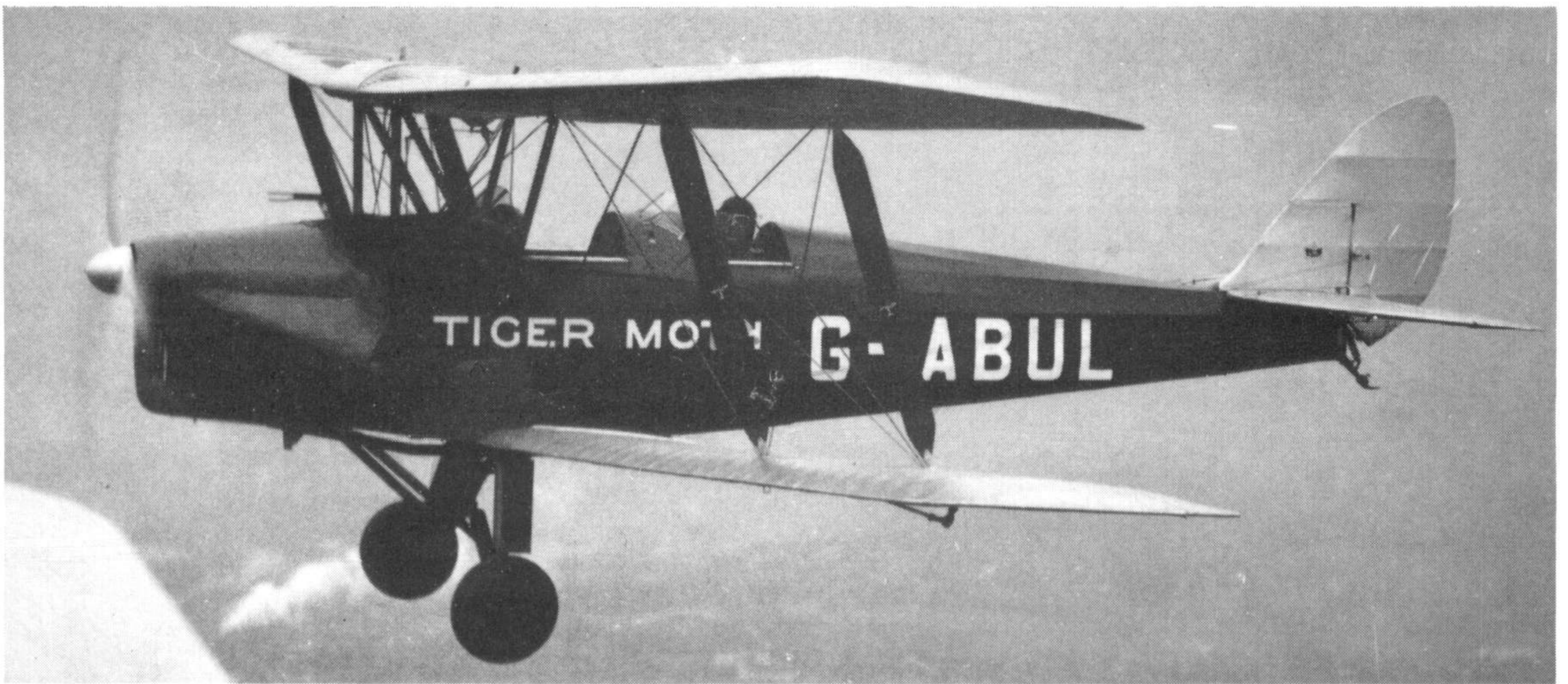
D.H.82 Tiger Moth G-ABUL, c/n 3107, of Cobham's Circus showing the fabric covered rear decking. (Photo: Charles E. Brown)
