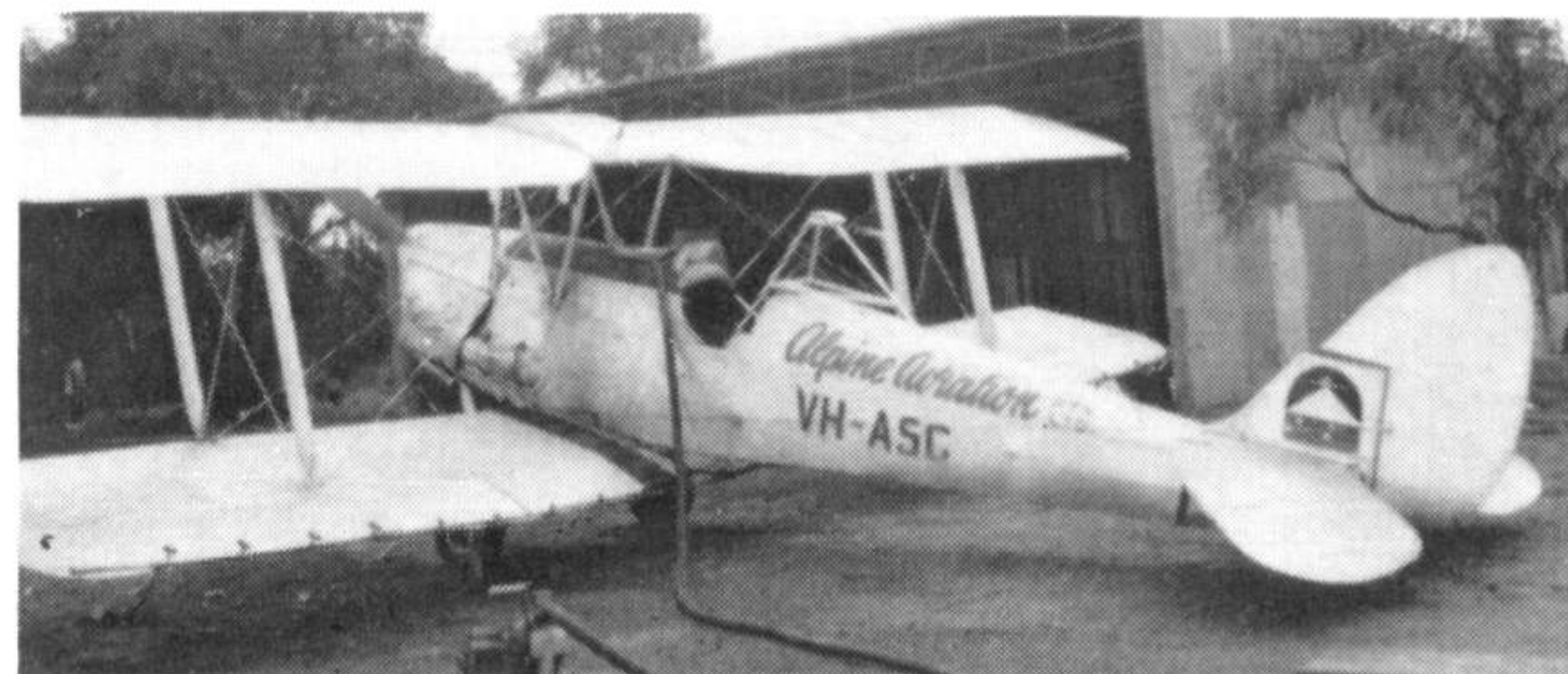
An Australian single seat crop sprayer VH-ASC, ex A17-397, of Alpine Aviation with tubular steel crash pylon and trailing edge jets. (Photo: John Hopton)
