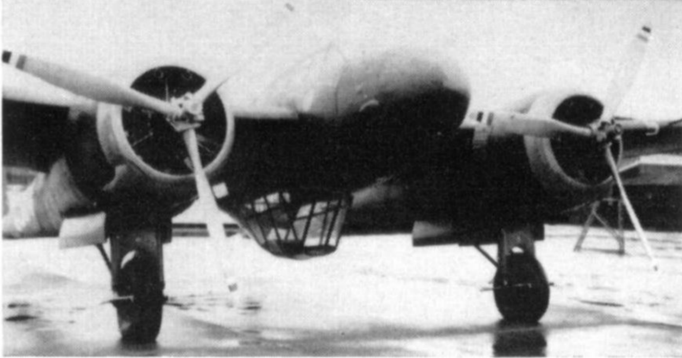
No. 304, the "bath-tub" G-1, with experimental observer's gondola; in practice it was found that the observer's position was too cramped for efficiency, and the project was dropped.
