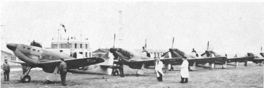
Fuselages of the first production batch at Toulouse-Saint Eloi in late November 1939; and machines of the initial batch awaiting delivery to the Armée de l'Air at Toulouse-Francazal in February 1940. It is just possible to distinguish the unfaired compressor intakes on the noses. (Photos: S.A.)
