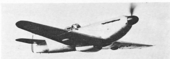
Top: The D.520-01 on its second flight, 8th October 1938; note underwing radiator. Centre: Note new fin and rudder in this view of D.520-01 over Toulouse in mid-November 1938; also the propeller spinner. Bottom: The second prototype in February 1939; note machine-gun "baths" under the wings.
