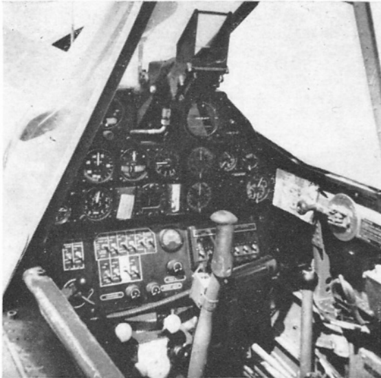
Cockpit and gunsight details of Desert Air Force Kittyhawks Mk. Ia; note operations log under cockpit, showing tally of nine bombing missions and three German aircraft shot down. (Photos via R. Ward)
