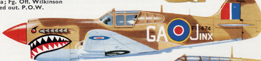
Kittyhawk Mk. IV, FX740, flown by Sg. Plt. G. F. Davis, No. 112 "Shark" Sqn.; Cutella San Angelo, Italy, May 1944. One 500 lb. bomb under fuselage, two 250 lb. bombs under wings. A/c. lost 31st May.
