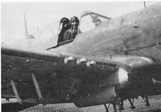
Powerplant and bomb-mounting details of a "Shark" Squadron Mk. III. (Photos: via R. Ward)
