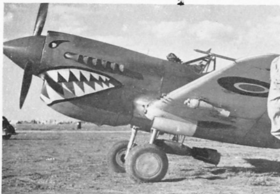
Kittyhawk Mk. III FR864 GA-M, flown from Pachino Agnone in August 1943 by Squadron Leader Illingworth. Note bomb load; two 250 lb. under fuselage and four 40 lb. anti-personnel under wings. (Photo: via R. Ward)
