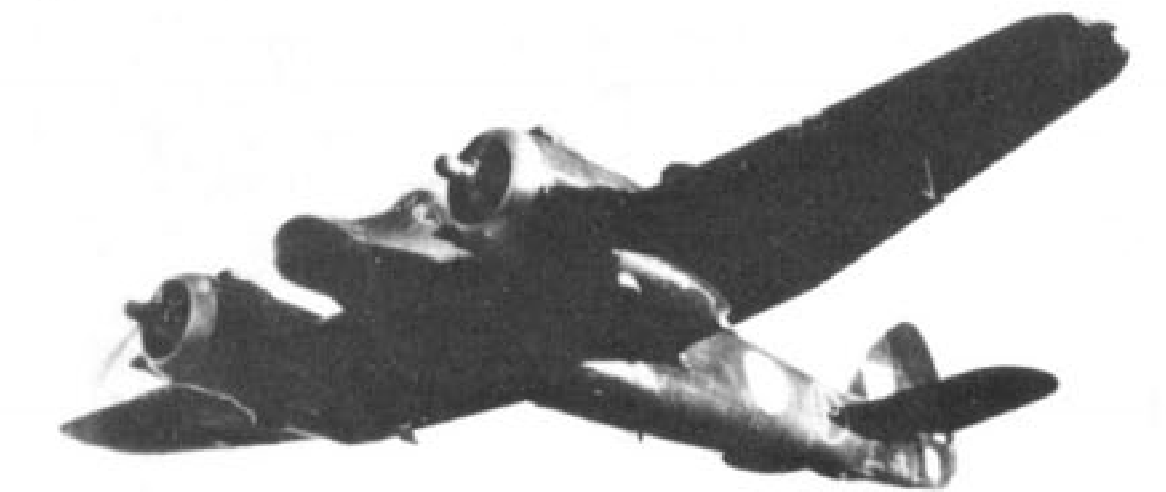
Immediately above: The second prototype Mk. II, R2061, seen here with R.R. "Exe"-type nacelles with extended tails. Below: X7579, a Beaufighter IF with A.I. Mk. VII centimetric radar.
