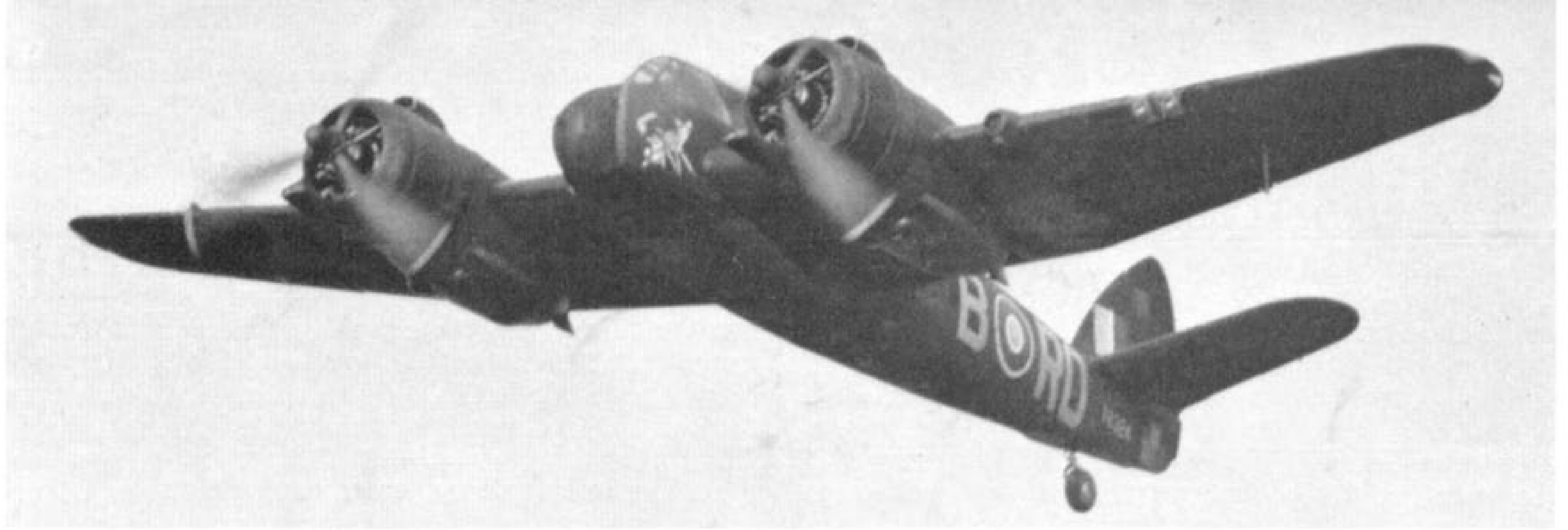
Mk. IF V8324 "RO-B" "Bambi" of No. 29 Squadron—subject of the five-view g.a. drawing on pp. 8 and 9. A.I. aerials were removed from original photo by wartime censor.
