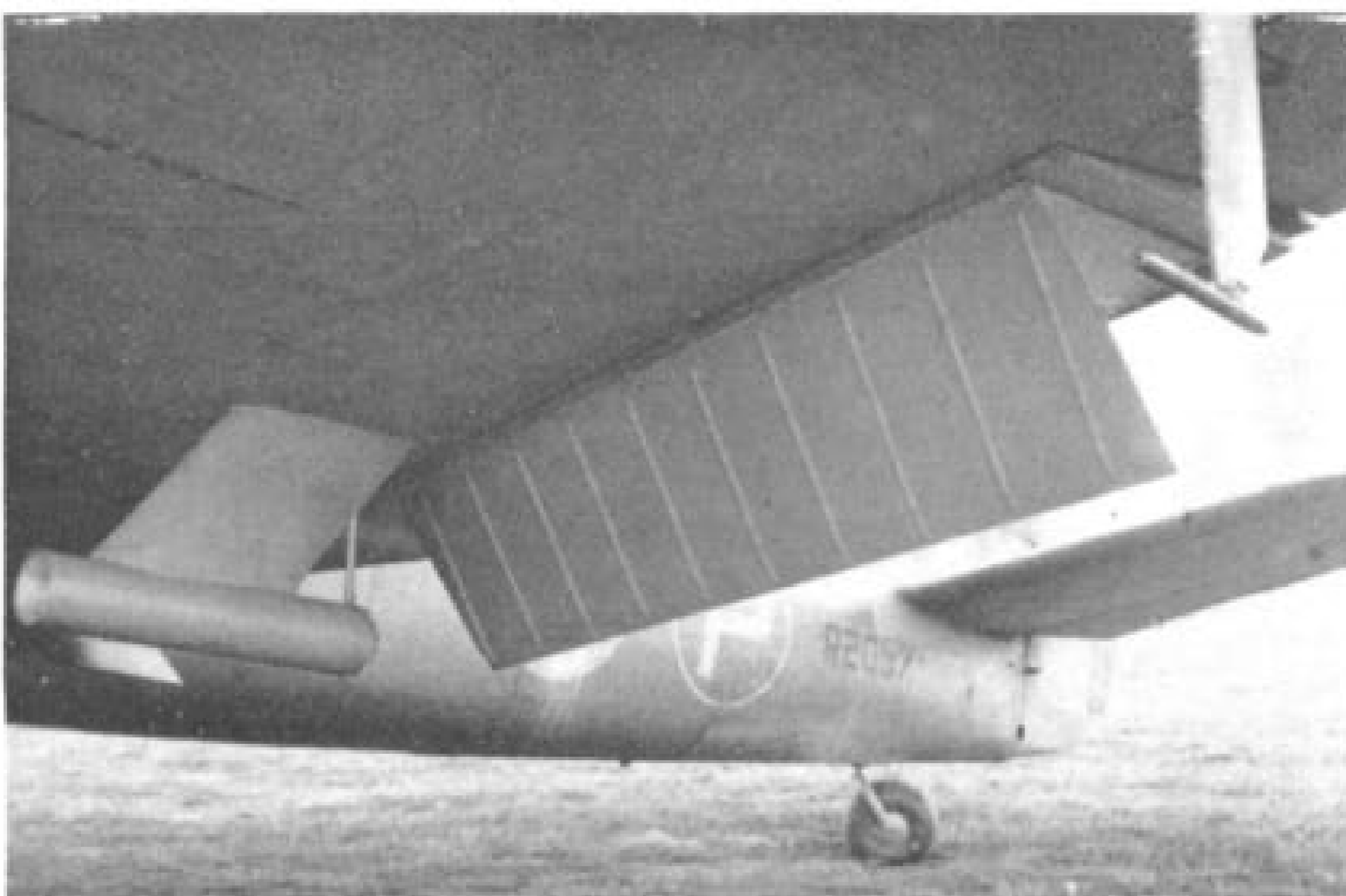
Above: Beaufighter IIF R2270 with dihedral tail plane. Below: T3032, a Mark II with dorsal-fin extension later adopted for the Mk. X.
