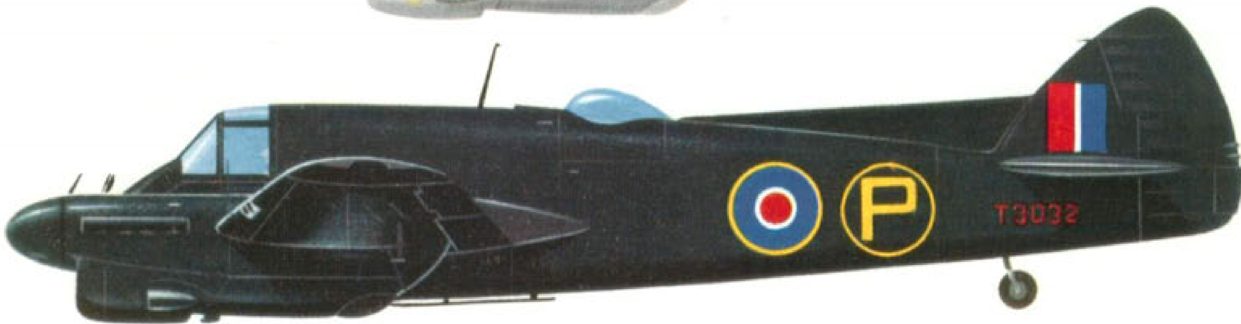
Beaufighter Mk. IIF, T3032, with an experimental dorsal fin.
