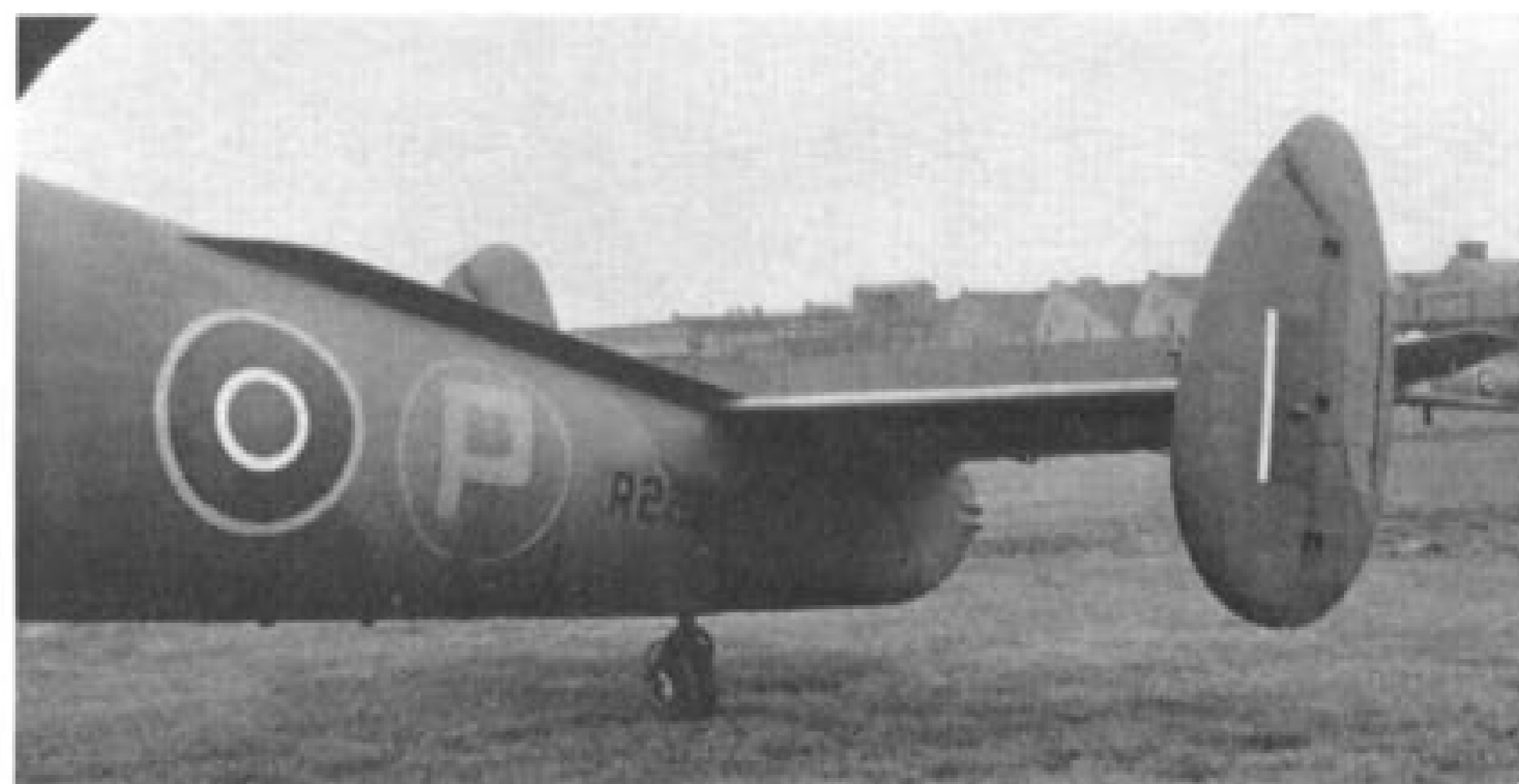
Mk. IF R2268 with wide tail plane and twin fins and rudders at Filton in 1940. Below: Same machine later, with strakes added.
