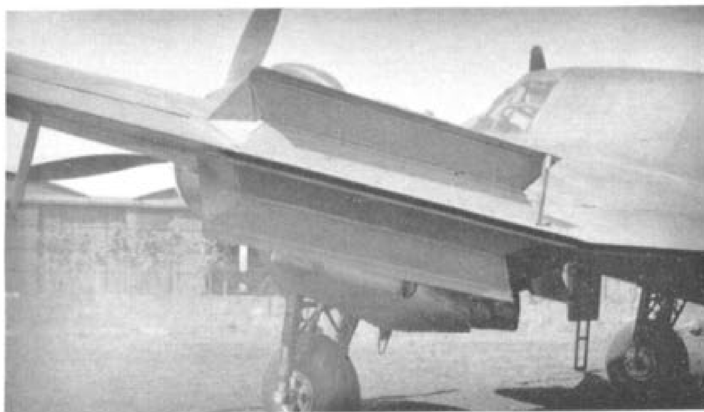
Two views of Mk. IF R2057 which had Fairey-Youngman bellows-type dive brakes and dihedral tail plane. The bellows were held shut by suction from the venturi below the wing.
