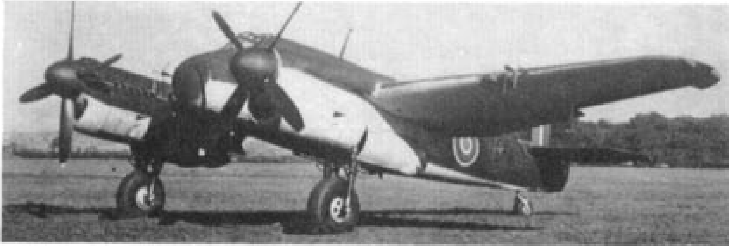
Above: Two views of T3177, a Mk. II allocated to Rolls-Royce as a Grifflon IIB test-bed.
