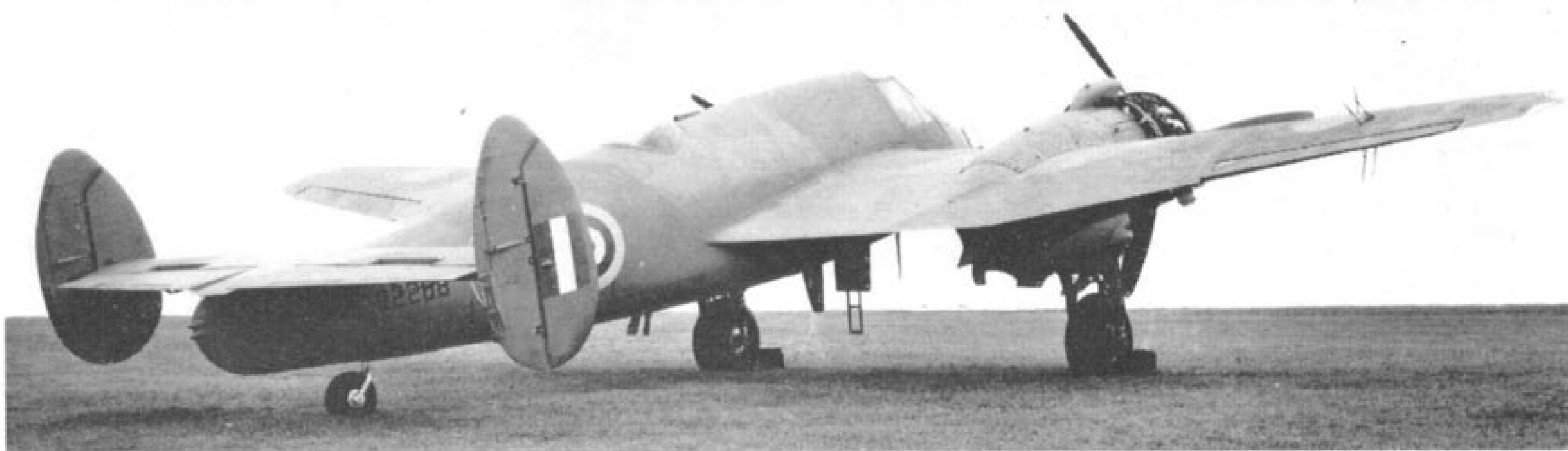
Mk. IF R2268 with wide tail plane and twin fins and rudders at Filton in 1940. Below: Same machine later, with strakes added.
