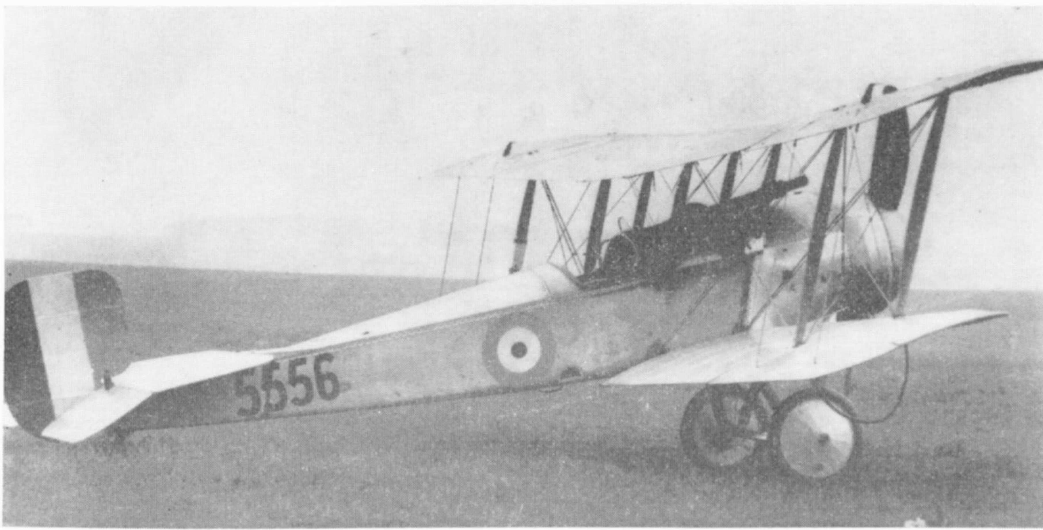
No. 5556 with basically similar installation but rather more refined engine cowling. Like No. 5555, this aircraft had the large rudder. (Photo: Ministry of Defence)
