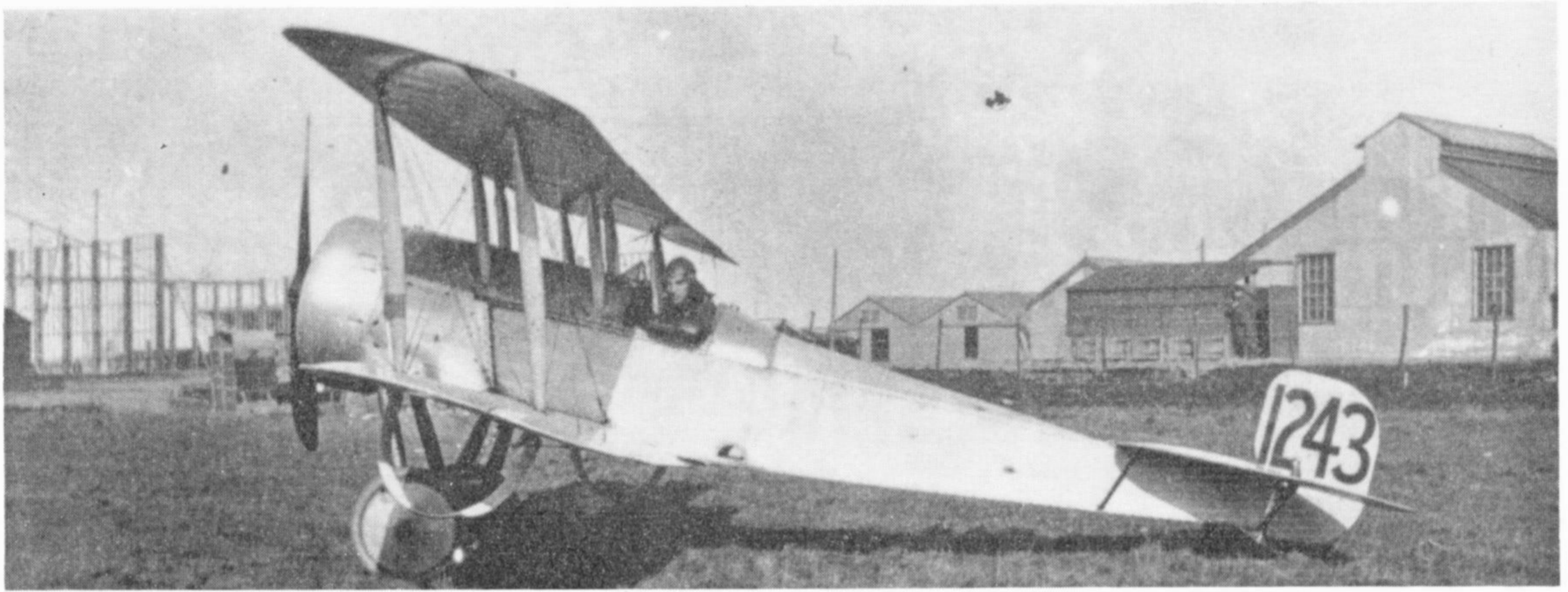
The first production Scout C, No. 1243, at the Isle of Grain. In the cockpit is Flight Sub-Lt. W. G. Moore. The fairings on the wing-tip skids are an unusual refinement.
