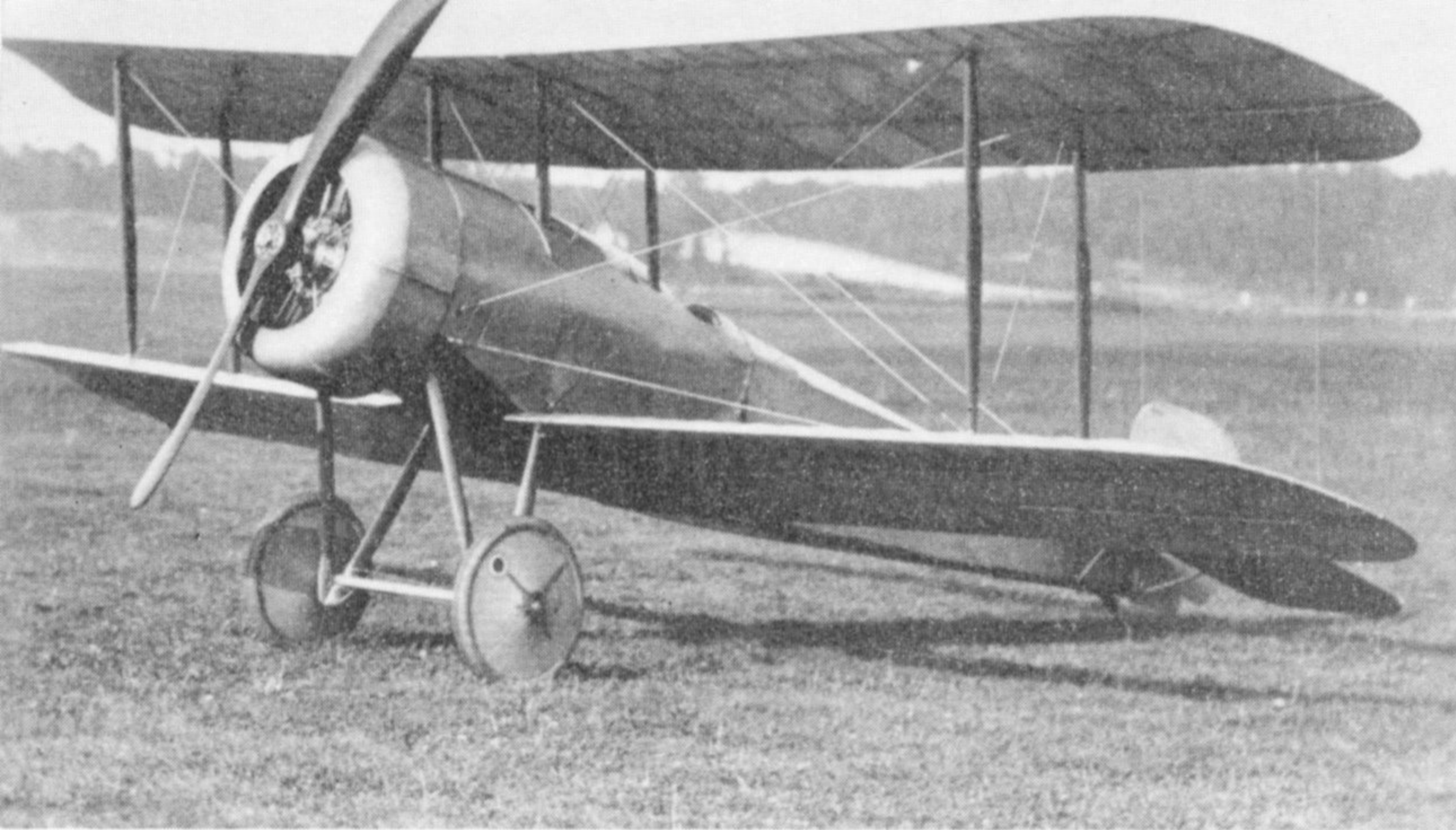
The modified Scout with new wings of greater span and chord and open-front engine cowling.
