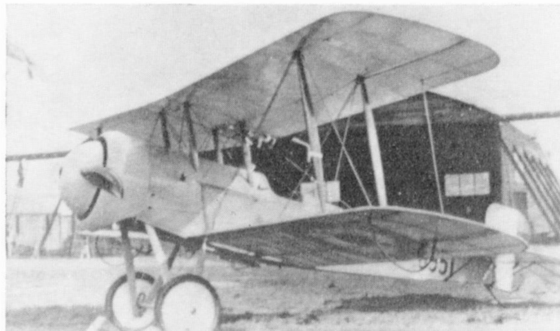
Scout D No. 8951 with spinner on 100 h.p. Monosoupape engine.
