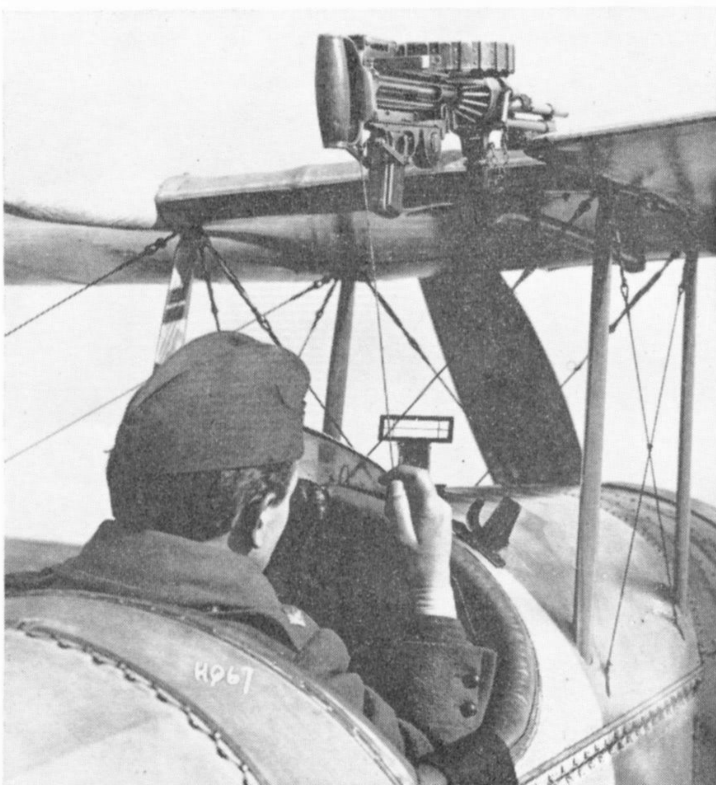
Overwing mounting of Lewis gun on R.F.C. Scout C. The gun was held in the level and vertical positions by spring clips, and the firing control was somewhat primitive. An unusual gun sight is fitted. (Photos: Crown copyright)
