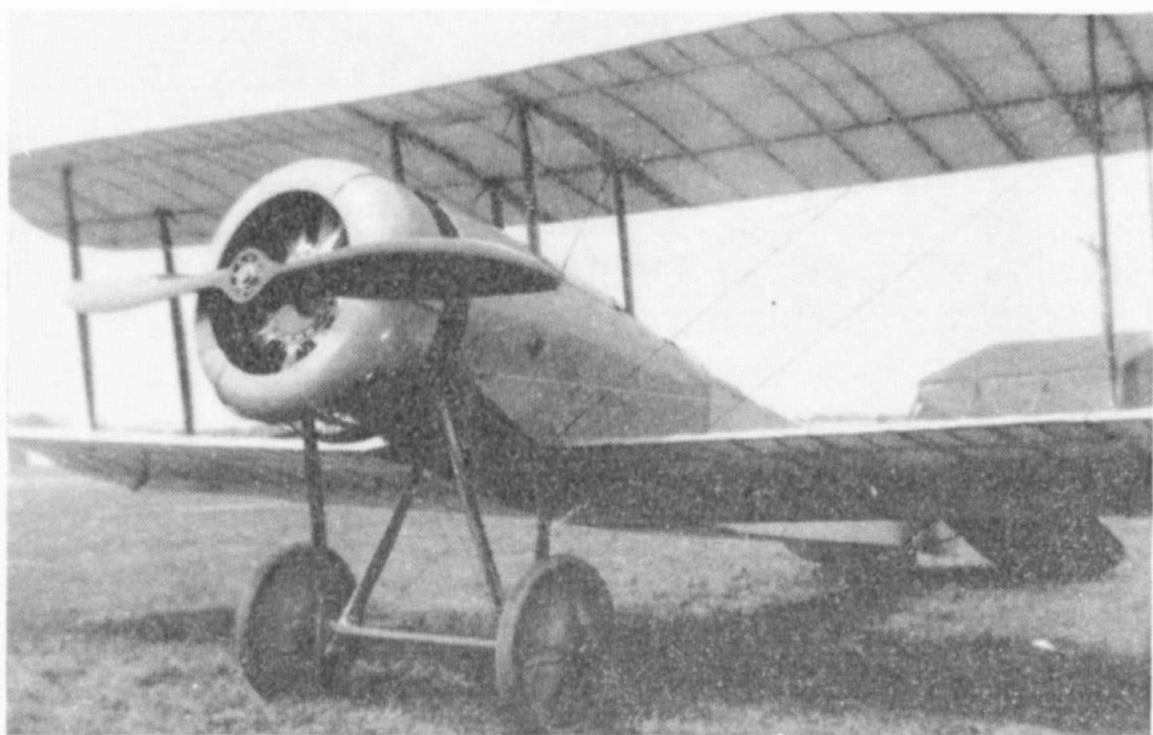
The first Scout after it had been bought by Lord Carbery and fitted with an 80 h.p. Le Rhône engine. With this engine the lower portion of the cowling was extensively cut away.
