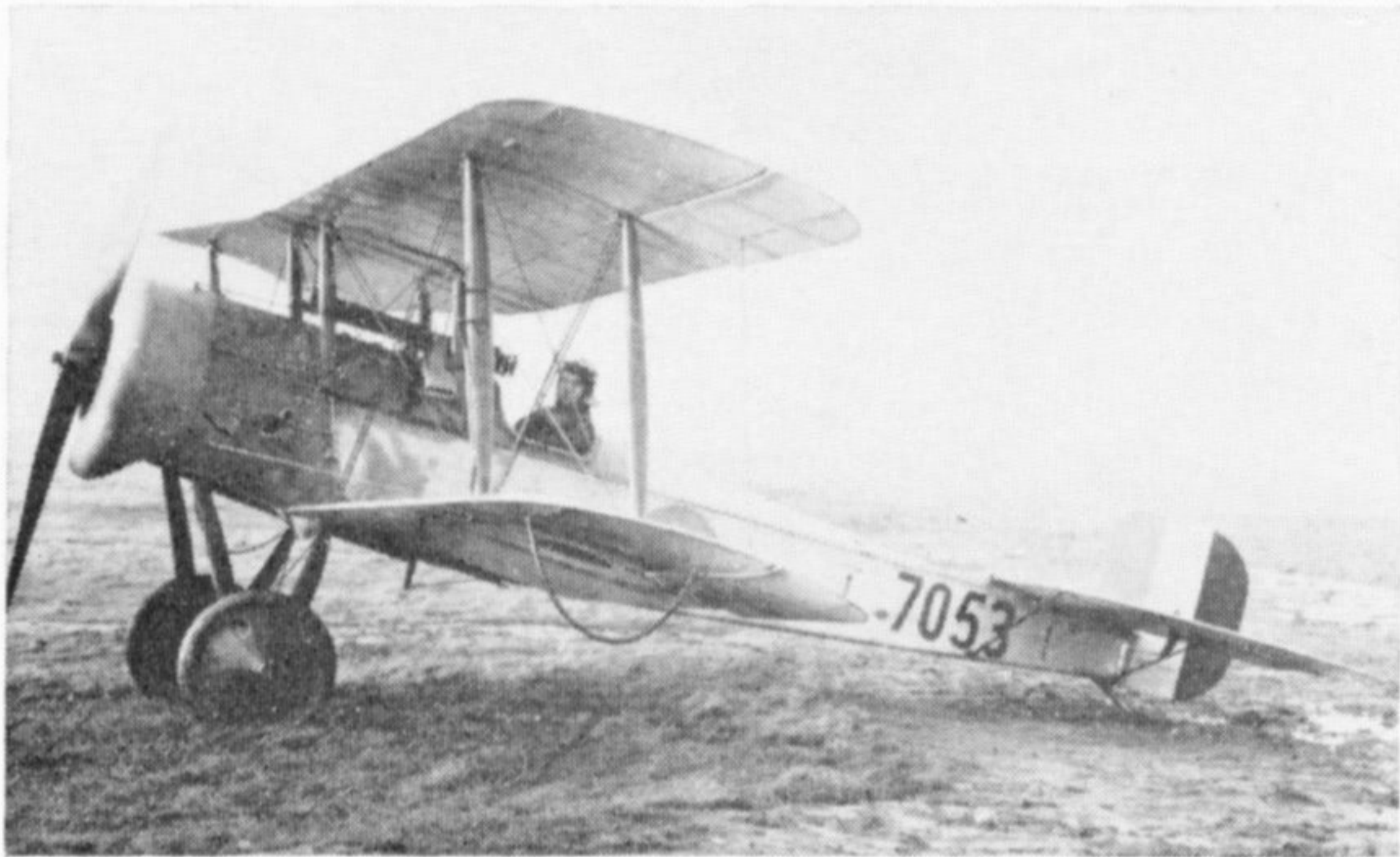
Scout D with synchronized Vickers gun. The installation of the armament differs slightly from that on No. 5314. The aircraft has the short ailerons and outboard wing-tip skids that typified the later Scouts D. (Photo: Aeromodeller)
