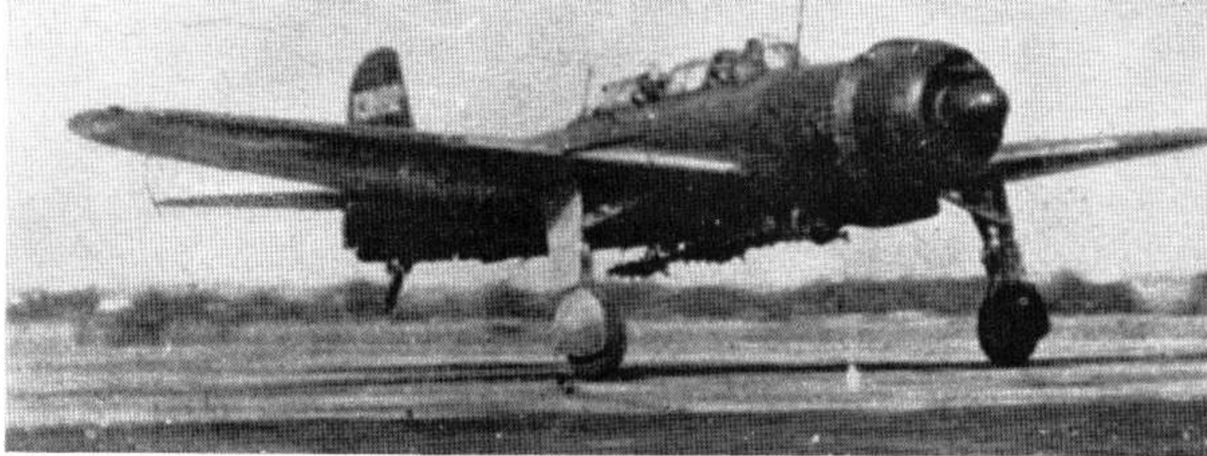
The Nakajima B6N1 Tenzan replaced the B5N2, first seeing combat in the Marianas in June 1944. Note bomb racks.
