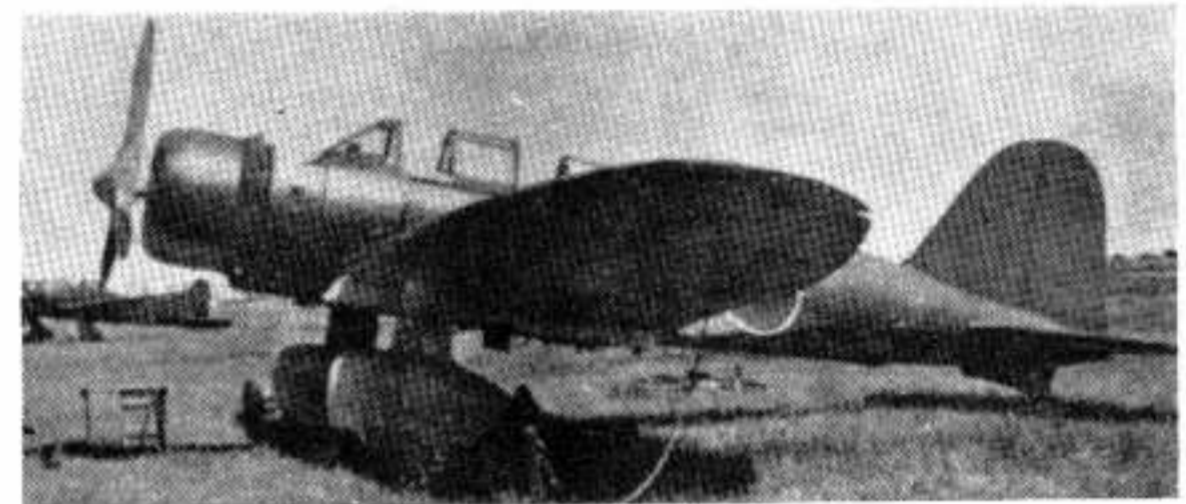
The common features of the B5M and the A5M "Claude" are apparent; a fixed spatted undercarriage and an elliptical wing.
