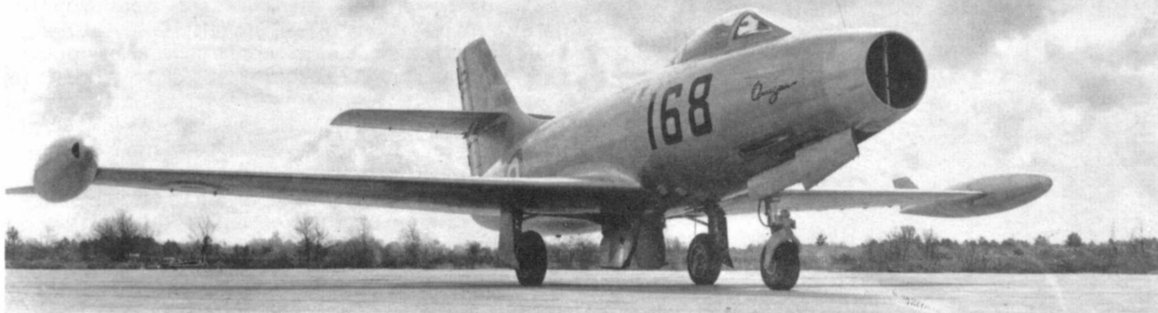
The 68th production Ouragan, displaying the new two-section nose wheel door introduced from the 51st aircraft onwards. (Photo: GAM Dassault)
