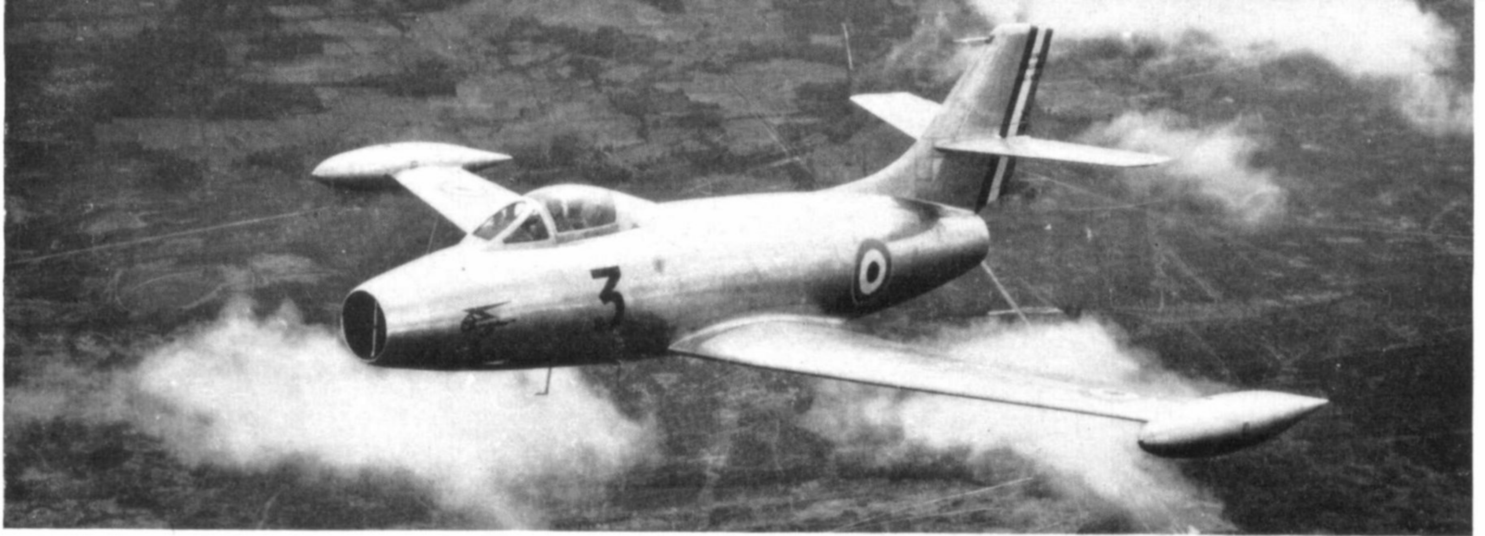
A fine aerial study of the third pre-series Ouragan: the tip-tanks still carry no fins. This aircraft was later the testbed for the HS403 afterburner developed for the Nene 104B. (Photo: Ministère des Armées "Air")
