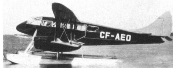
CF-AEO was converted to Fairchild 5500 floats and chassis by Canadian Fairchild at Longueuil, P.Q. and was flown to Rockcliffe (Ottawa) on 18th June 1935 for type approval tests by the R.C.A.F. Test flights were carried out by F/O C. W. Morrison of the Test and Development Flight, and the Rapide had a modified rudder, two cabin doors and an emergency exit for the pilot. With its sale to Canadian Airways in July 1935 the undercarriage reverted back to wheels and the Rapide was fitted with cameras for survey work.
