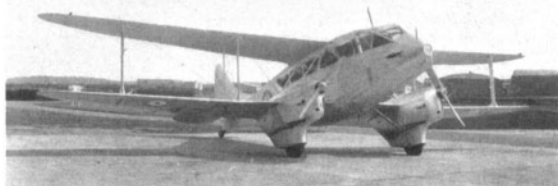
The military D.H.89, K4772, at Martlesham Heath on 26th April, 1935. Note extended dorsal fin, a Vickers Mk. V machine-gun and landing light in nose, five cabin windows (each side), navigation lights on wings and rudder, wooden propellers, and a deepened fuselage to house 4 x 20 lb. and 2 x 120 lb. G.P. bombs. Military Rapides were also sold to Spain, Iran and Lithuania.
