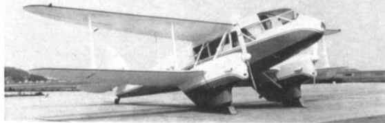
Owned by Avions Fairey S.A., OO-AFG (ex G-AKNC) was stripped down and completely rebuilt in 1958. Modifications included the installation of an electrical actuator (with indicator) for flap operation, 44 channels VHF radio, radio compass, a blue moulded perspex canopy over the pilot's cockpit and enlarged cabin windows. An extra folding door was fitted to allow the carriage of bulky cargo. The exterior was finished in red and white. (Photo: Avions Fairey S.A.)
