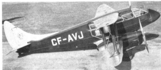
CF-AVJ, in full Canadian Airways livery and insignia, showing the additional starboard cabin door, was fitted with wheels for the Vancouver to Seattle service. This Rapide was destroyed by fire at Saint John, N.B. when the port engine exhaust started a fire during run up on 17th May 1939. (Photo: Canadian Airways)
