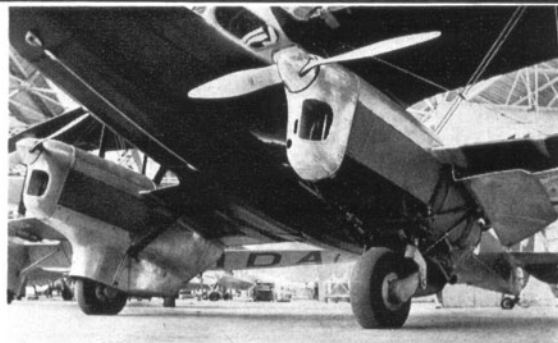
The Rapide E9, c/n 6420, experimentally fitted with a Dowty levered suspension undercarriage in 1938. (D.H. Photo)
