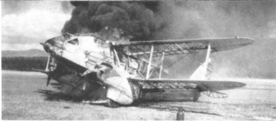
The sad sight of N.Z.N.A.C.'s ZK-ALC Tiora on fire at Rotaruia airfield when exhaust flames from the starboard engine set the grass alight and subsequently itself. The burnt away fabric reveals the spars and girder wing structure. There were no human casualties. (Photo: N.Z. Herald)
