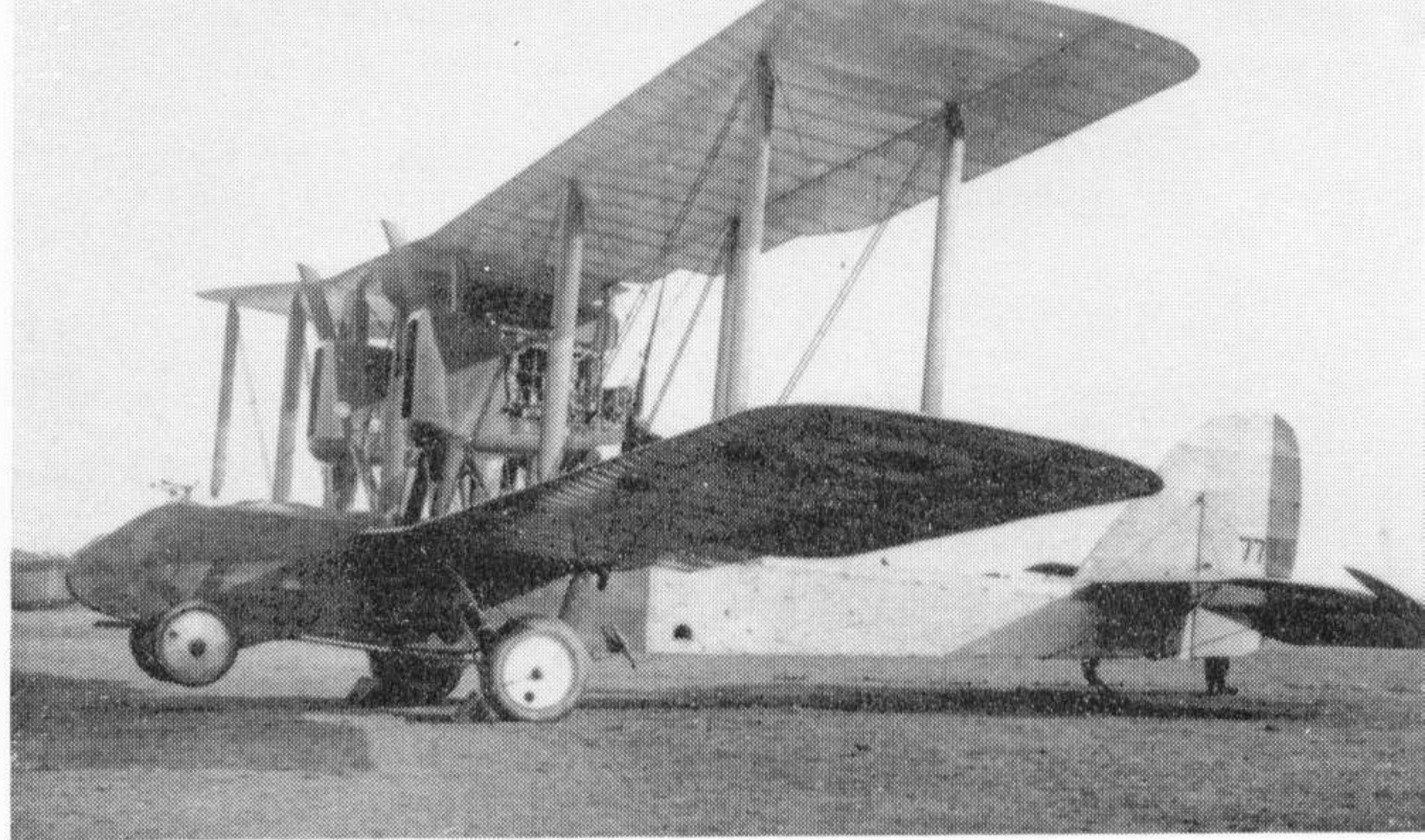
The basic configuration of the D.H.10 was first expressed in the D.H.3 of 1916. This photograph illustrates the D.H.3A with two 160-h.p. Beardmore engines. (Photo: I.W.M. Q67535)
