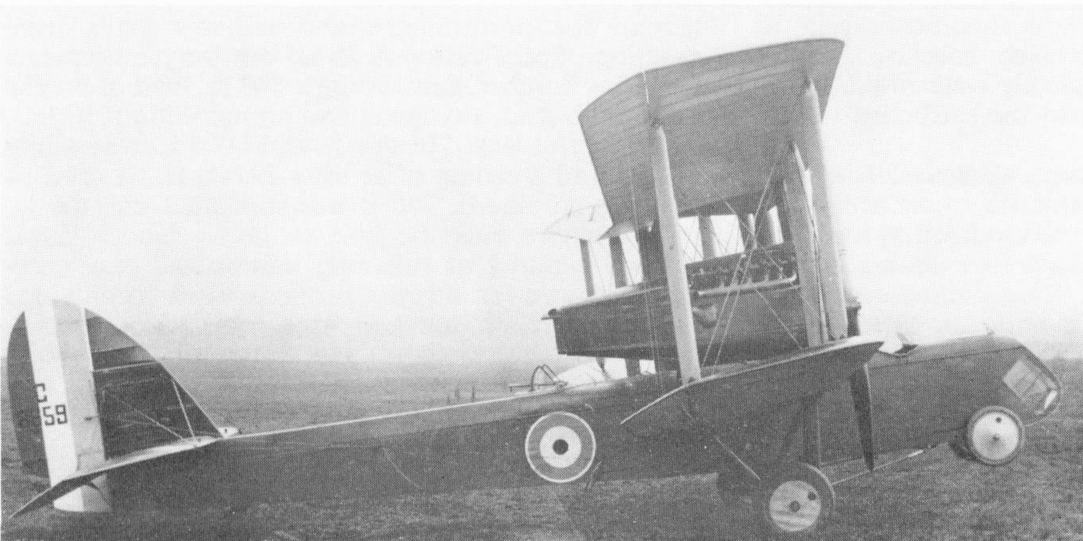
Left and above: The second prototype, C8659, with two Rolls-Royce Eagle tractor engines and transparent panels in the nose.
