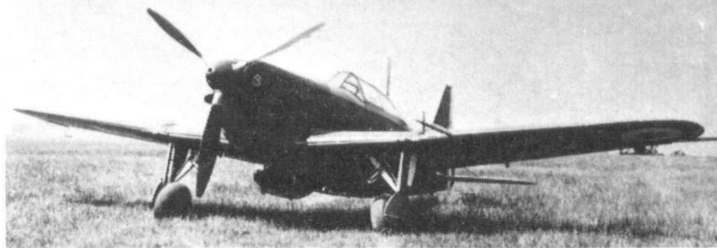
M.S. 406 No. 4, the fourth pre-production aircraft and the true prototype of the M.S. 406 series. (Photo: E.C.A.)
