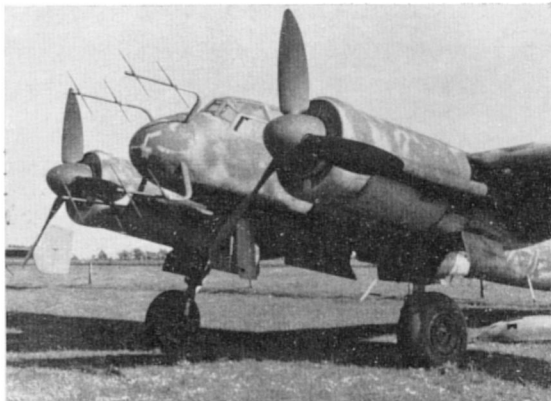
A Ju 88G-7a; note engine and camouflage details.
