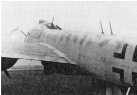
Two 20 mm. MG 151 cannon in a Shräge Musik installation pointed obliquely upwards from the fuselage; a single 15 mm. MG 131 in the rear of the cockpit provided a token rear defence. Note the code of NJG 102, "7J" in small characters ahead of the outline cross.
