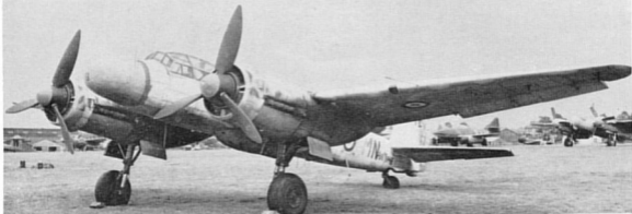
The final variant of the Ju 88 night fighter series, the G-7c. Ten examples were built before the German collapse; this aircraft carried the centimetric wavelength FuG 240 Berlin N-1a radar. (Photo: Imp. War Mus. MH4884)
