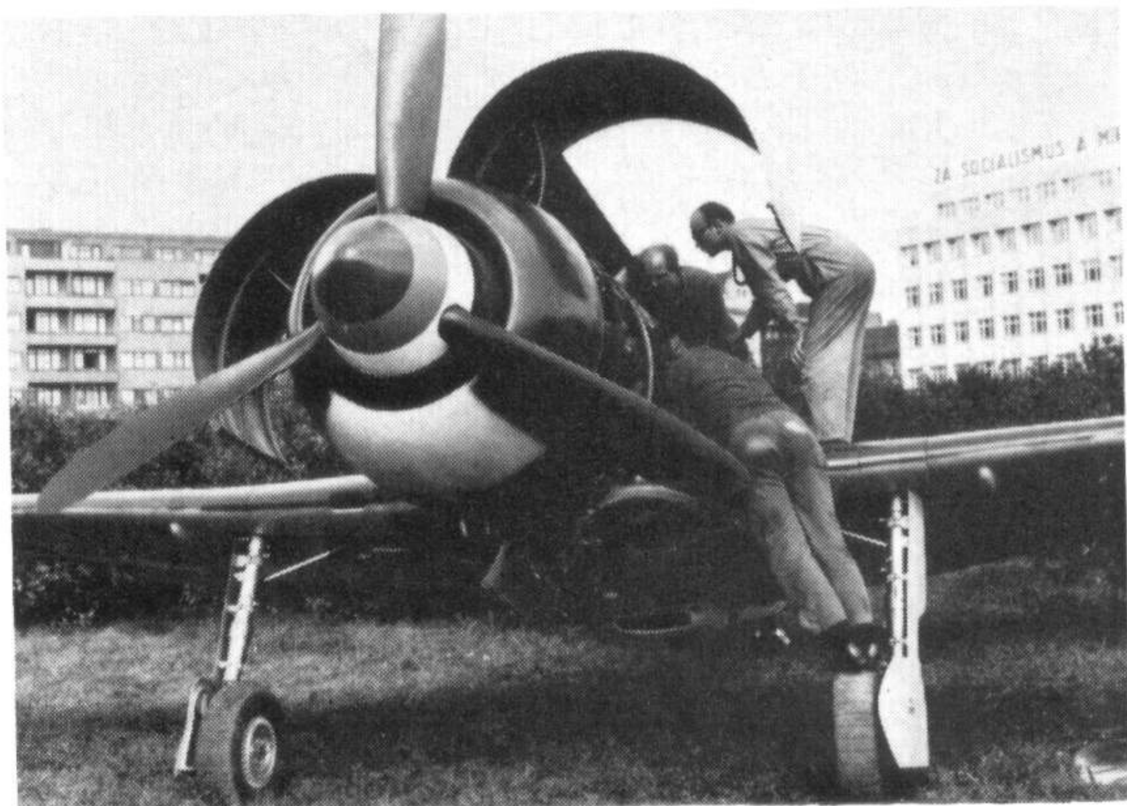
An La 7 is now preserved at the Prague Technical Museum in Czechoslovakia; these photographs give good views of the engine, undercarriage, and cannon magazines. Note also the simplicity and smoothness of the general finish. (Photos: Josef Krybus)
