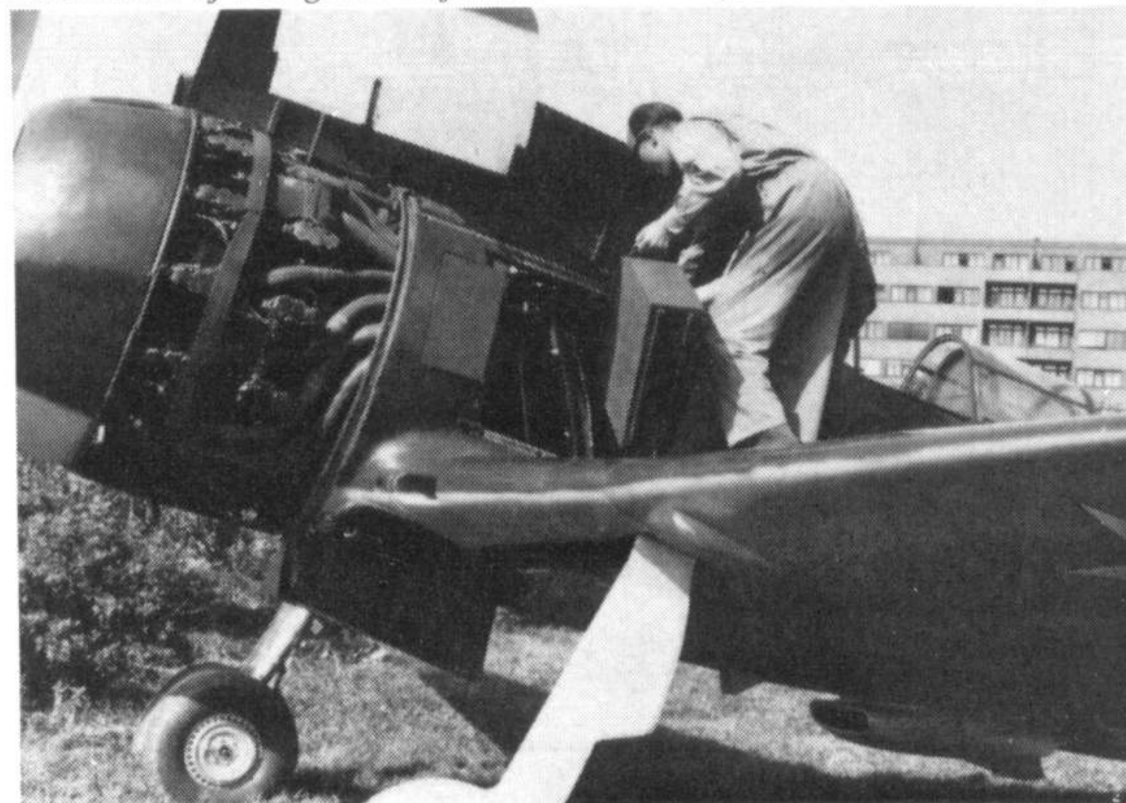
An La 7 is now preserved at the Prague Technical Museum in Czechoslovakia; these photographs give good views of the engine, undercarriage, and cannon magazines. Note also the simplicity and smoothness of the general finish. (Photos: Josef Krybus)
