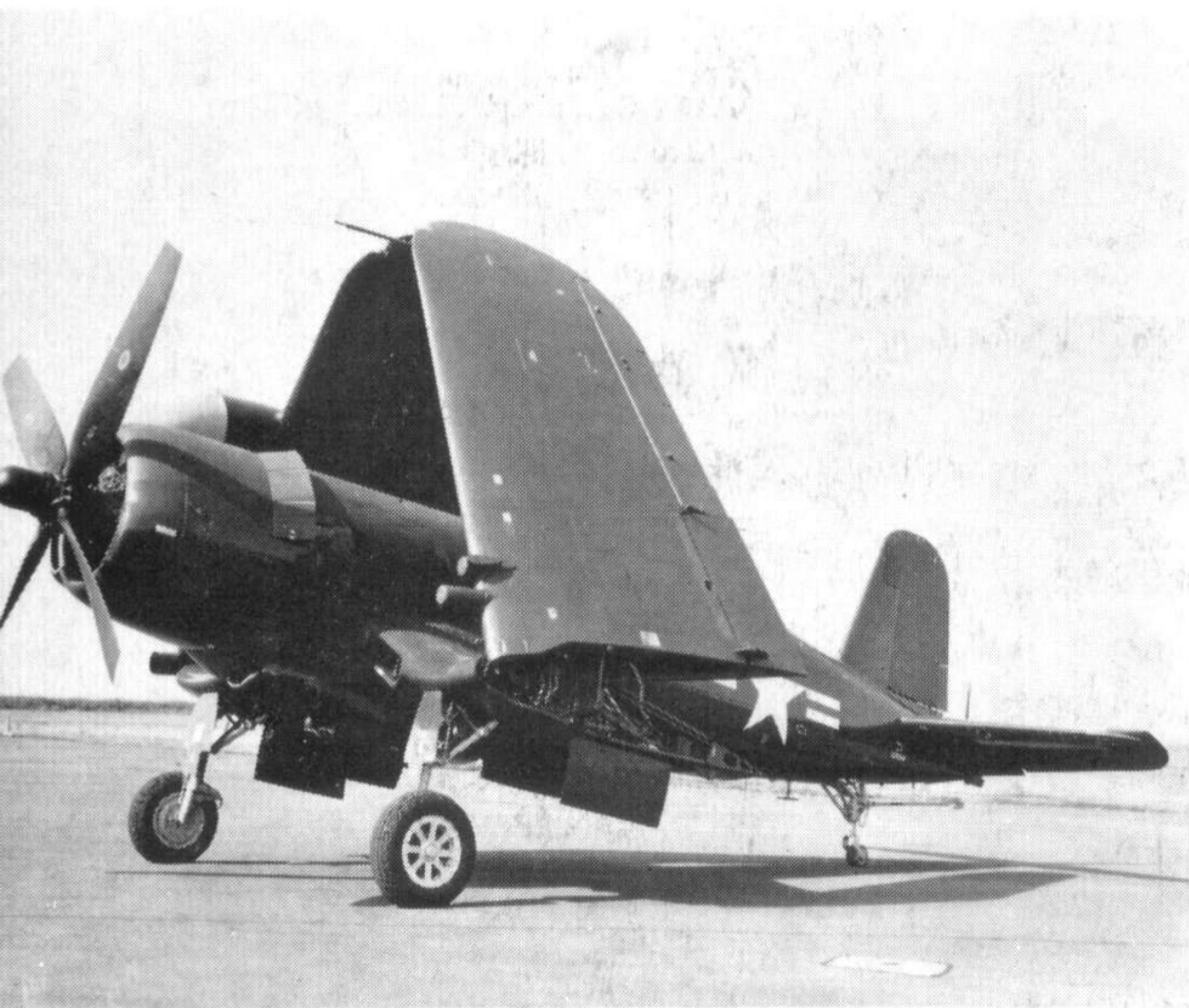
F4U-5N with wings folded; the small "bucket" on the starboard leading edge close to the fold line protects the gun camera from muzzle flashes during night combat.
