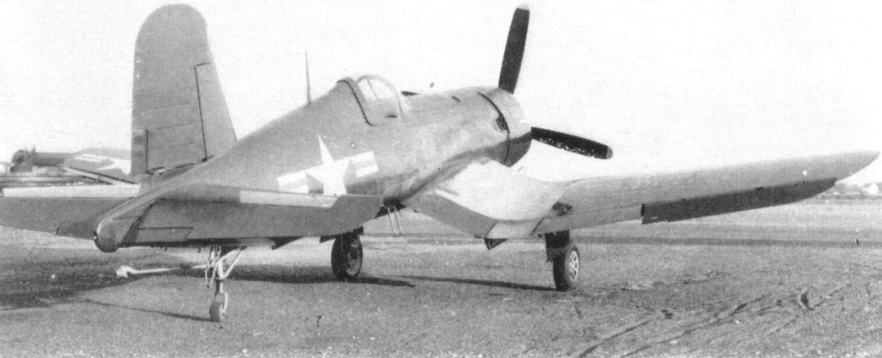
Note widened cowling for cheek inlets of this F4U-5, also fairing aft of canopy permitting higher seat positions. The canopy bulged beyond the edges of the sliding frame to improve rearward vision.
