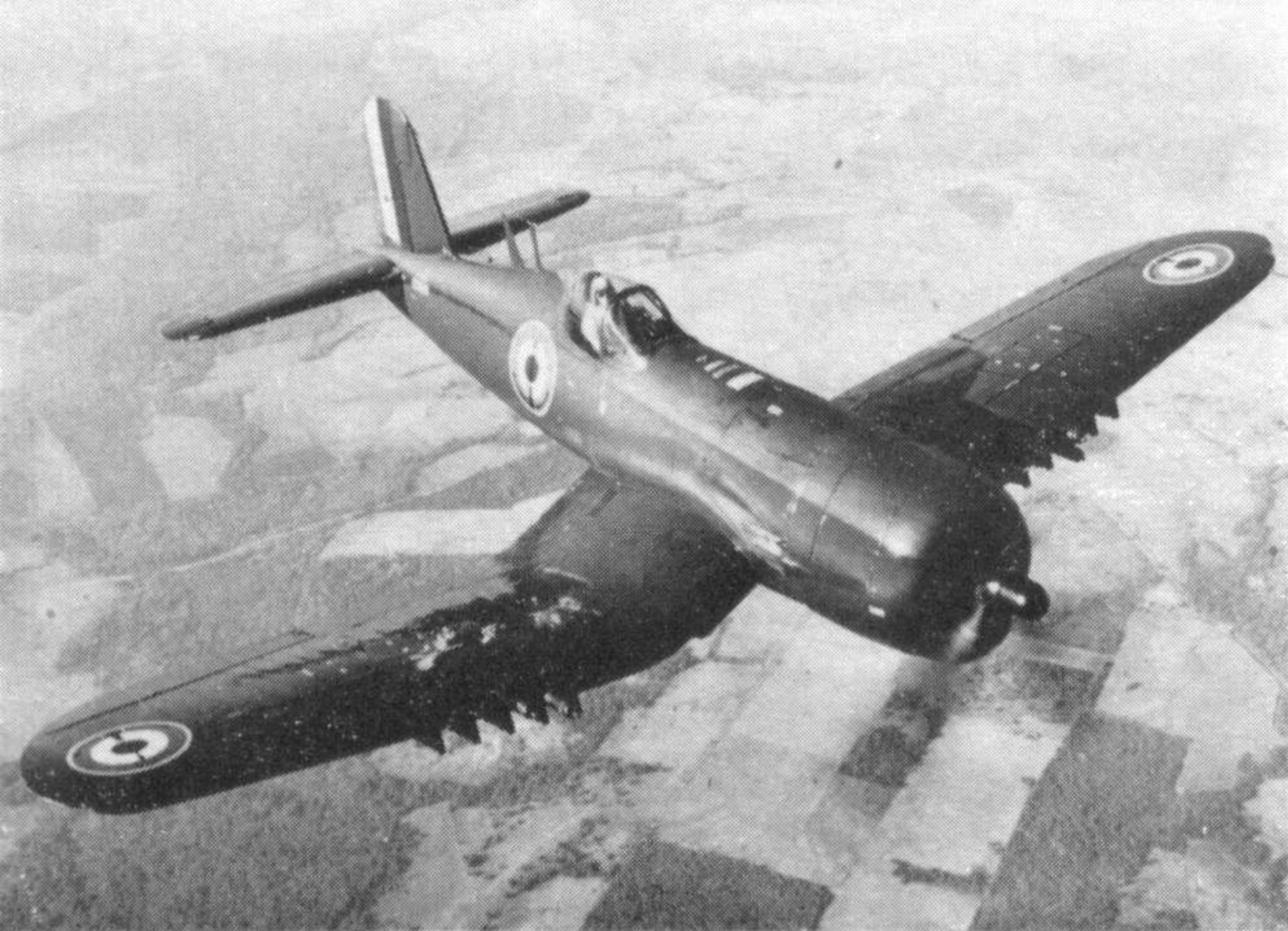
F4U-7 for the French Aéronavale during a flight test in the U.S.A. The fuselage lines of the F4U-5 were retained: in common with the -5 and AU-1 there was a widening ahead of Station 91 \frac{3}{4} .
