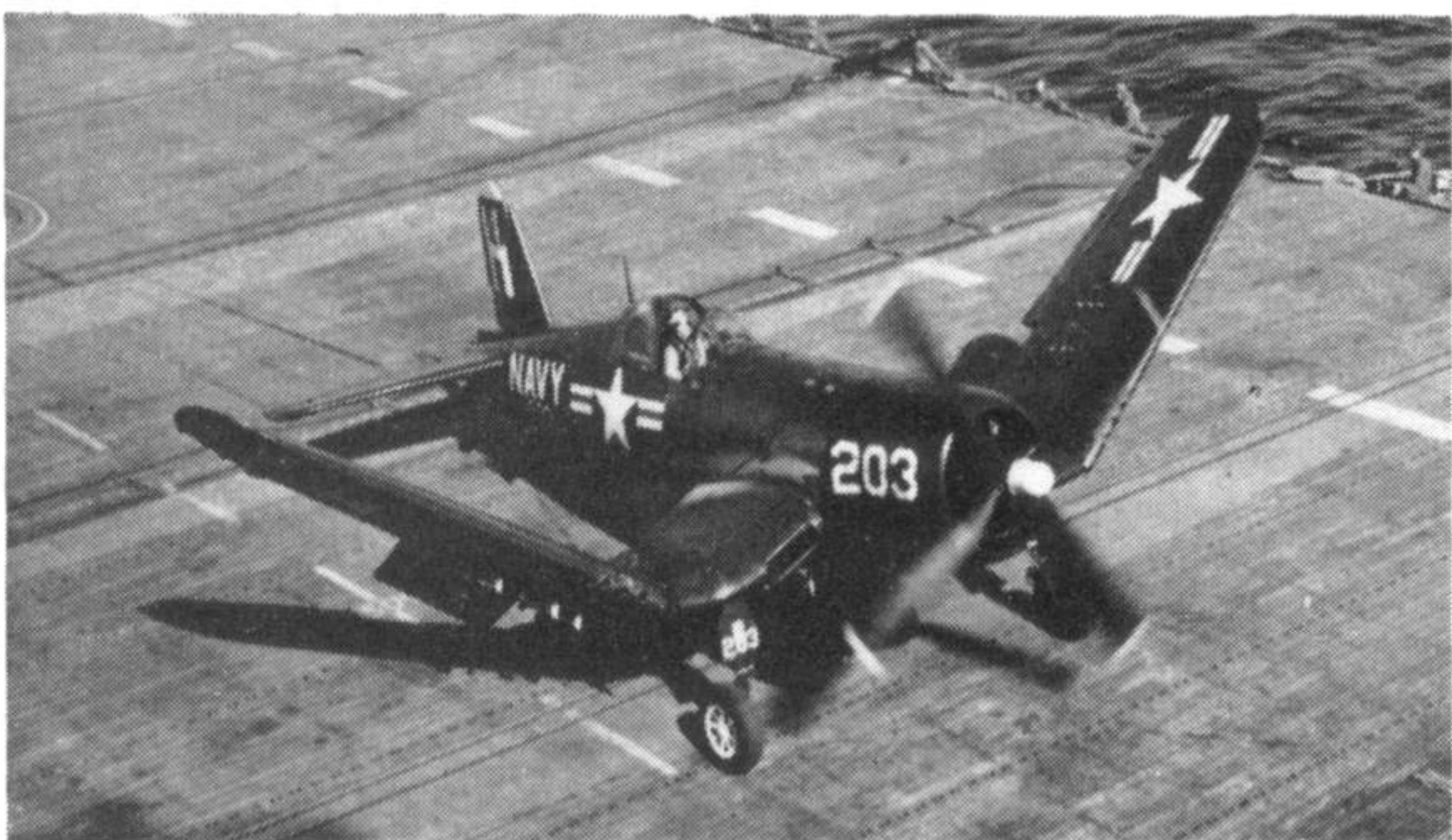
An F4U-4 of U.S. Navy Fighter Squadron VF 713 folds its wings to park on the flight deck of the carrier U.S.S. Antietam, cruising in Korean waters in March 1952.
