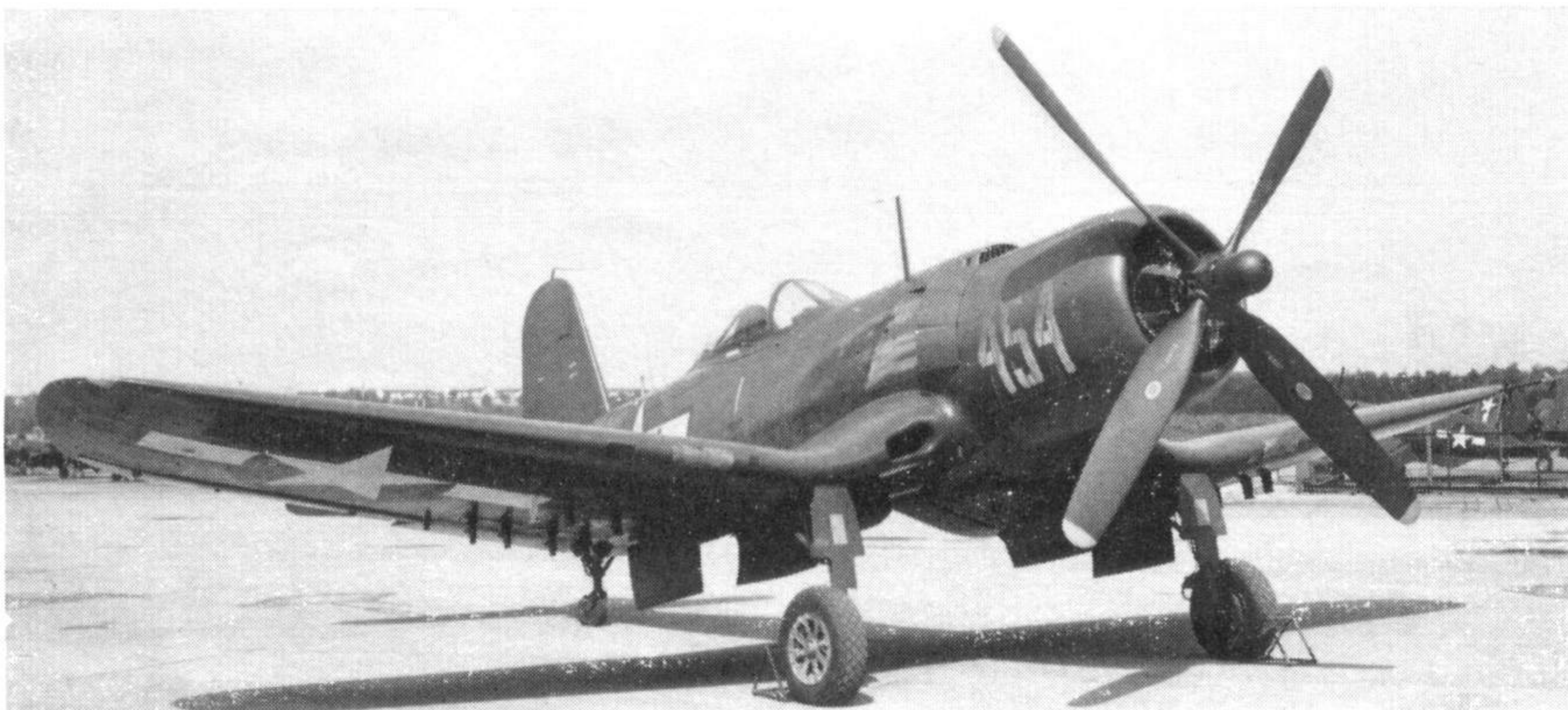
F2G-1 BuNo 88454; note the wing root inlets, smaller than those of a standard Corsair. Without a supercharger, no intercoolers were required, and only the oil coolers were fed from the wing roots. (Photo: Goodyear)
