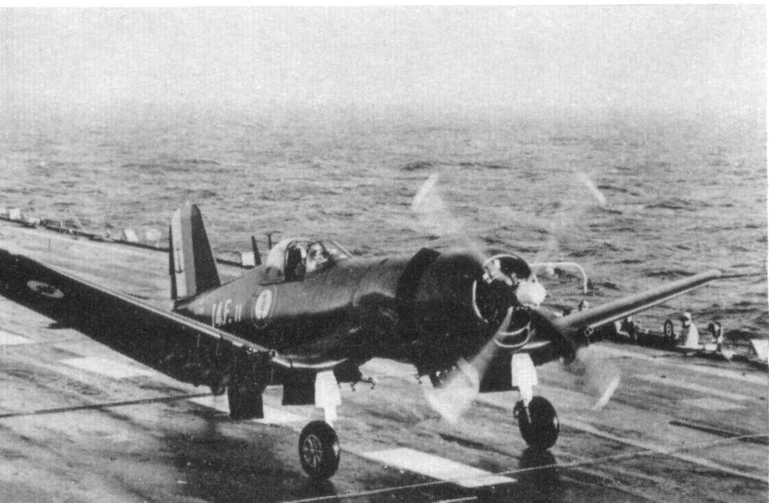
Early rounded windshield on a Korea-based F4U-4.
