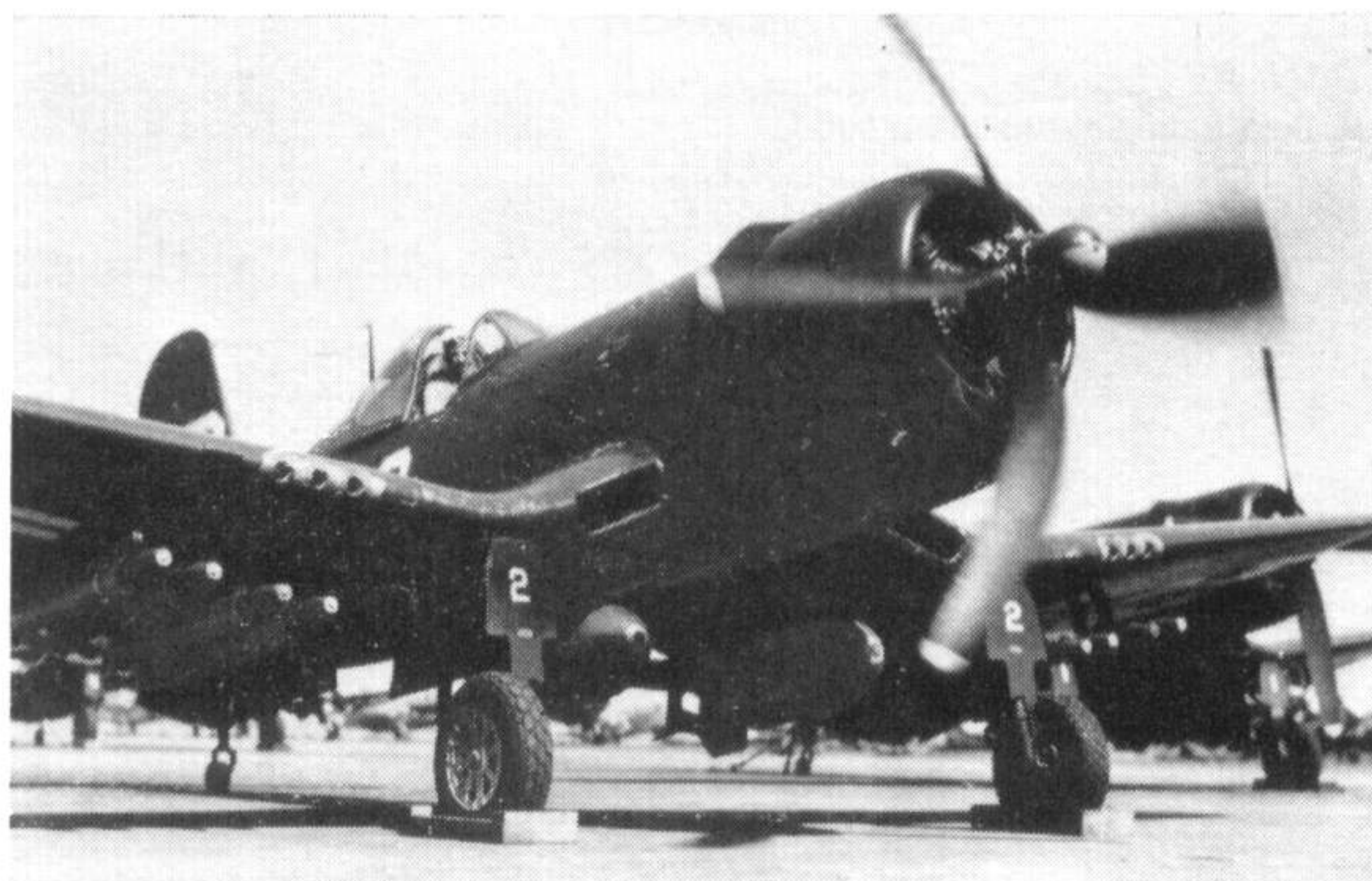
Early rounded windshield on a Korea-based F4U-4.
