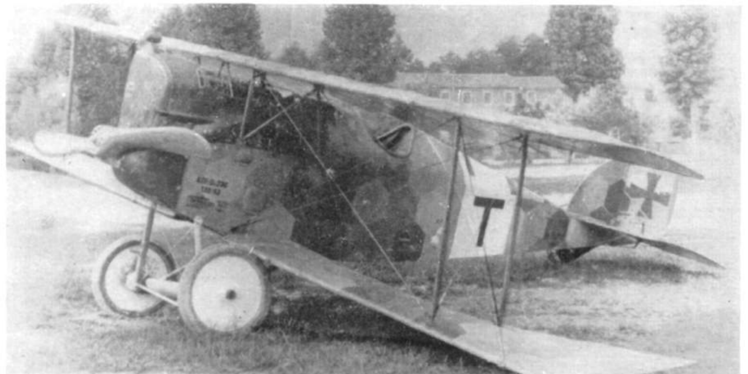
On the 23rd June 1918 Italian pilots forced this Berg, No. 138.43, to land behind the Allied lines on the Piave Front. It was powered by a 200 h.p. Austro-Daimler engine.
