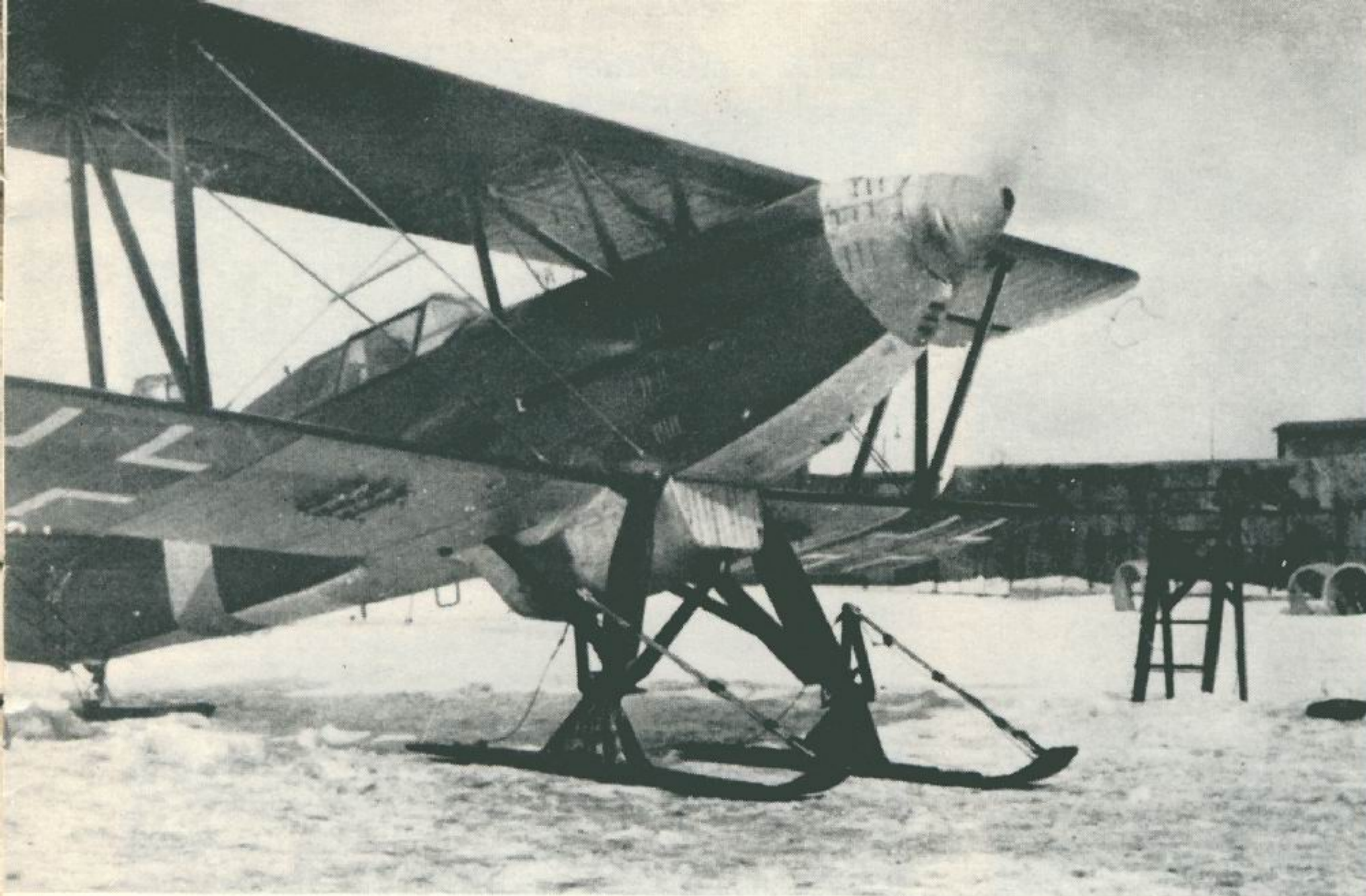
A ski-undercarriage Bk-534 at Trencin before delivery to the Slovak Air Force elements in Russia during the winter of 1941. Note olive-painted undersurface of top wing, and German-style markings on yellow tips of the lower wing. (Photo: Ing. S. Androvic)
