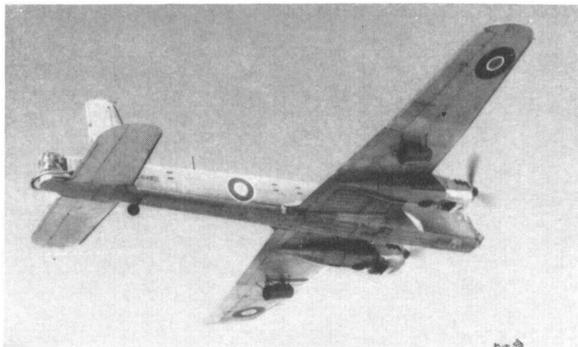
Below: Mk. V T4149 with underwing RATOG containers; used by R.A.E., Farnborough.
