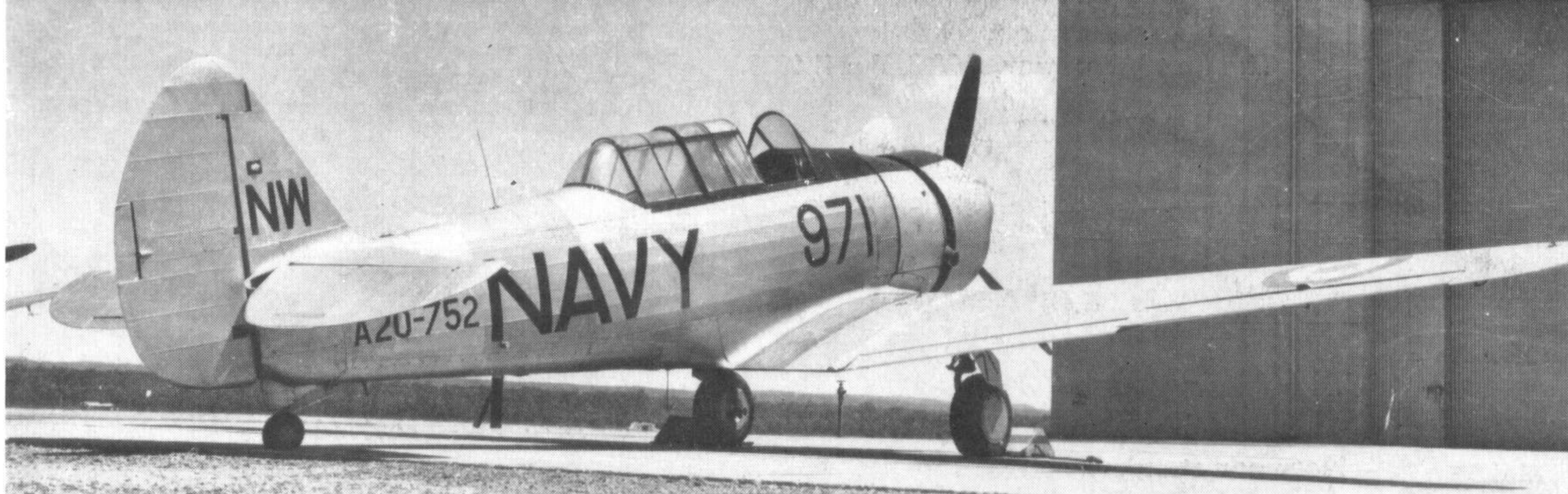
Wirraway III A20-752 was originally a CA-16 but was later converted by Commonwealth to a CA-20 (see p. 10) and used at the Royal Australian Naval Air Station, Nowra. (Photo: P. Ricketts)
