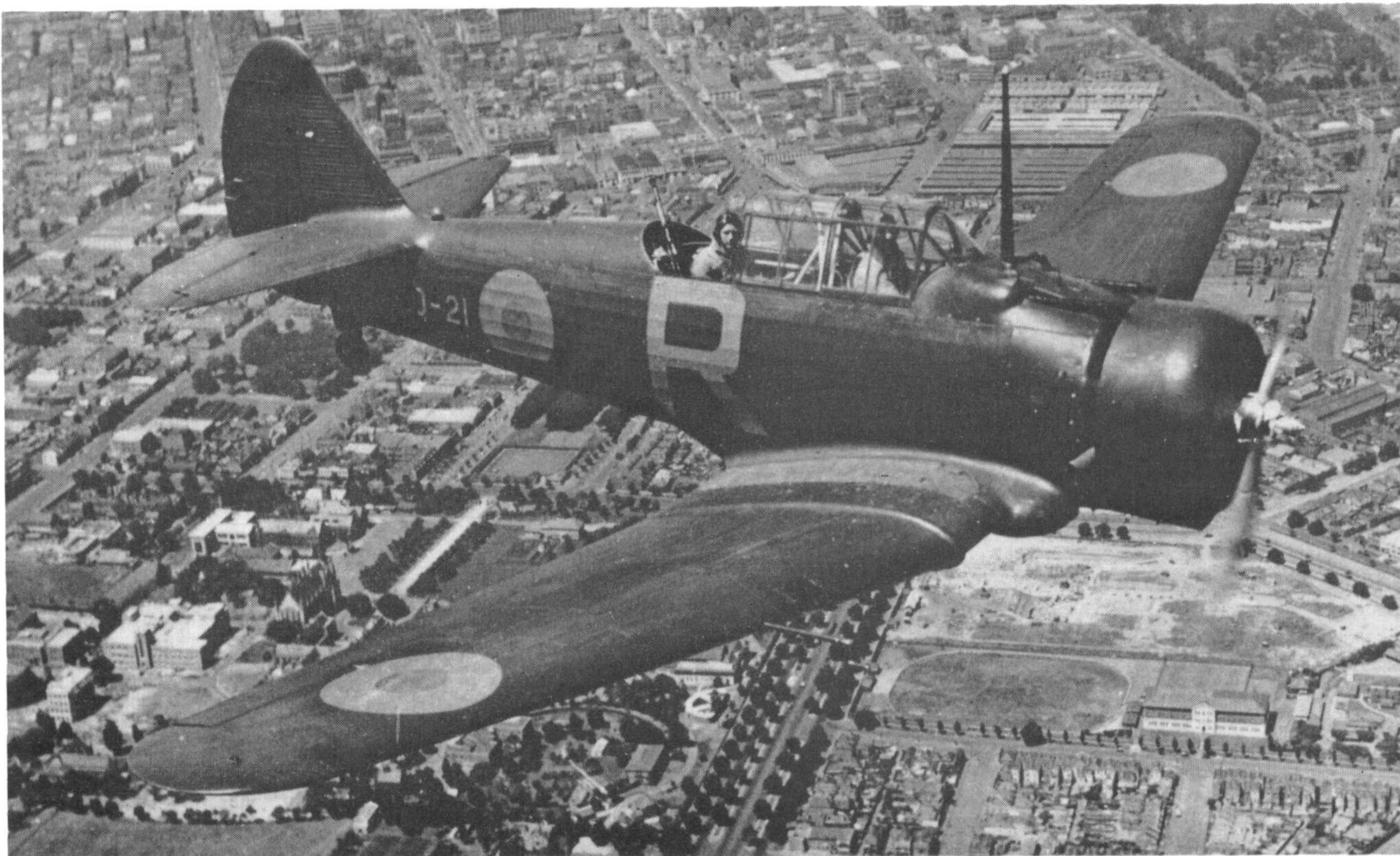
Another view of A20-21 seen here over Melbourne during 1940. Details of the fixed forward-firing guns and the flexible gun are clearly visible. (Photo: Australian War Memorial)
