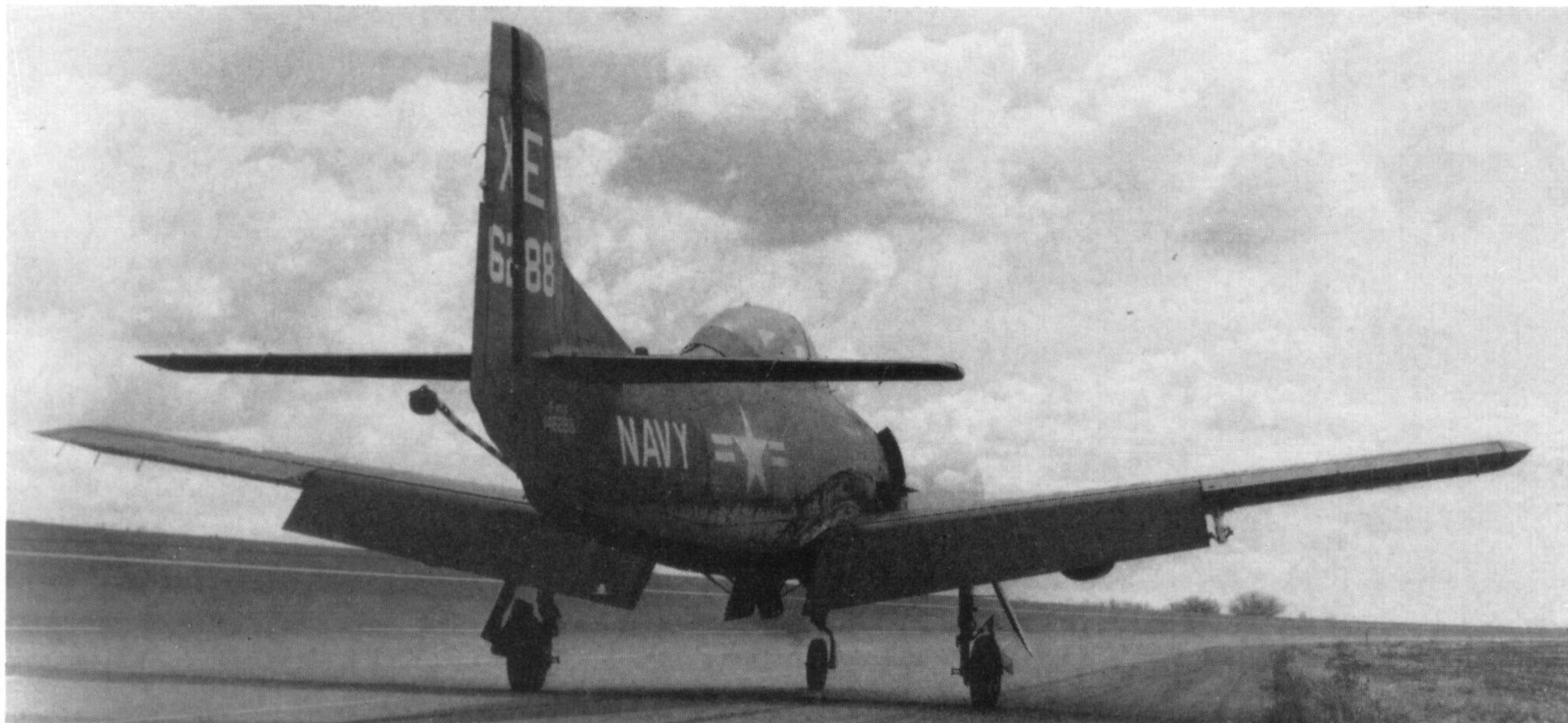
A T-28C during circular runway evaluation tests at General Motors' Mesa, Arizona, test track. Visible just below the open cowling flap is the spin recovery strip installed on T-28C's when underwing stores are carried. (Photo: U.S.N. via Naval Aviation News)
