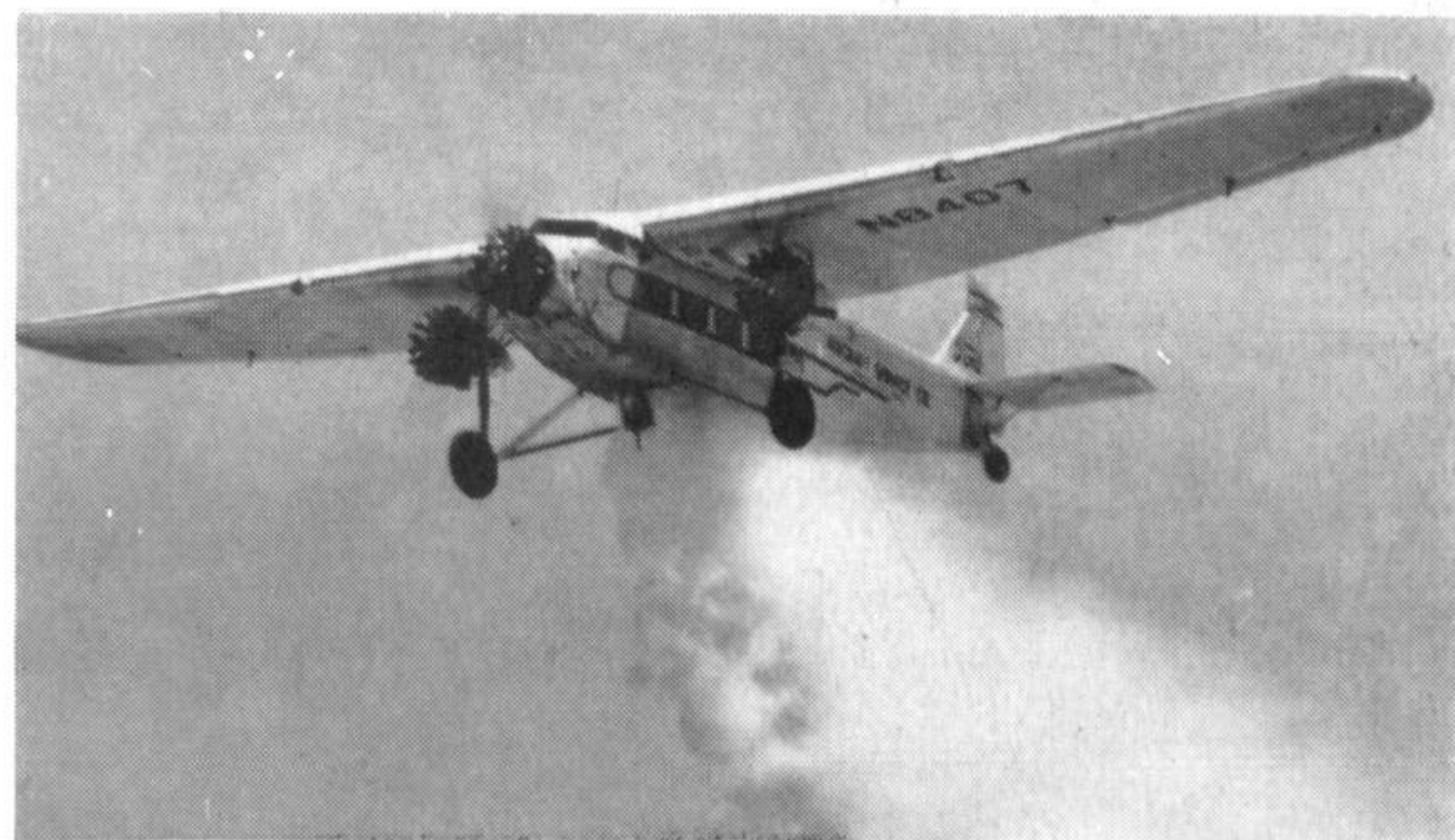
N8407 was fitted with two 275 gallon borate tanks in 1957. Pilot-operator Glen Higby used it to fight forest fires in the Boise (Idaho) National Forest. (Photo: U.S. Forest Service)
