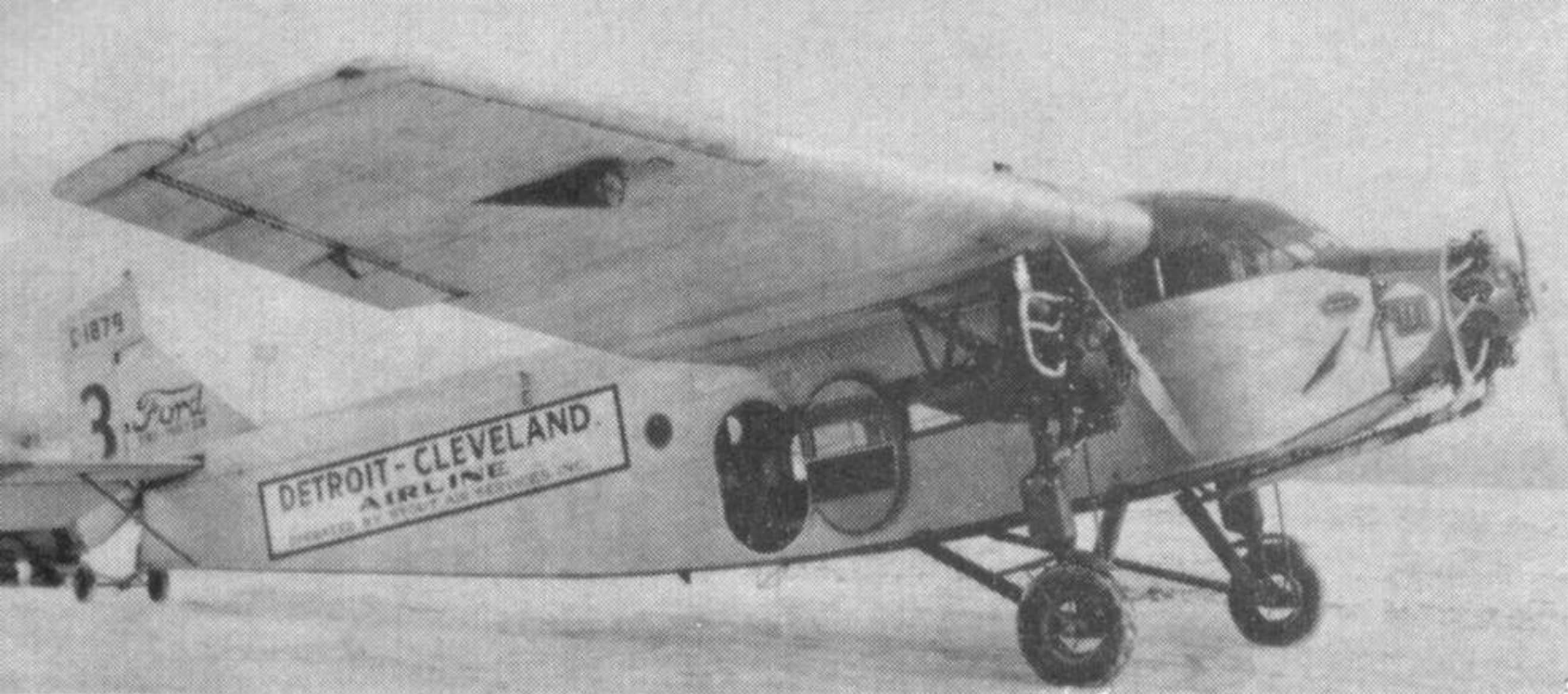
The 4-AT-A, first production model. This plane, the fifth built, shows the early design with engine exhaust going up through the wing. A 1927 photo showing early Stout Air Services.
