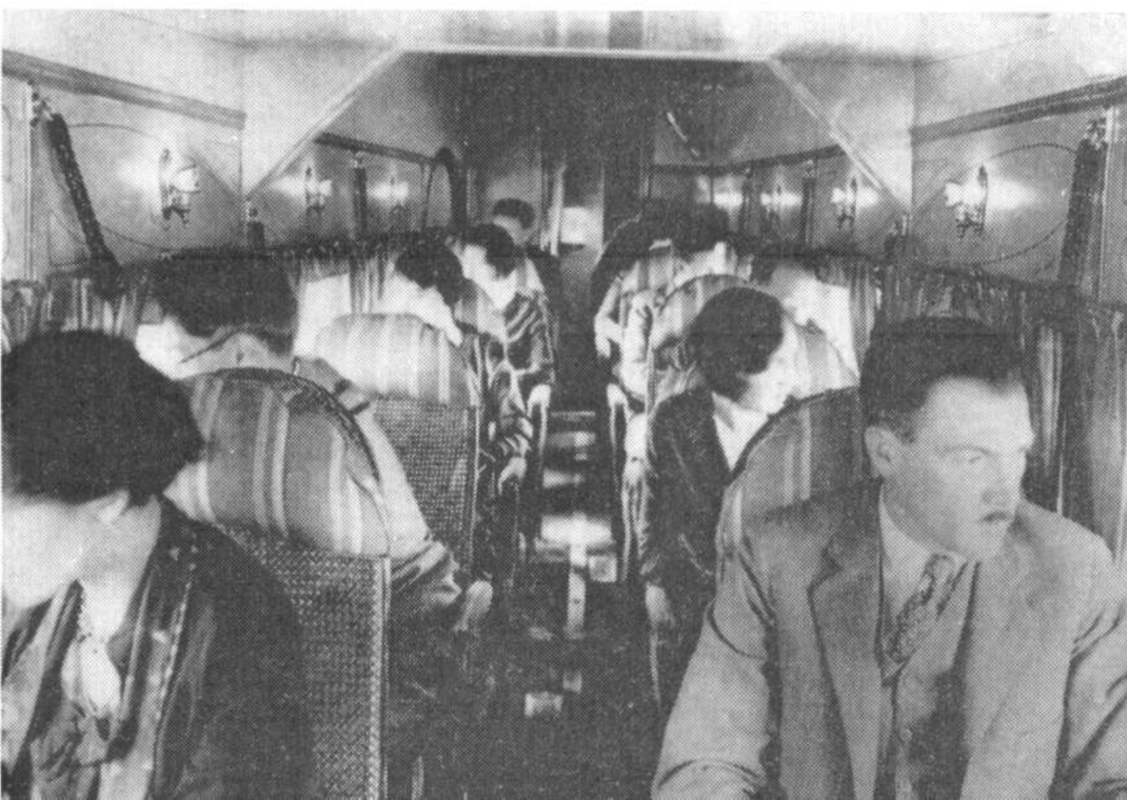
Passenger compartment of a standard airline 5-AT-B of 1929. The wicker seats were soon replaced with metal seats. (Photo: T.W.A.)
