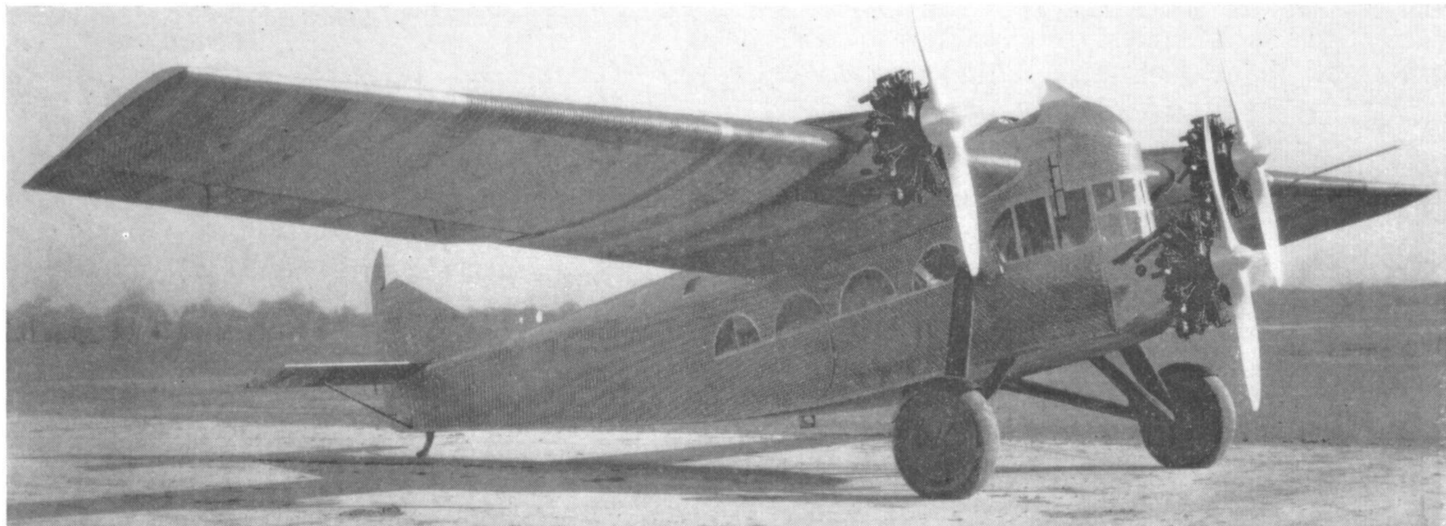
The first Tri-Motor, model 3-AT, designed and built by Bill Stout in 1925. It was a modified and enlarged 2-AT, replacing the single Liberty with three Wright J-4's of 200 h.p. each.
