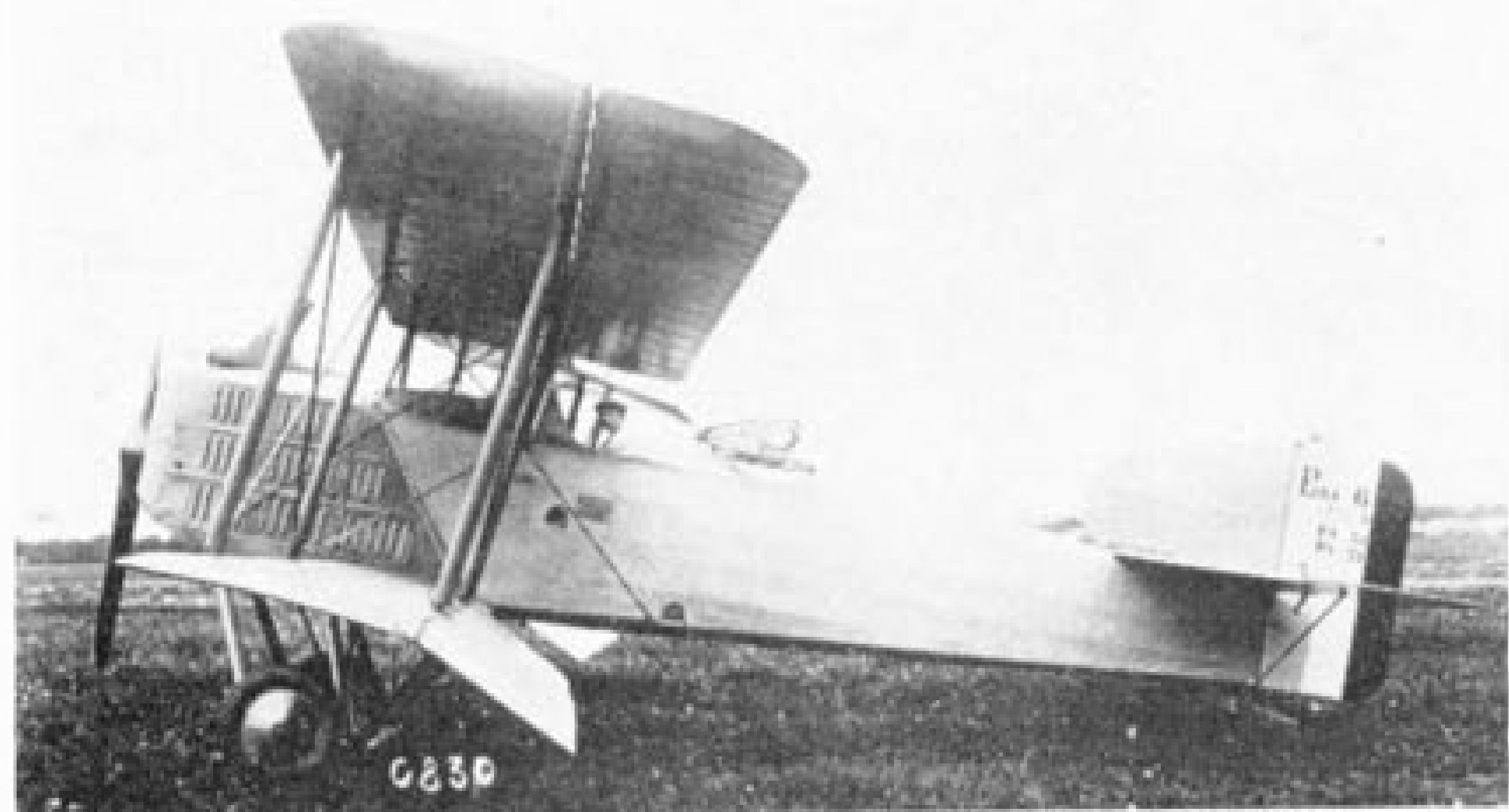
Two views of an early Breguet 14B2, No. 670. The three-quarter front view shows the greater length of the lower wing; both illustrations show the lower-wing flaps clearly. This aircraft had not been fitted with Michelin bomb racks and their characteristic forward projection of the lower-wing leading edges when this photograph was made; there were no windows in the fuselage sides at the observer's cockpit, and his gun ring was a T.O.4. No shutters were fitted to the radiator at this stage.
