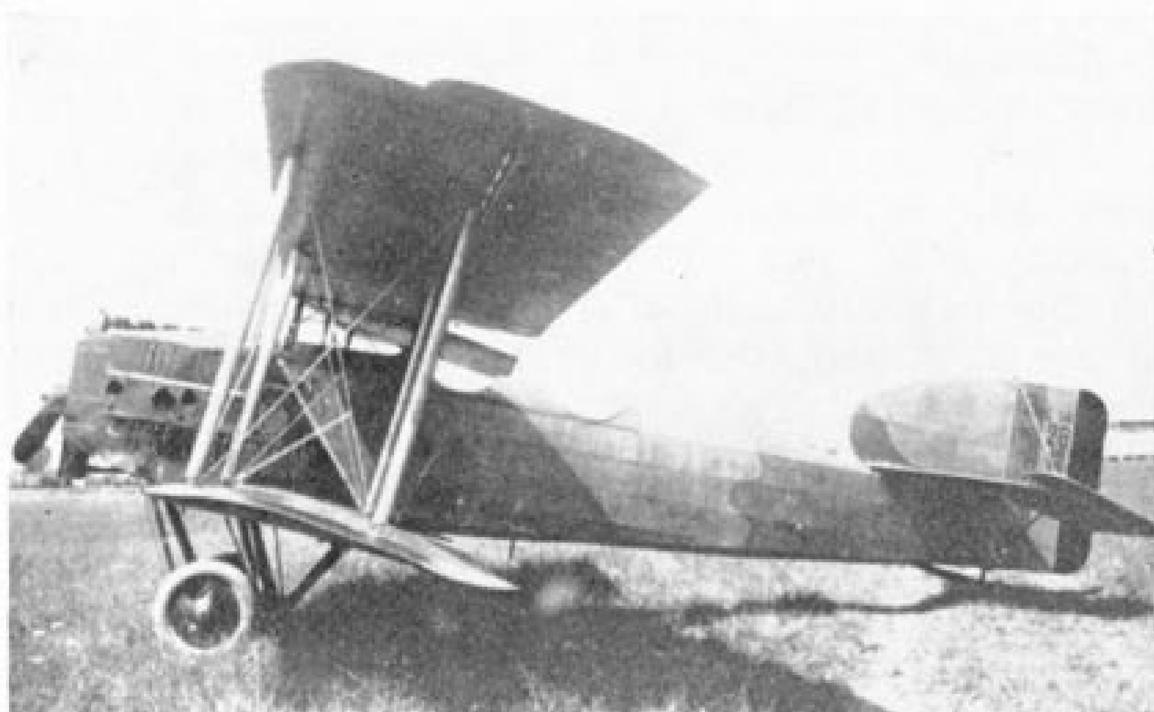
Fiat-powered 14A2 with horn-balanced ailerons and straight trailing edges on mainplanes. The engine has the enlarged radiator and all armament has been removed.
