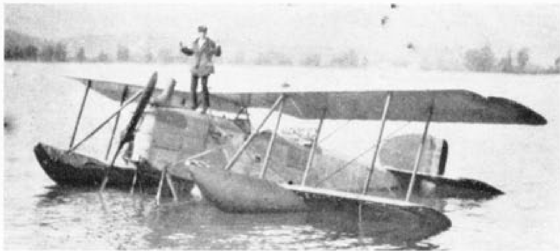
Breguet 14B2 fitted with flotation gear. The aircraft has horn-balanced ailerons, wire trailing edges, the late 14B2 lower wing and underwing skids. (Photos: Jean Noël)
