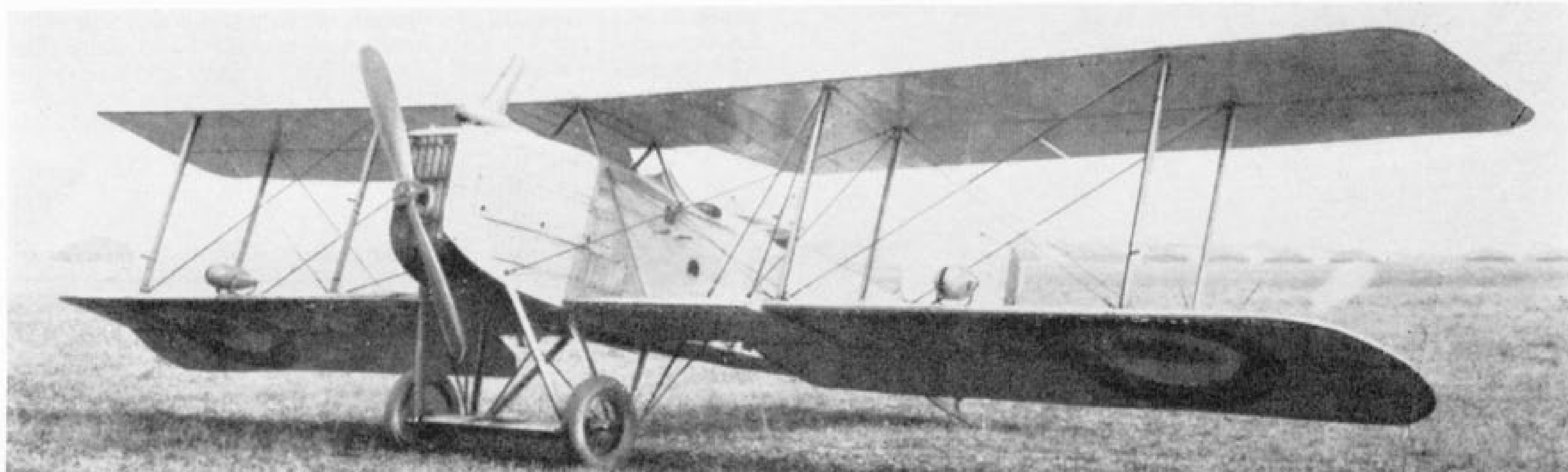
A Breguet 14B2 fitted with Brandt et Fouilleret landing lamps on the lower wings. The aircraft has the original 14B2-type wings with flaps and straight trailing edges, and the observer's gun mounting is a T.O.3. Radiator shutters are fitted. (Photo: Jean Noël)
