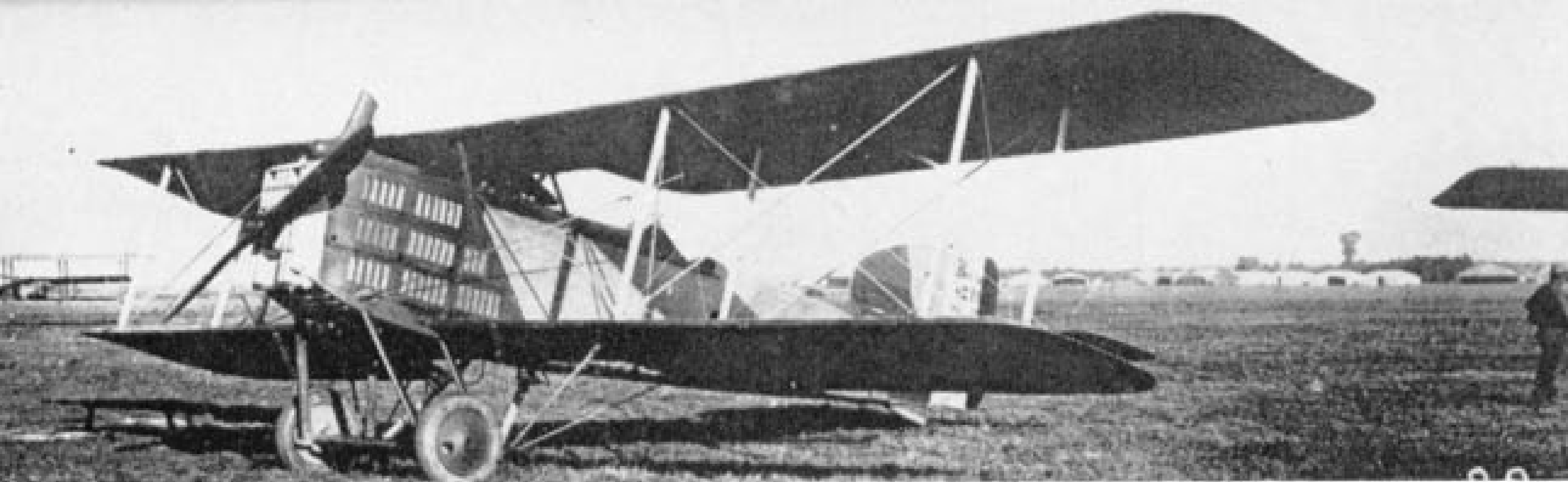
Breguet 14B1 No. 2196. This aircraft has the standard Breguet 14A2 wing arrangement, despite its bombing function. Other Breguet 14B1s had 14B2-type wings.
