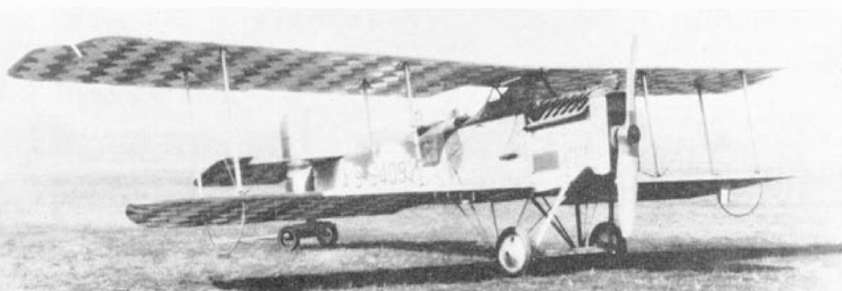
A different Liberty installation in a Breguet 14B2 at McCook Field, U.S.A. This aircraft had the revised 14B2 wing structure with horn-balanced ailerons, together with the later bomb racks that required no forward extensions of the lower-wing leading edges. It bore the U.S. Air Service number A.S.94097 and the McCook Field Project No. P-148.
