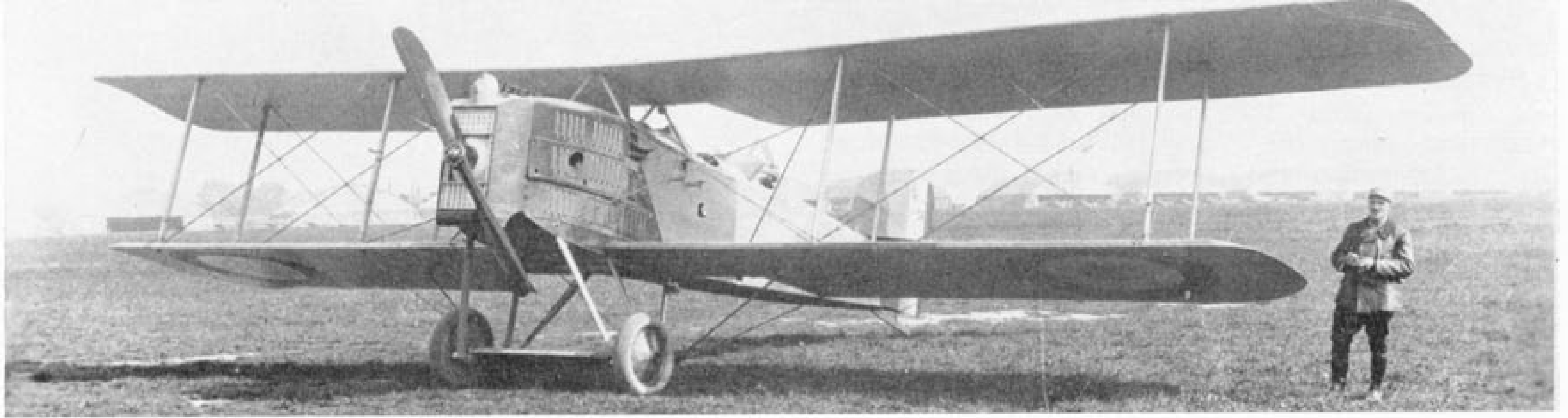
Breguet 14A2 No. 2405 with Fiat A-12 engine and frontal radiator. The aircraft has the original 14A2 wings with straight trailing edges, and inter-cockpit windshields are fitted. (Photo: Musée de l'Air 02343)
