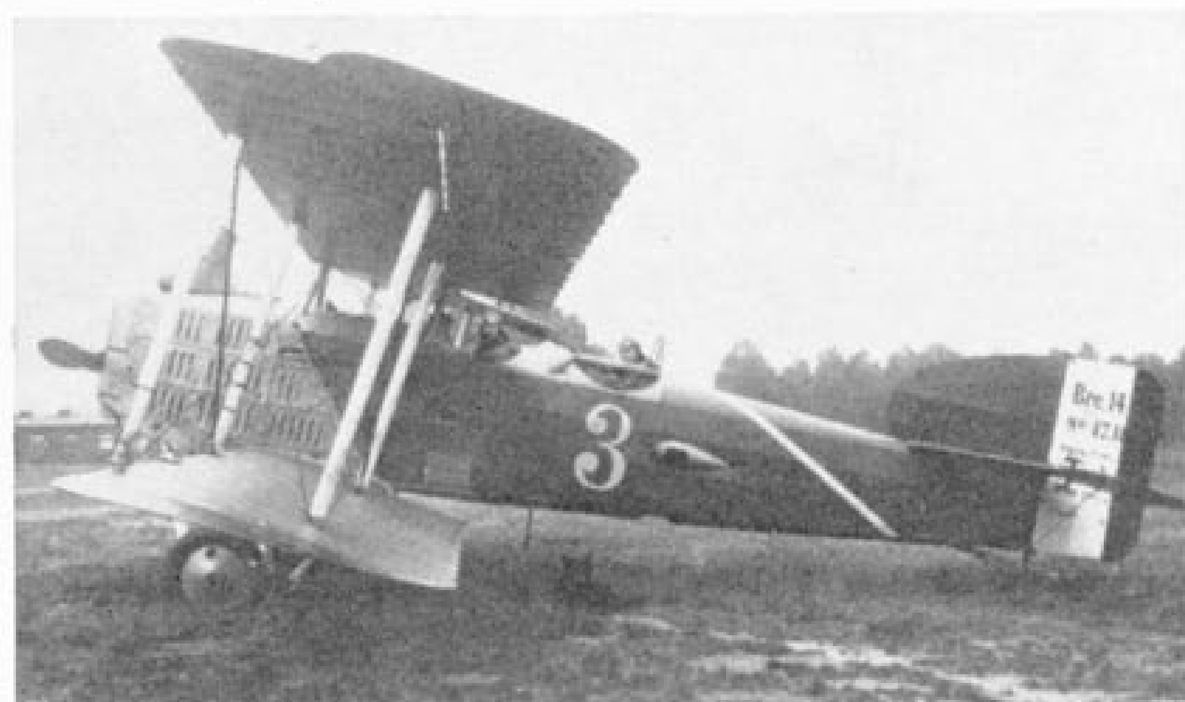
Breguet 14A2 No. 17188 with horn-balanced ailerons and wire trailing edges. Equipped for photographic reconnaissance duties, this aircraft had windshields fitted on the decking between the cockpits.
