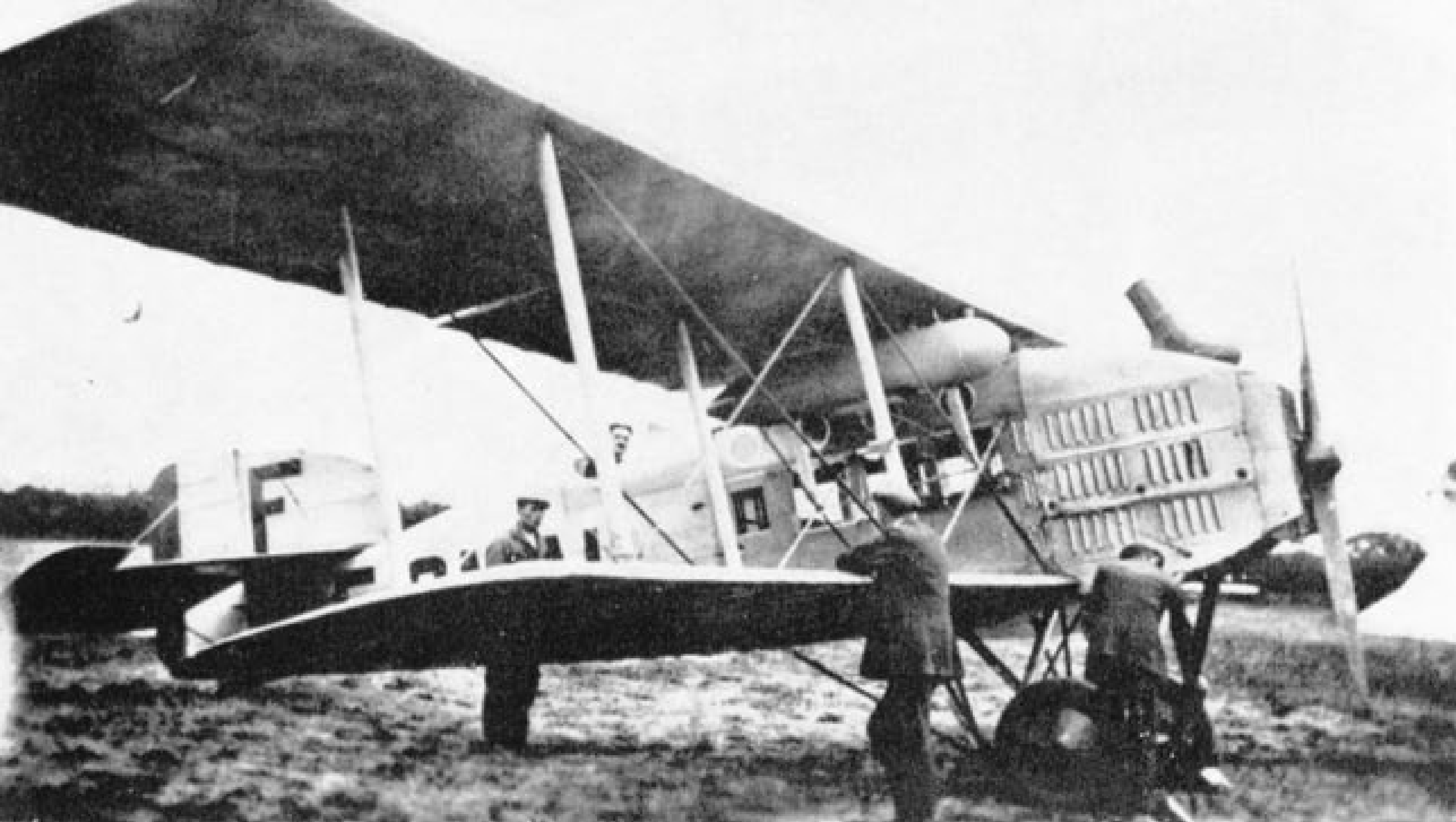
Breguet 14Tbis with the improved cabin arrangements and additional windows that distinguished it from the 14T. The bracing of the interplane fuel tanks to the intersections of the flying and landing wires is noteworthy.
