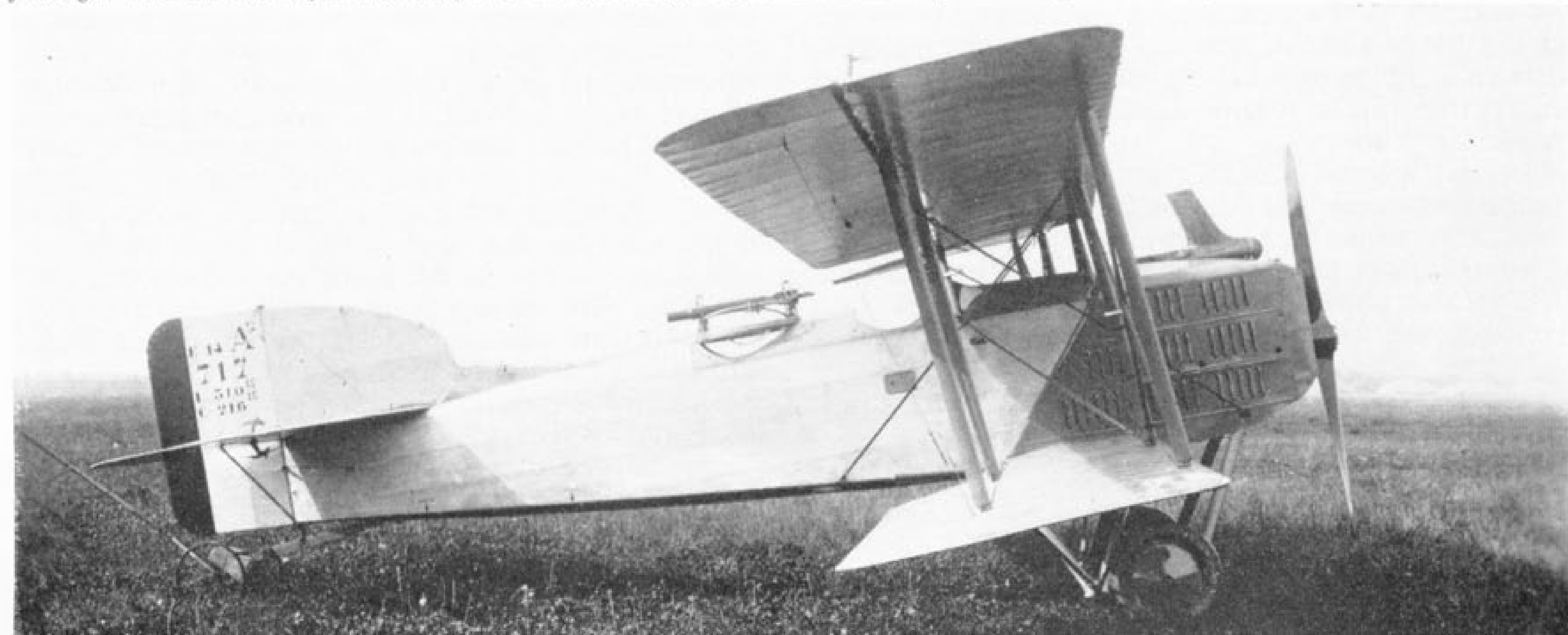
A later production aircraft, No. 717, with modified rudder having its lower edge more or less in continuation of the lower line of the fuselage. The observer's gun mounting is a T.O.3, a copy of the British Scarff mounting. (Photo: Musée de l'Air 01105)
