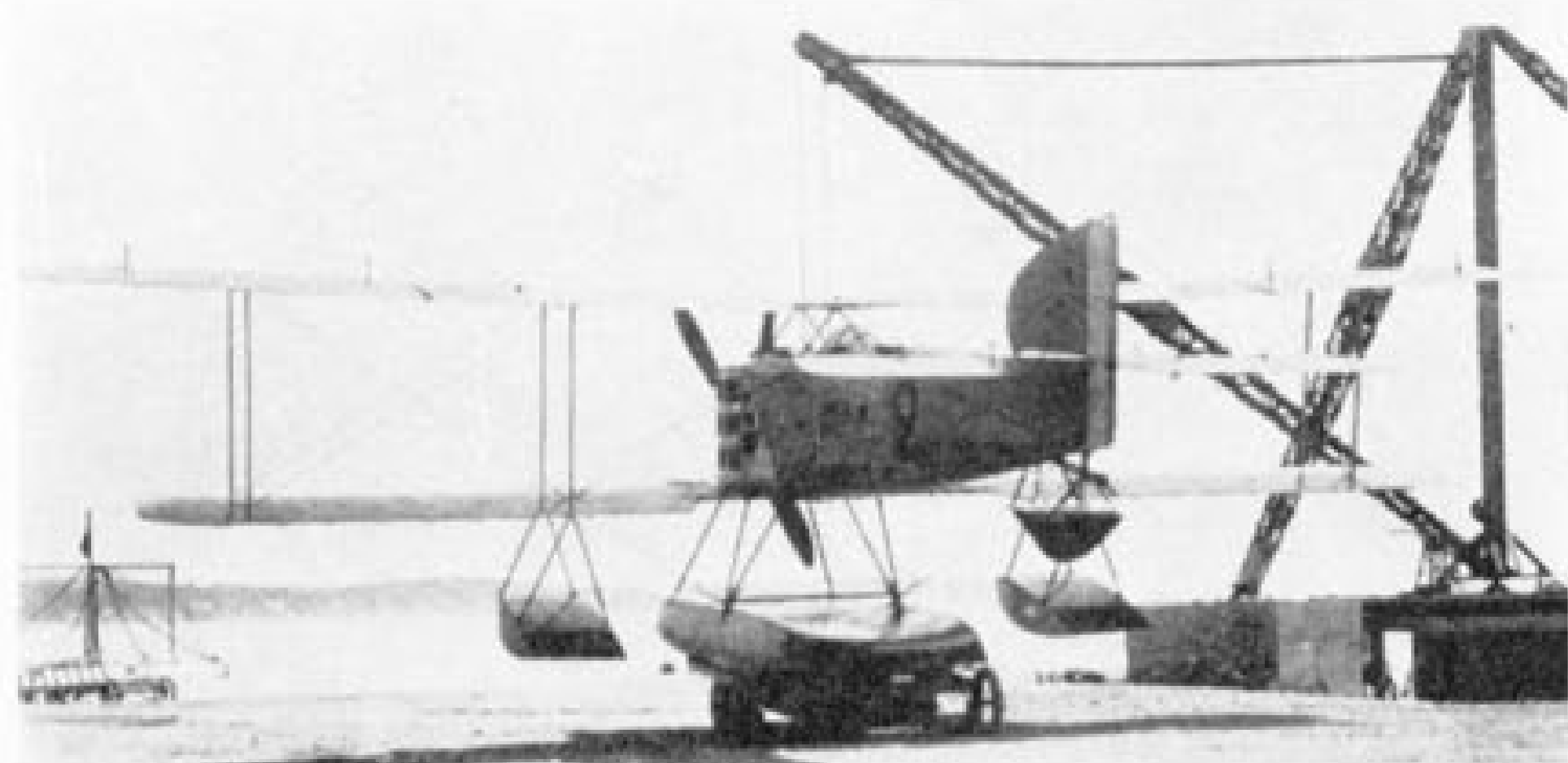
Breguet 14H. The aircraft has horn-balanced ailerons and wire trailing edges on the mainplanes; the lower wing appears to be that of a 14A2, yet the fuselage has the side windows of a 14B2.
