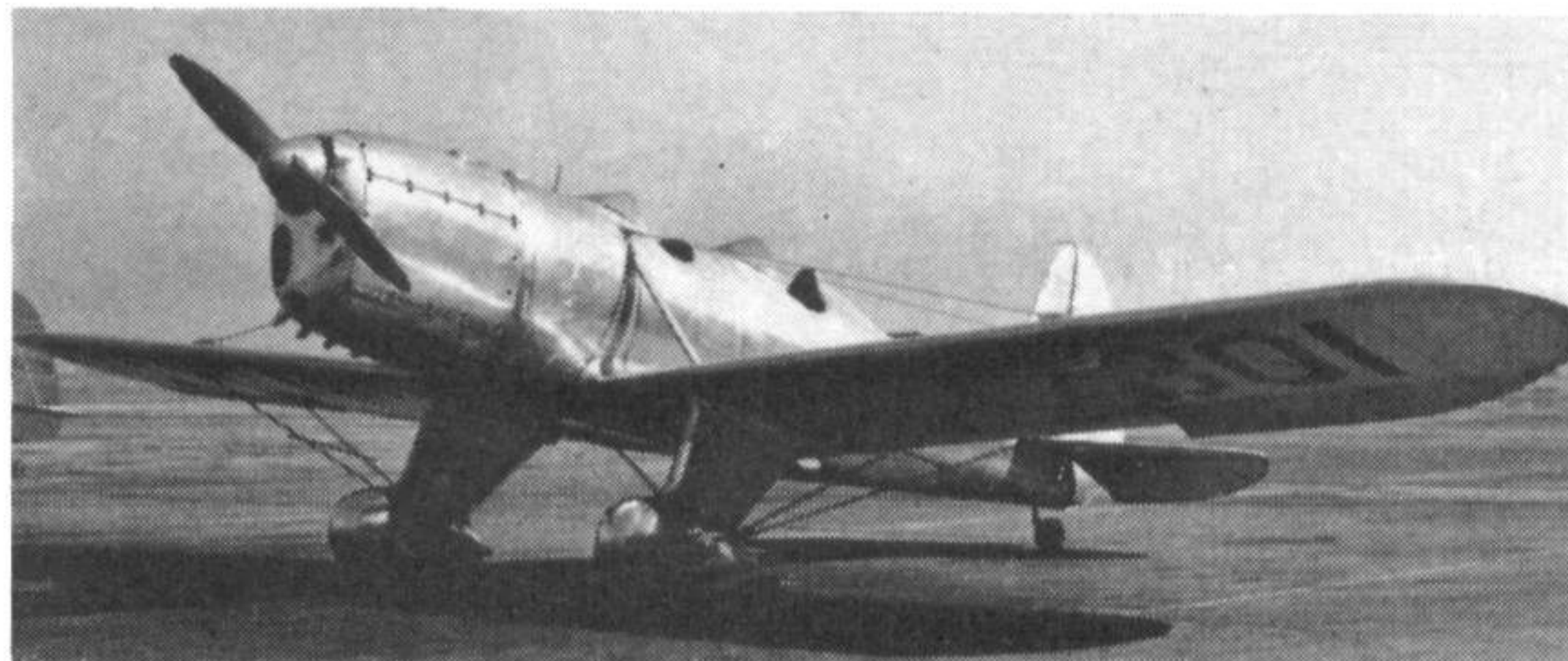
The S-T-A Special, NC17301, powered by a Menasco C-4S engine. (Photo: William T. Larkins)
