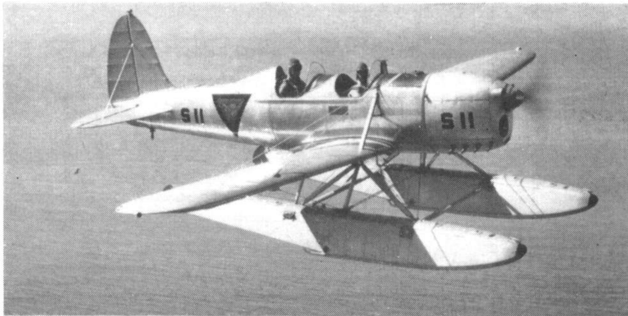
An S-T-M-S2 in Netherlands East Indies service, with optional float undercarriage installation. (Photo: Ryan)
