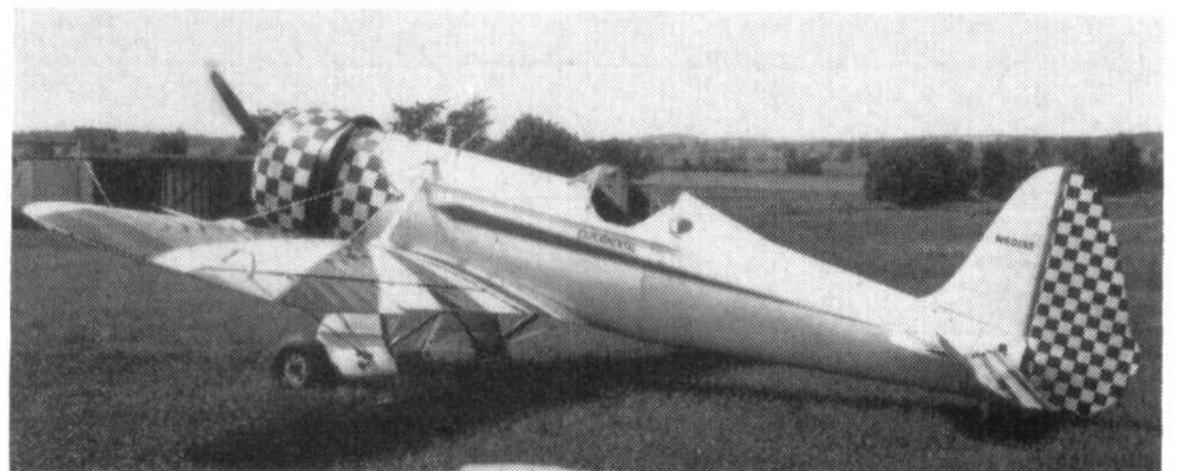
Three converted Ryans: (top) PT-22, c/n 1418 with 220 h.p. Continental engine and Twin Cessna cowling; (middle) a Ranger-powered Ryan of unknown origins; and (below) PT-22, c/n 2056, N60155, with Continental R-670-4 engine.
