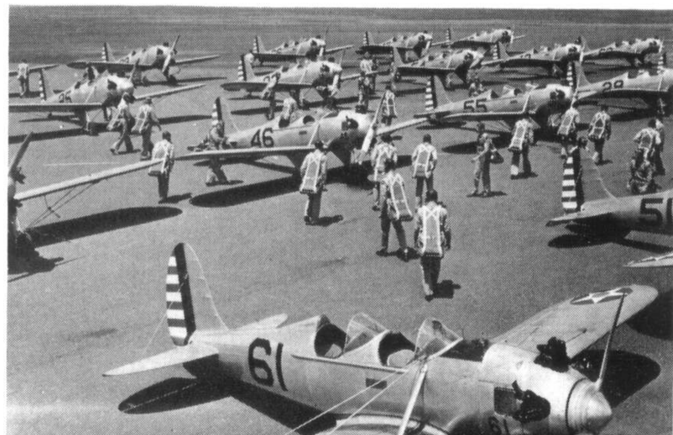
Random mixture of PT-20A and YPT-16 aircraft in "tie-down area"; essentially the same aircraft by this stage, they display mixed propeller installations. Some of each type have metal airscrews with no spinners and wooden airscrews with spinners.
