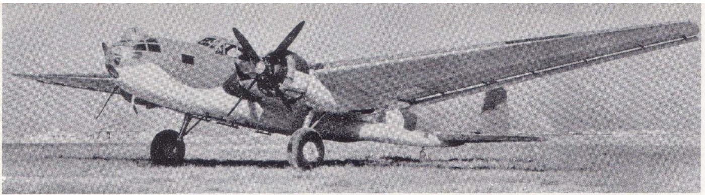
A Ka-15 powered by a pair of Kinsei 2 engines driving fixed pitch four-blade wooden propellers as seen during flight trials. (Photo: via the author)
