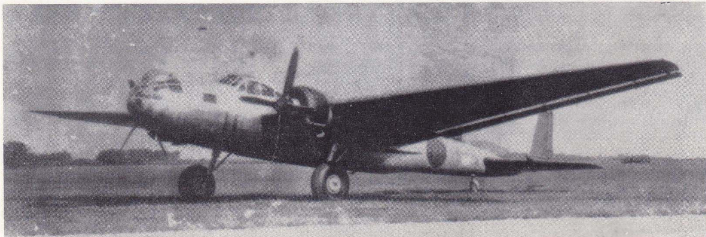
One of fifteen Mitsubishi Ka-15 prototypes fitted with a bombardier position in a "greenhouse" nose.
