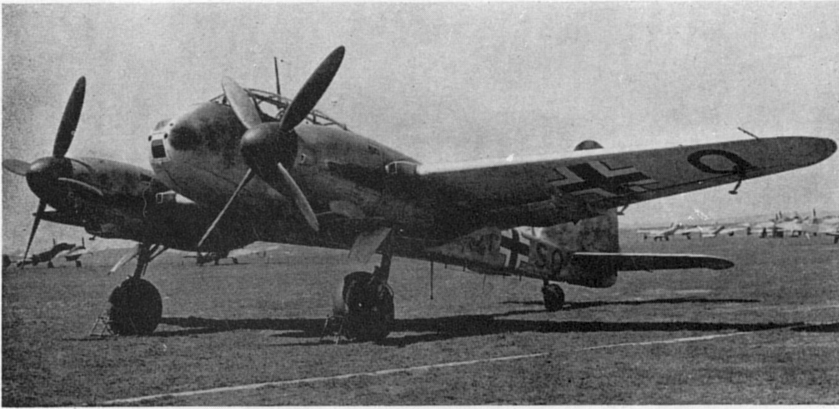
The Me 210 V13 was specially modified as a prototype for the Me 310, with four-bladed airscrews and a pressurized cockpit. (Photo: H. J. Nowarra)
