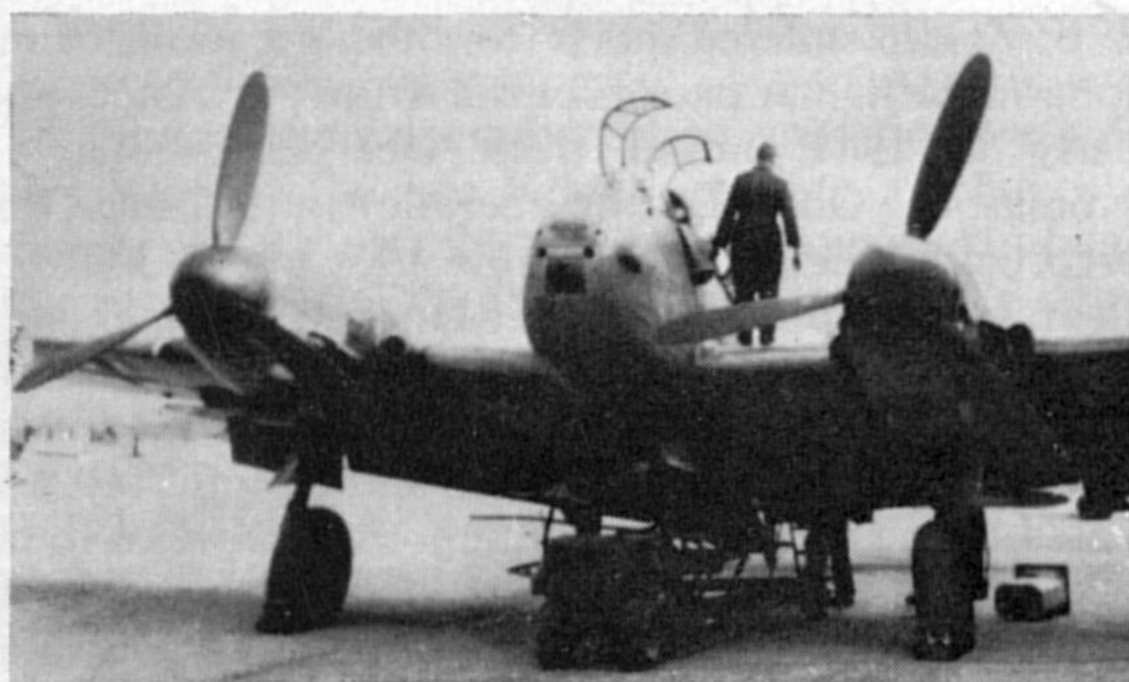
An Me 410 experimentally fitted with an LT-950 torpedo under the fuselage. (Photo: H. J. Nowarra)
