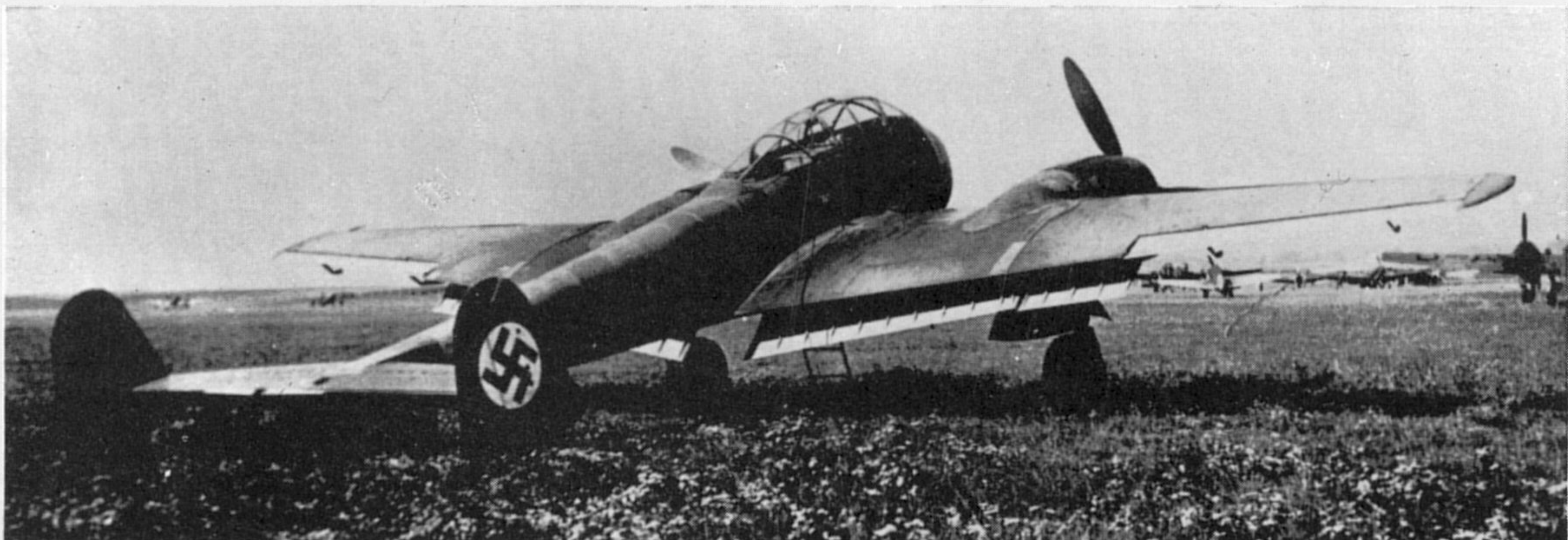
D-AABF, the first Me 210 prototype; apart from the obvious feature of the twin tail, the early cockpit canopy is noteworthy.
