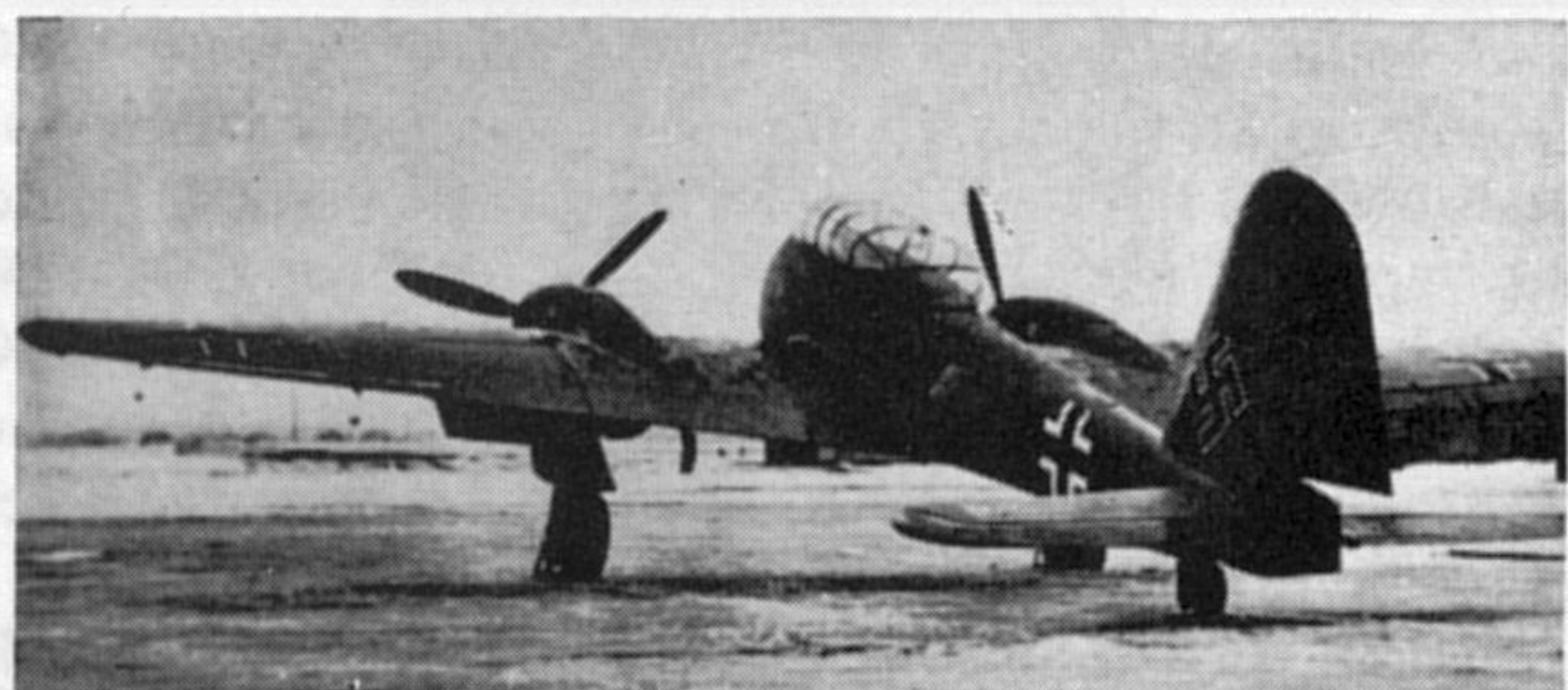
The revised cockpit and single tail of the second prototype, Me 210 V2. Despite the modified tail the machine was extremely unstable, and crashed during flutter tests on September 5, 1940.
