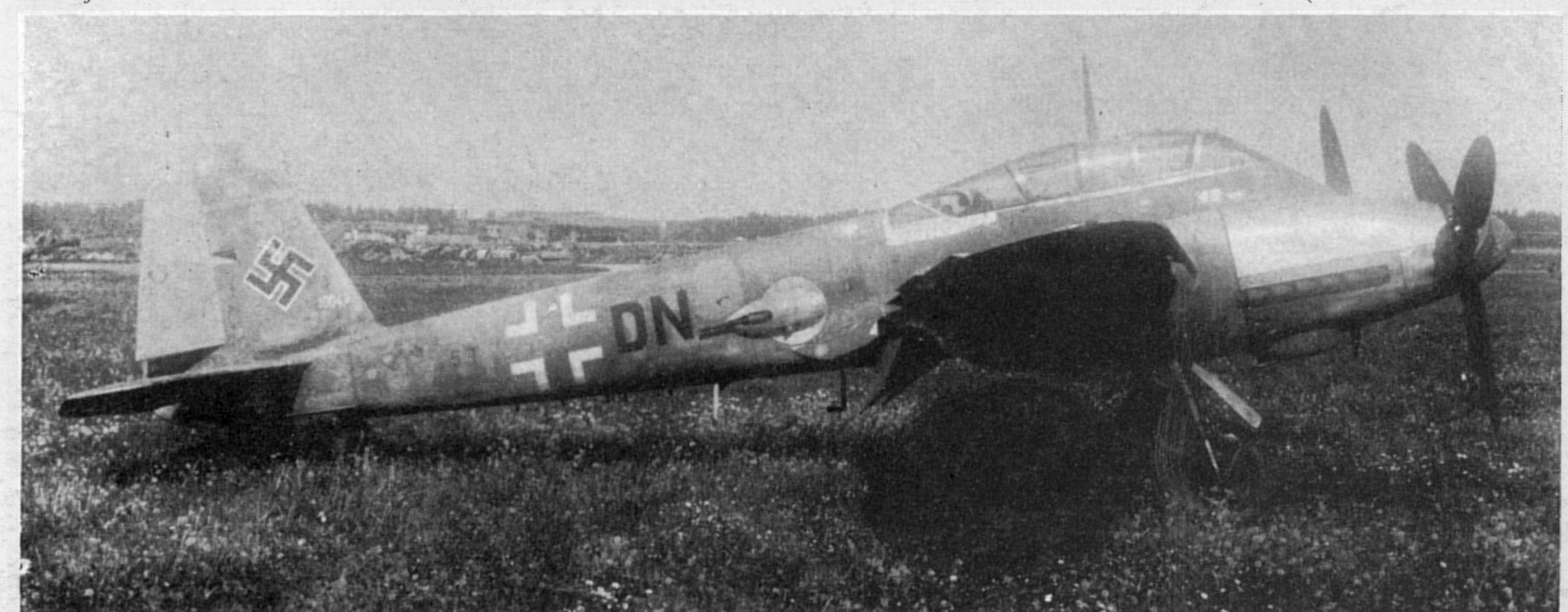
Messerschmitt Me 410A-3, W.Nr.10047, "5T+DN" of an unidentified reconnaissance unit. It will be noticed that the cowlings, barbets, cockpit framing and rudder are still in bare metal finish, possibly indicating replacement parts hastily fitted to a damaged aircraft. (Photo: H. J. Nowarra)
