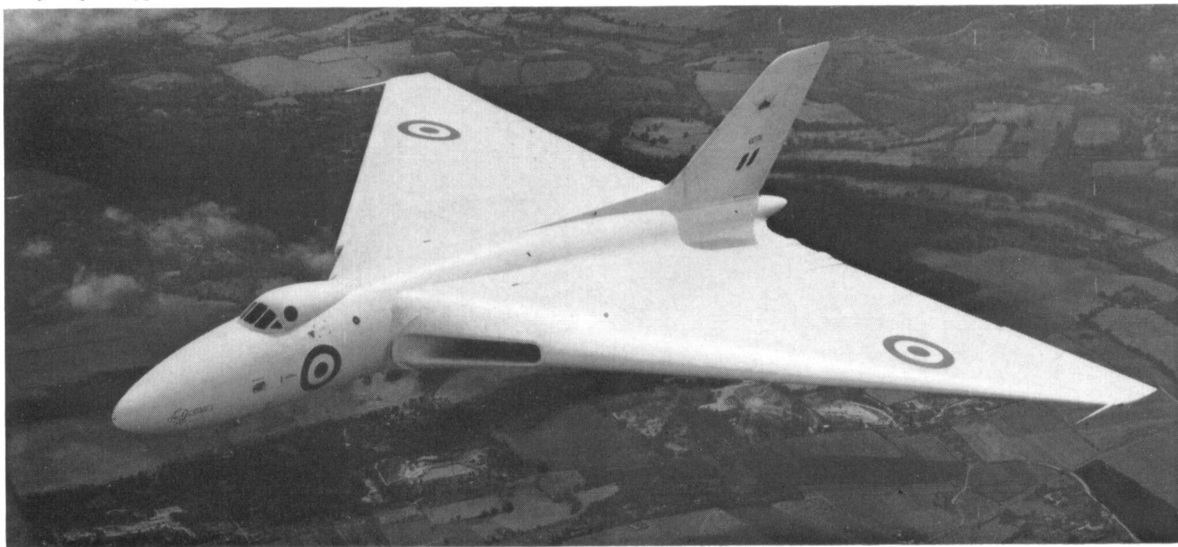
The first prototype Avro 698 Vulcan, VX770, showing the initial, undistorted delta wing planform. (Photo: Avro)
