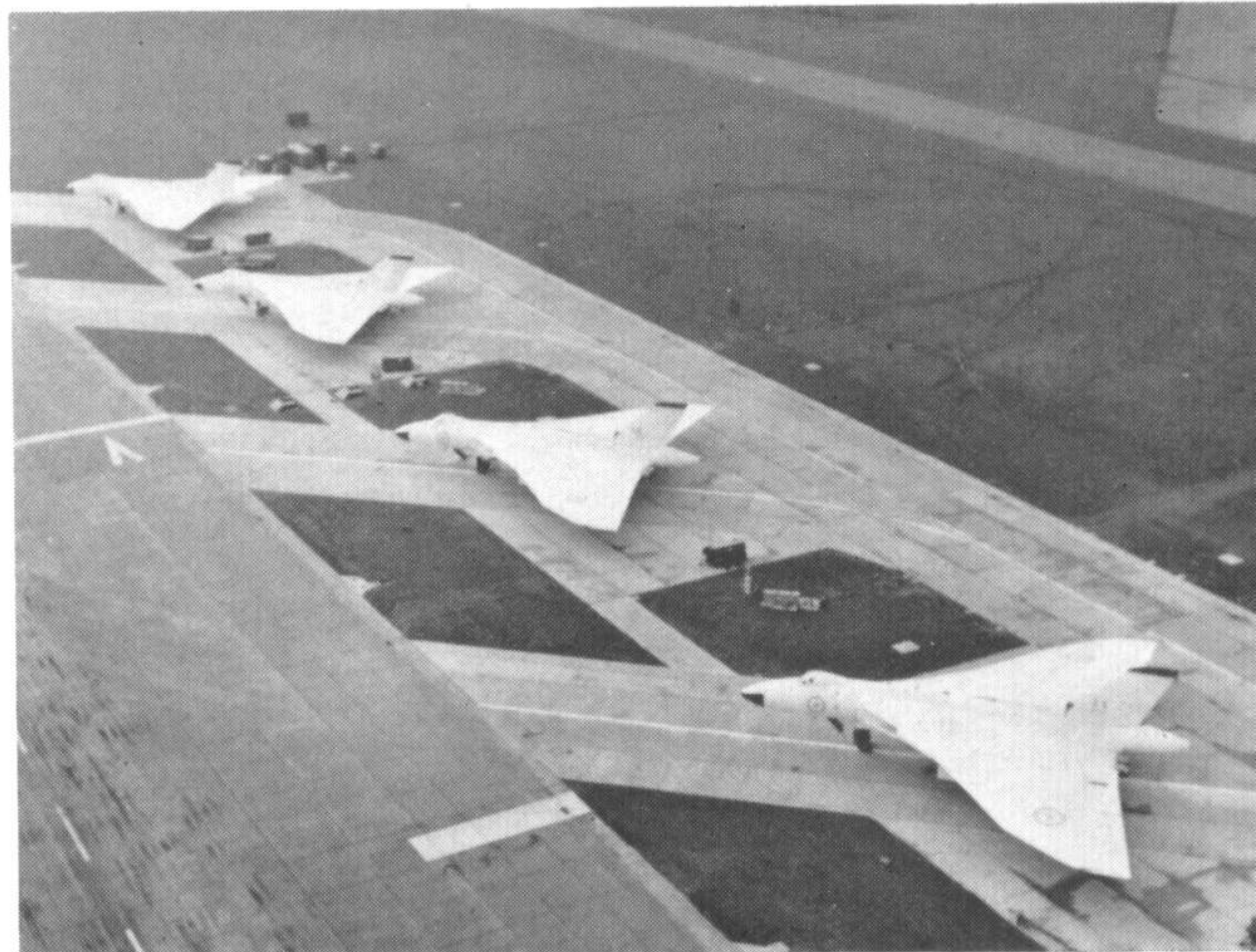
Four Vulcan B.2's on their O.R.P.'s (Operational Readiness Platforms) angled into the side of the runway to speed "scrambling". (Photo: M.o.D.)
