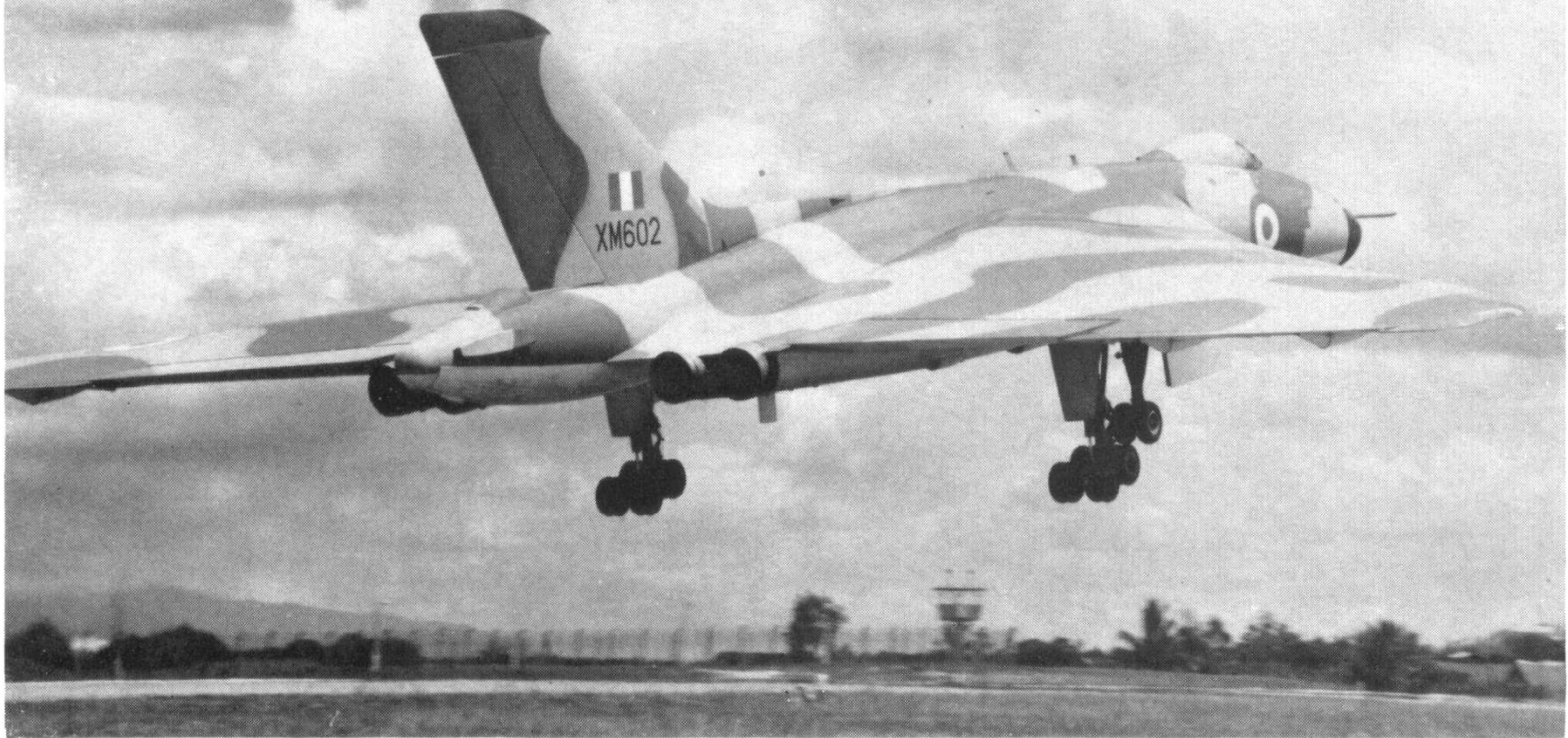
A Vulcan B.2 seen just after unsticking, showing details of the tail cone which contains radar countermeasures equipment.
