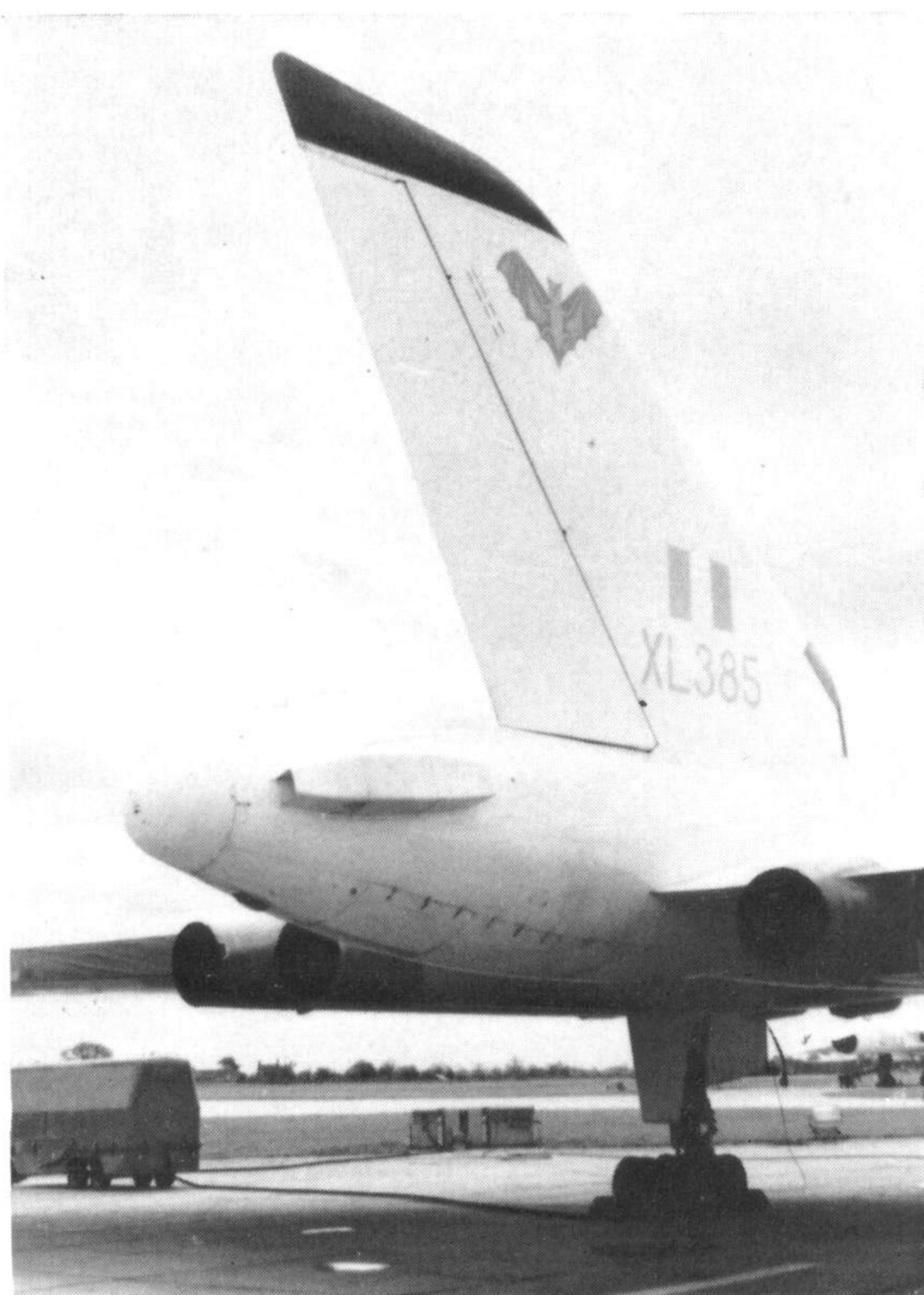
A close-up of B. Mk. 2 XL385 of No. 9 Sqn. showing the extended tailcone housing R.C.M. equipment.
