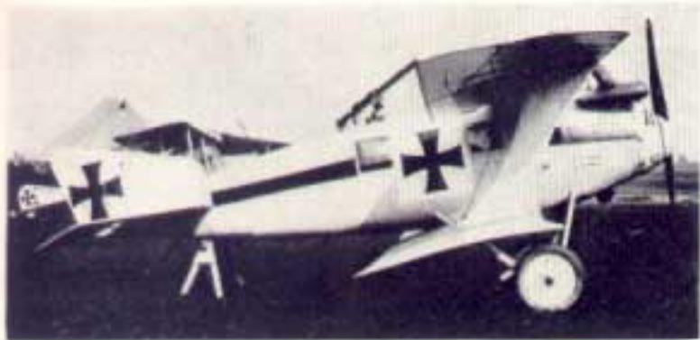
Ready for action; a Roland C.II of Kampfgeschwader I, Staffel 6 at Mont near Verdun. The type first saw combat above the horror of Verdun, armed at that time only with an LMG 14 Parabellum in the observer's position.
