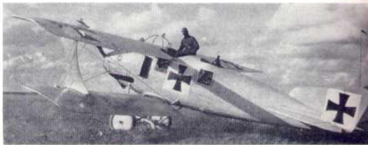
Oberleutnant Ritter von Schleich of Feld Flieger Abteilung 2b in his Walfisch : note the rear view mirror on the crash pylon and the "pilot fish" on the anemometer airspeed indicator strut. In the close-up can be seen the Roland trade-mark under the forward window, the foot step cover (not a window) in the centre of the cross insignia, and the restriction of forward vision by the ear-type radiators.
