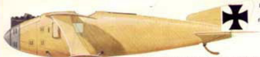
Roland C.II prototype powered by 160 h.p. Mercedes D.III engine; October 1915.
