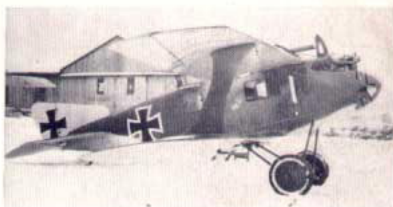
This view shows more details of the Linke-Hofmann exhaust stack characteristics.
