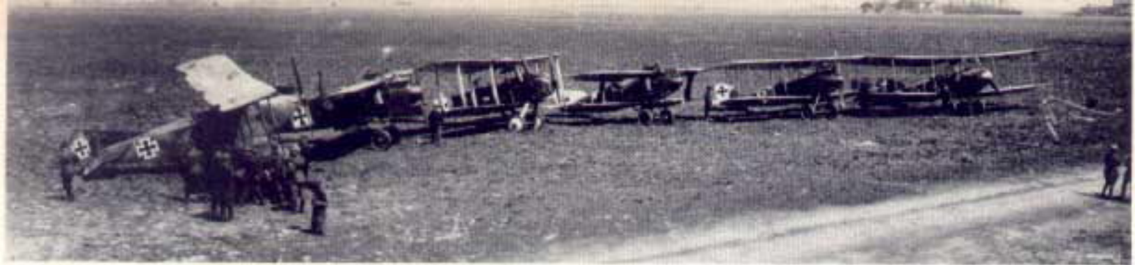
German two-seater squadrons were usually equipped for general purpose missions, as demonstrated by the variety of types making up the strength of Flieger Abteilung (A)292 in May, 1917. The small size of the Walfisch is immediately apparent. From left to right: AEG C.IV 6657/16; Roland C.II 2700/16 series; LVG C.IV; Roland C.II; DFW C.V; and Albatros C.V.
