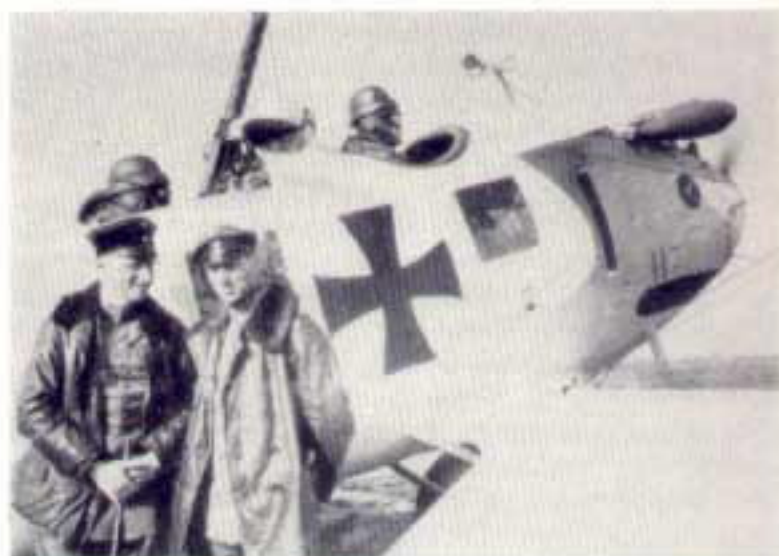
Above: a Walfisch prepares to take off; note how deep in the fuselage the crew are seated and the pilot's restricted forward vision of airfield terrain. Below: a close-up showing neat cowling, streamlined exhaust stack and claw brake on undercarriage axle: this photograph is dated April, 1916.
