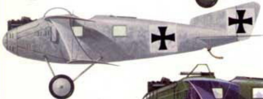
Roland C.II, 4437/15, flown by Lt. von Hippel at Jagdstaffelschule Fomars in January 1917. Note grey paint smeared over basic blue-grey finish and white ground of national insignia. The national insignia on the wing surfaces were left untouched.
