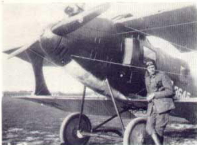
Leutnant von Hippel with his Roland C.IIa(Li). Note circular Linke-Hofmann trademark beneath, and the aileron control rod behind, the radiator. Racks for four 12.5 kg. bombs can be seen under the centre-section. (Photo: von Hippel)
