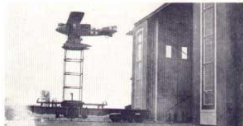
Hoping to develop a correlation with the many hours of wind-tunnel testing, the makers tested a full-scale production Walfisch on a high-speed railroad track: results were unfortunately inconclusive.
