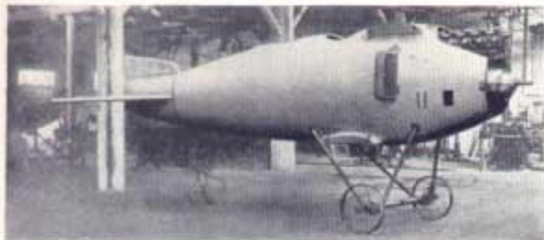
Fuselage and completed airframe of the C.II prototype. In these Roland brochure pictures the single window of the prototype can be seen to have been fitted at a late stage; it provided illumination in the deep fuselage and an emergency exit in case of a crash. No crash pylon was fitted to the prototype.
