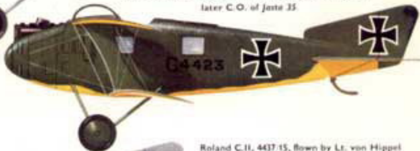
Roland C.II, 4437/15, flown by Lt. von Hippel at Jagdstaffelschule Fomars in January 1917. Note grey paint smeared over basic blue-grey finish and white ground of national insignia. The national insignia on the wing surfaces were left untouched.
