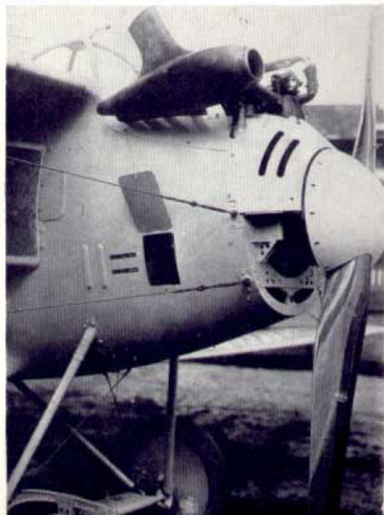
Above: a Walfisch prepares to take off; note how deep in the fuselage the crew are seated and the pilot's restricted forward vision of airfield terrain. Below: a close-up showing neat cowling, streamlined exhaust stack and claw brake on undercarriage axle: this photograph is dated April, 1916.
