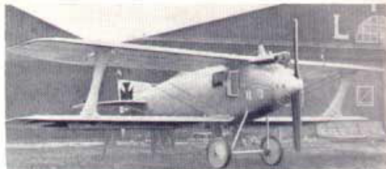
Fuselage and completed airframe of the C.II prototype. In these Roland brochure pictures the single window of the prototype can be seen to have been fitted at a late stage; it provided illumination in the deep fuselage and an emergency exit in case of a crash. No crash pylon was fitted to the prototype.
