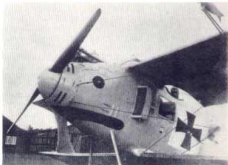
Oberleutnant Ritter von Schleich of Feld Flieger Abteilung 2b in his Walfisch : note the rear view mirror on the crash pylon and the "pilot fish" on the anemometer airspeed indicator strut. In the close-up can be seen the Roland trade-mark under the forward window, the foot step cover (not a window) in the centre of the cross insignia, and the restriction of forward vision by the ear-type radiators.
