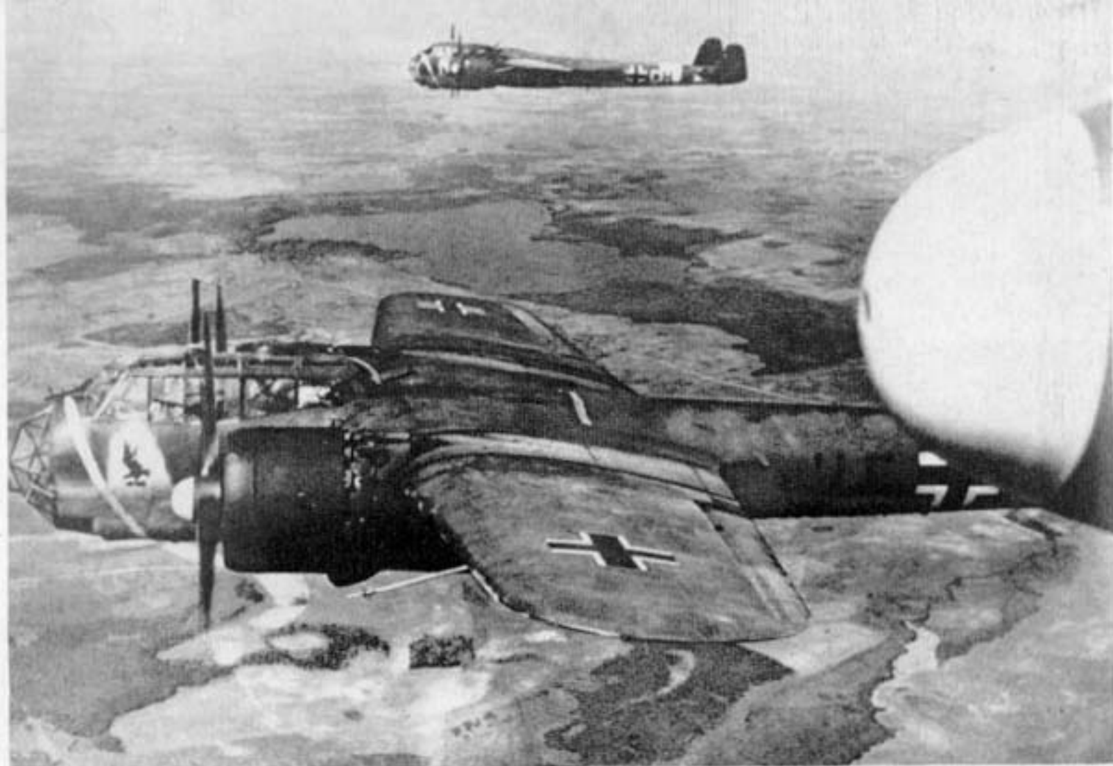
A formation of Do 17Z's of the Holzhammer Geschwader during operations in the East. By this stage in its career the Dornier often carried one or two additional beam guns in the centre cockpit windows. (Photo: R. Ward Coll.)
