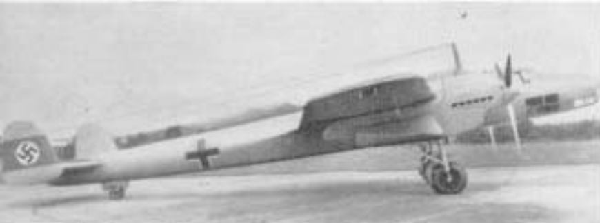
The Do 17MV-1 was a high-speed machine powered by DB 600A engines; it caused something of a sensation at the Zurich Competition of July 1937, achieving a speed of 284 m.p.h. (Photo: J. W. Caler Collection)
