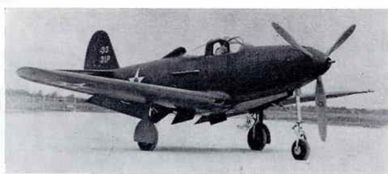
A P-39C of the 31st Pursuit Group; note lack of wing guns. (Photo: A. G. Simmons)
