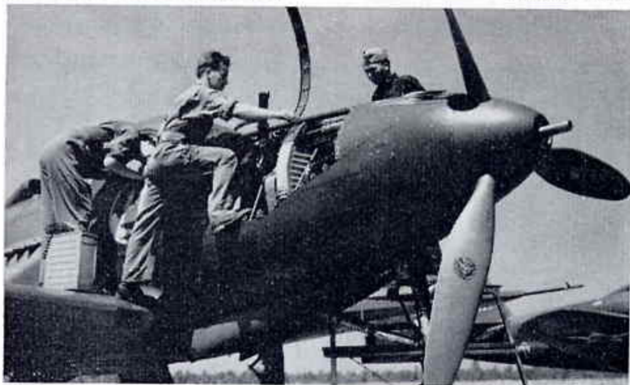
A P-39C of the 39th Squadron, 31st Pursuit Group, being rearmed; note details of the .30 cal., .50 cal., and 37 mm. cannon guns in the cowling and nose. (Photo: Bell)
