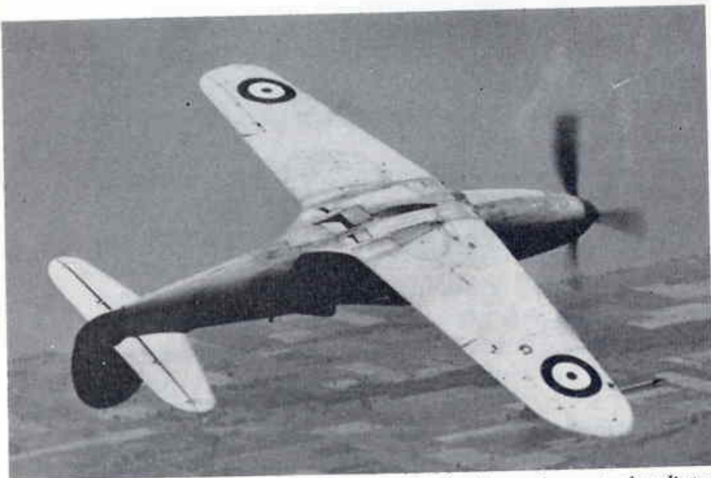
An R.A.F. Airacobra in inverted flight shows the central radiator exit door and the two oil cooler doors. (Photo: Bell Aerospace Corp. via F. H. Maupin)
