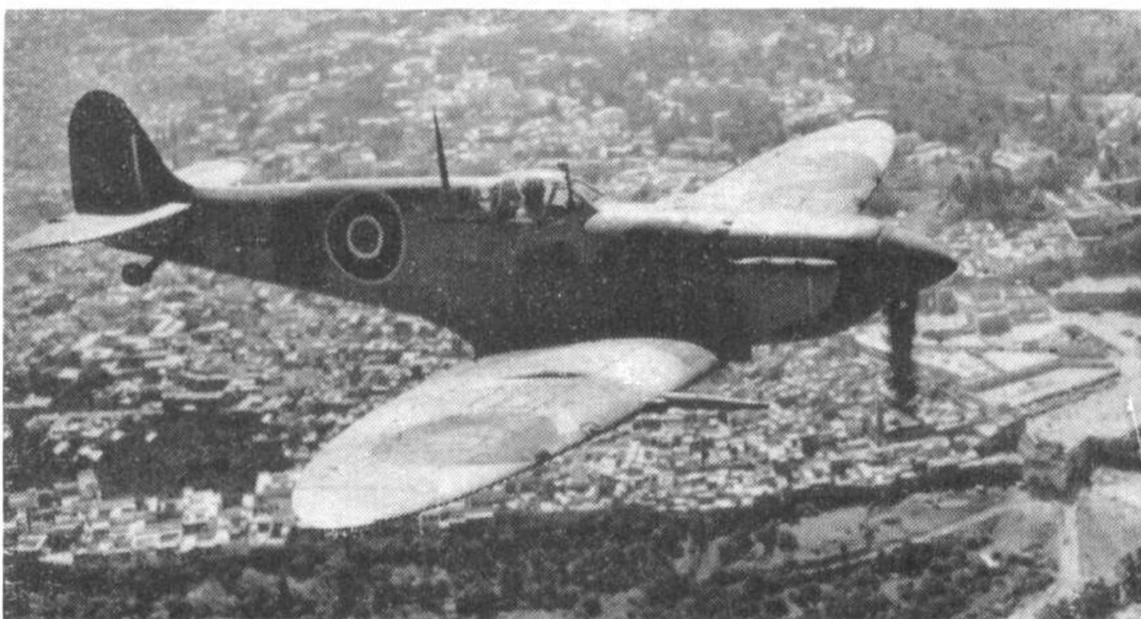
A late-production Spitfire Vc, MA859, on a delivery flight over Morocco; note the absence of a tropical filter. (Photo: Imp. War Mus.)
