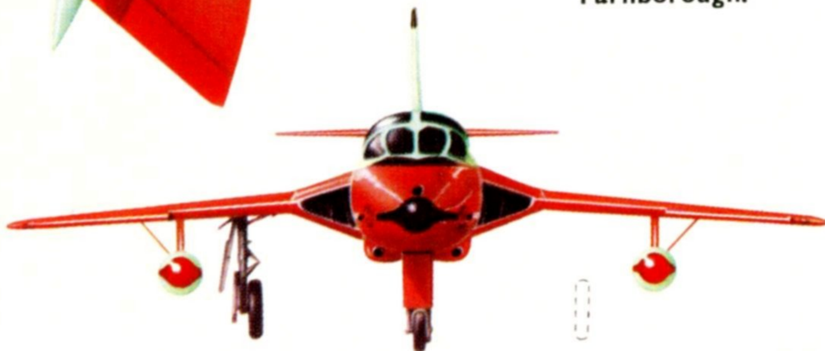
Aircraft, equipped with 350-gallon ferry tanks, as demonstrated by A. W. ("Bill") Bedford, O.B.E., at the 1960 S.B.A.C. Air Display, Farnborough.
