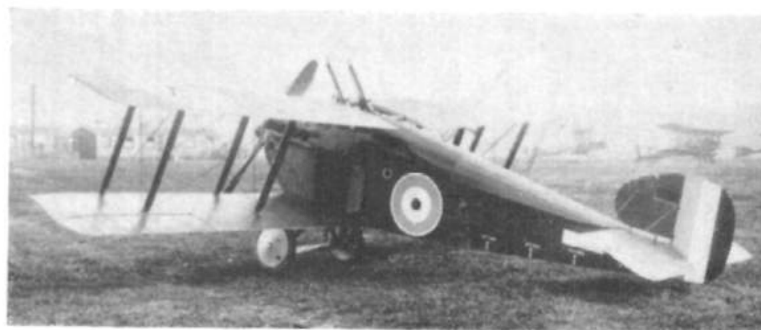
The third prototype at Brooklands. This aircraft had flank radiators on the fuselage sides, twin Lewis guns on the front spanwise member of the wing attachment frame, a small spinner, and a further revision of the fin and rudder.
