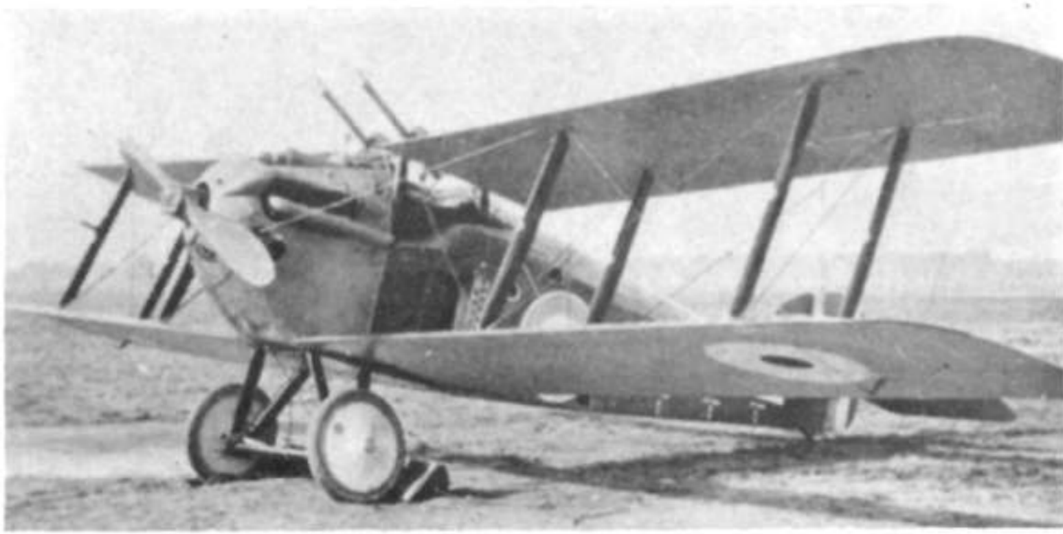
The third prototype at Martlesham Heath, showing the flank radiators. When this photograph was taken the aircraft did not have its spinner.
