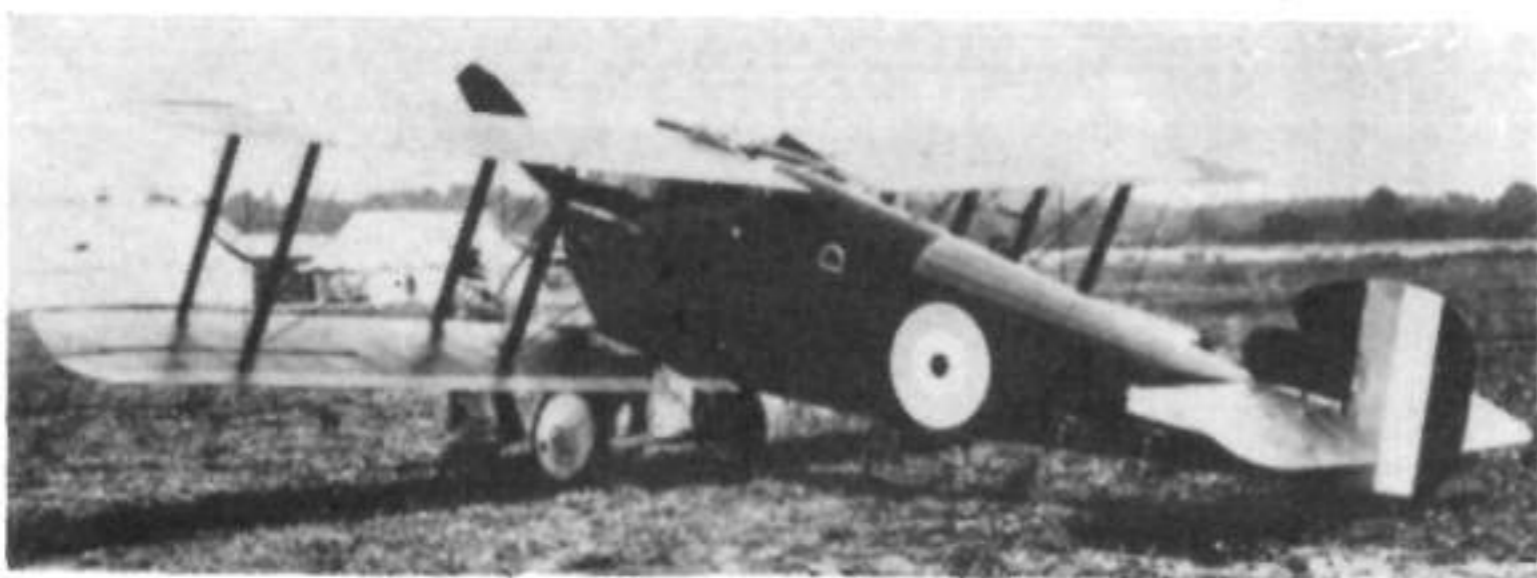
This three-quarter rear view of the second prototype illustrates the revised form of fin and rudder fitted to the aircraft. The streamlined header tanks for the wing radiators can also be seen at the upper wing roots.
