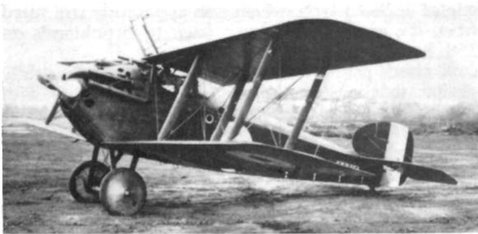
Standard production Dolphin with full armament. The production aircraft was virtually indistinguishable from the fourth prototype, but had steel-tube undercarriage V-struts and the structure of the fin and rudder was modified.
