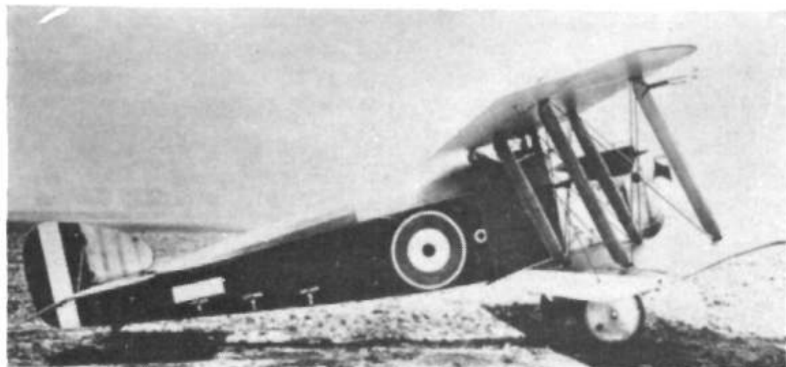
The first Dolphin at Martlesham Heath, with extended plywood decking behind the cockpit. The fin had apparently been recovered, as the Sopwith name was absent at this time.
