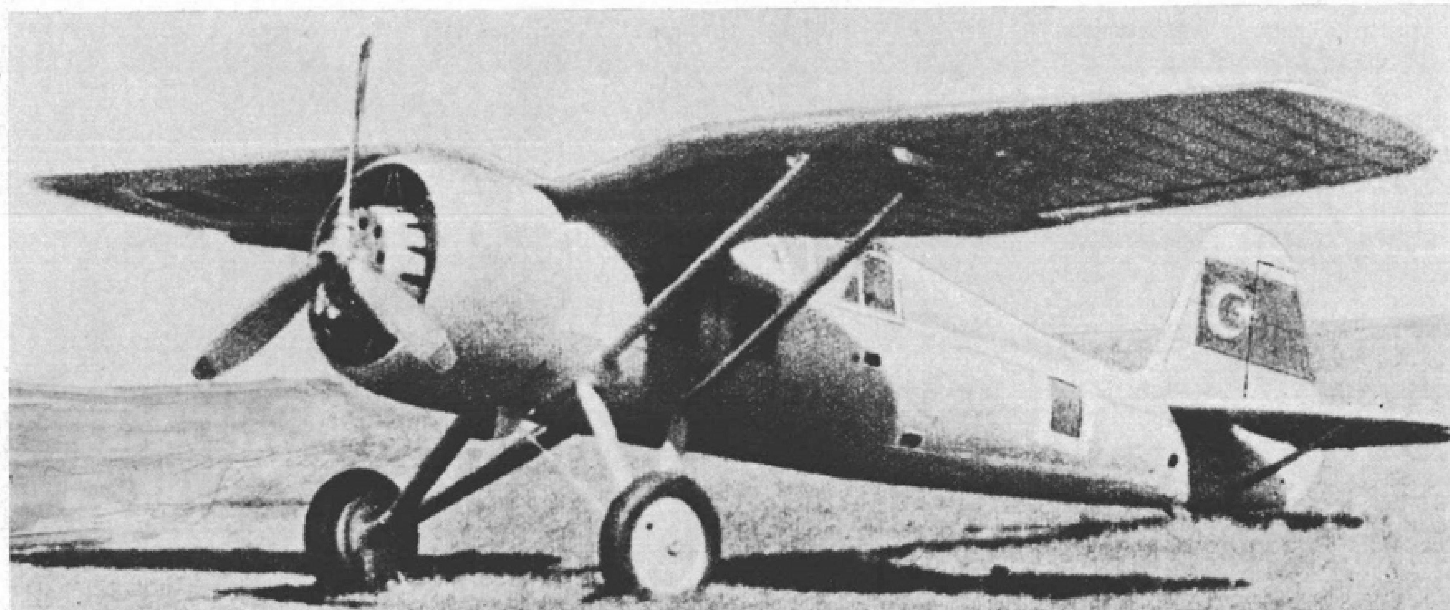
This Turkish-built P.24G has been re-engined with a Pratt & Whitney Twin Wasp and is now preserved at the Etimesgut training centre.
