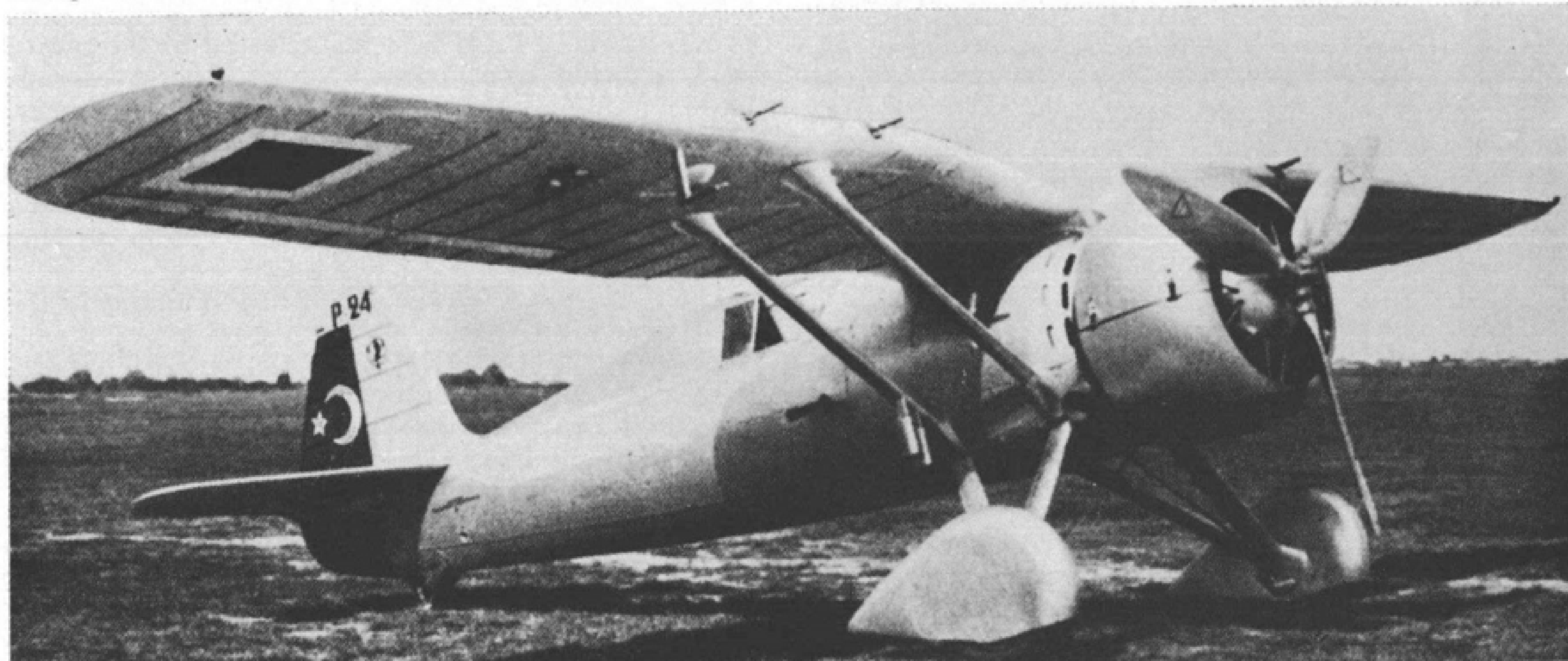
Late production P.Z.L.-built P.24C showing details of the wing-mounted guns and the airspeed indicator venturi.
