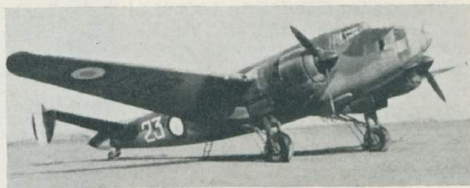
Two LeO's at Istres in 1940 after the Armistice, (left) an aircraft of 1st Escadrille, G.B.II/31 with the fuselage roundel painted out and a unit insignia in its stead, and (right) one of G.B.I/12's aircraft showing the fairing for the fixed forward-firing machine-gun located on the starboard side beneath the cockpit. (Photo: above: E.C.A.)
