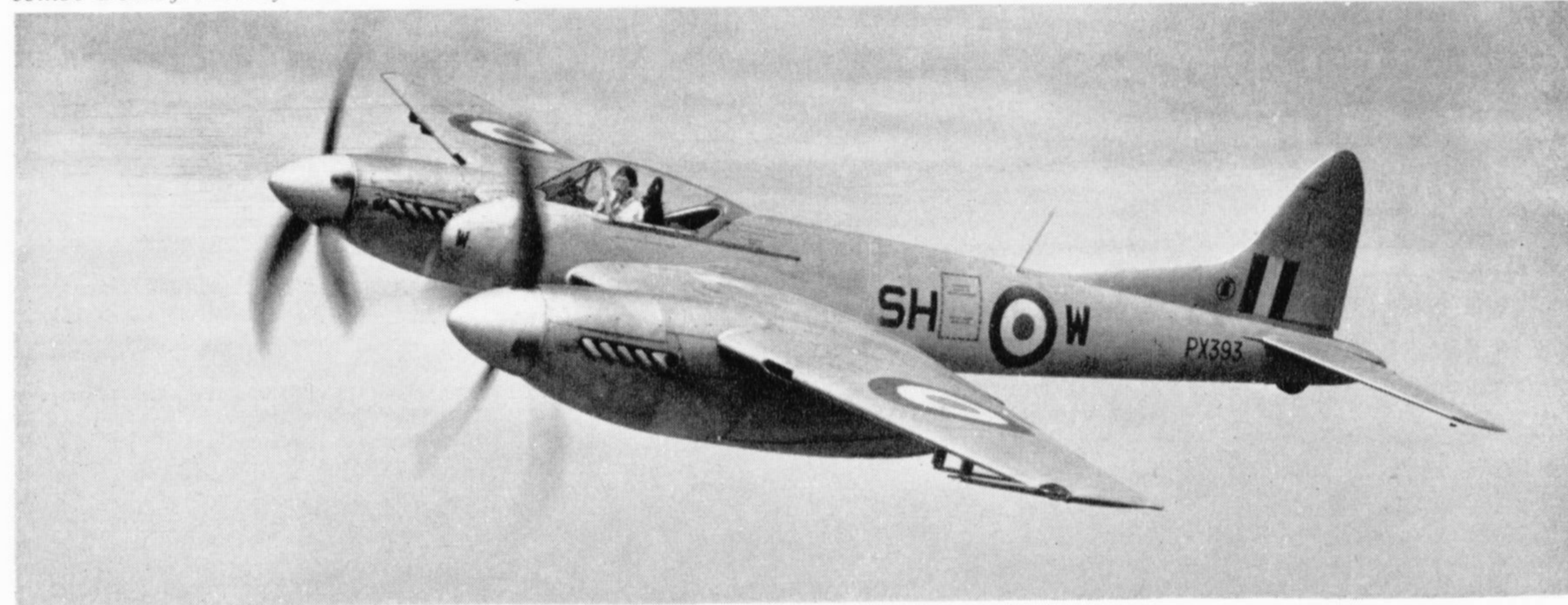
Hornet F. Mk. 3 PX393 of No. 64 Squadron in silver finish and late-style national markings. Individual letter on nose, unit emblem on base of fin and underwing rocket rails are all apparent, as is contra-rotation of the airscrews. The aircraft was based at Boscombe Down from July 1949 until February 1951.
