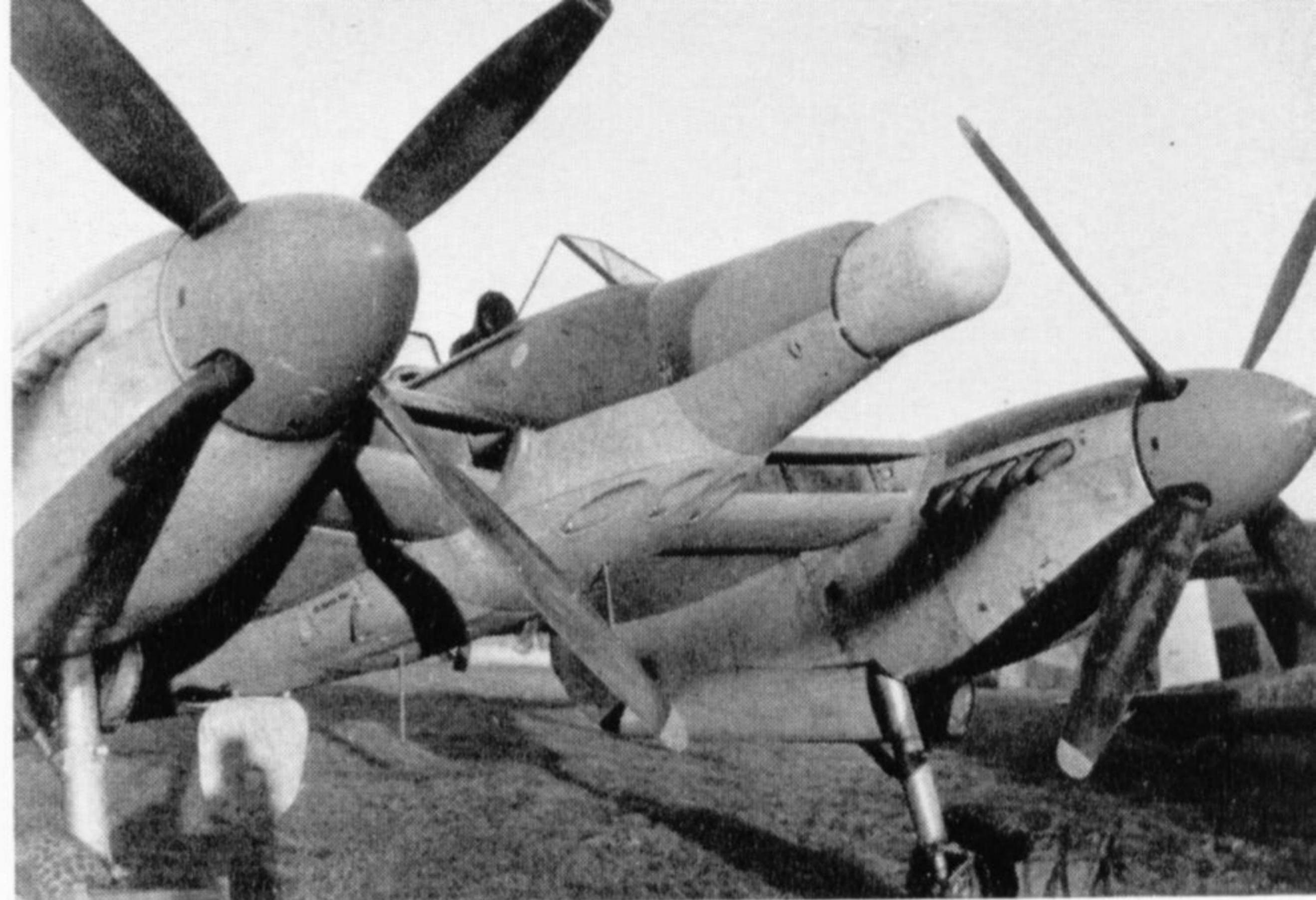
Sea Hornet N.F. Mk. 21 prototype PX230 showing nose "thimble" radome installation.
