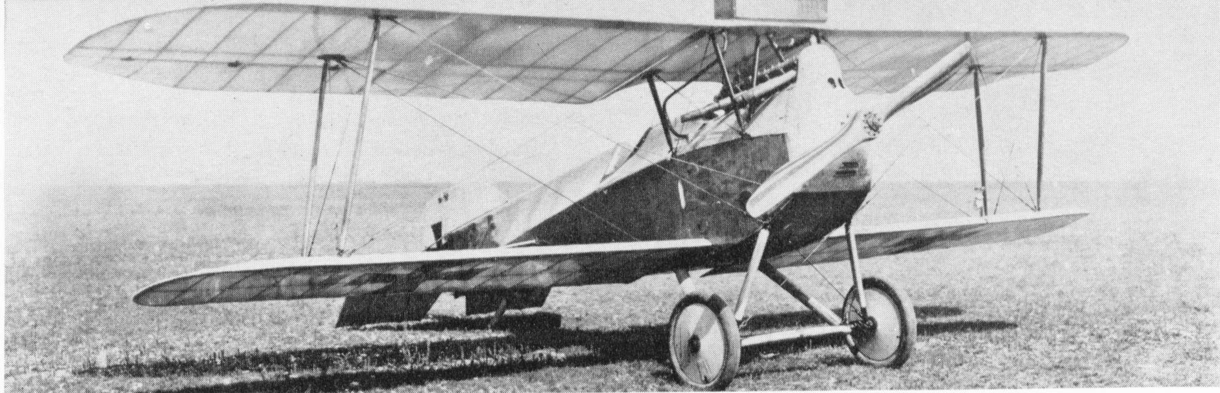
Phönix 20.16 (185 h.p. Austro-Daimler) seen, after rebuilding as the D.I prototype, fitted with strengthened wings.
