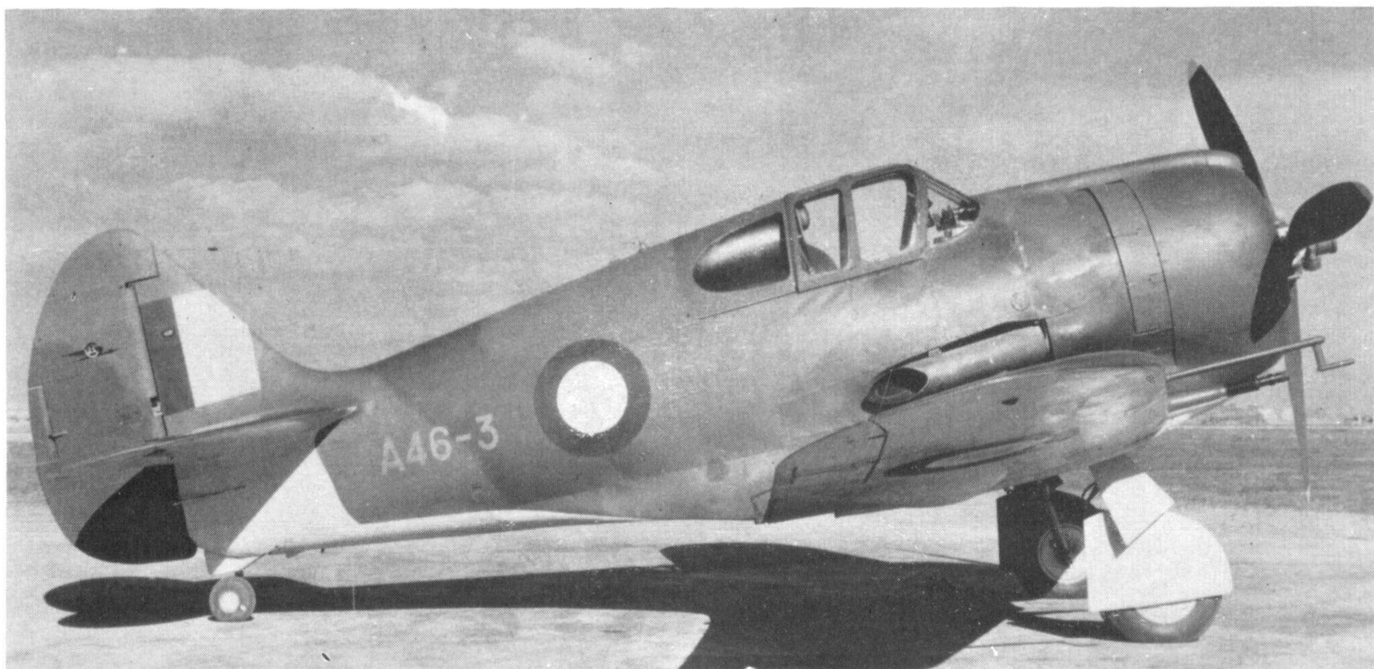
This view of A46-3 clearly shows the straight-through exhaust characteristic of the CA-12. (Photo: Australian War Memorial)
