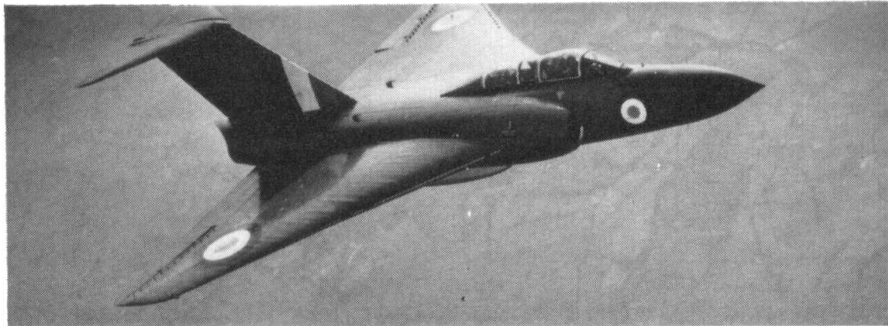
Two flying studies of the F.(AW) Mk. 4, distinguishable from the Mk. 1 by the two fuel simulator pressure heads on top of the fuselage.
