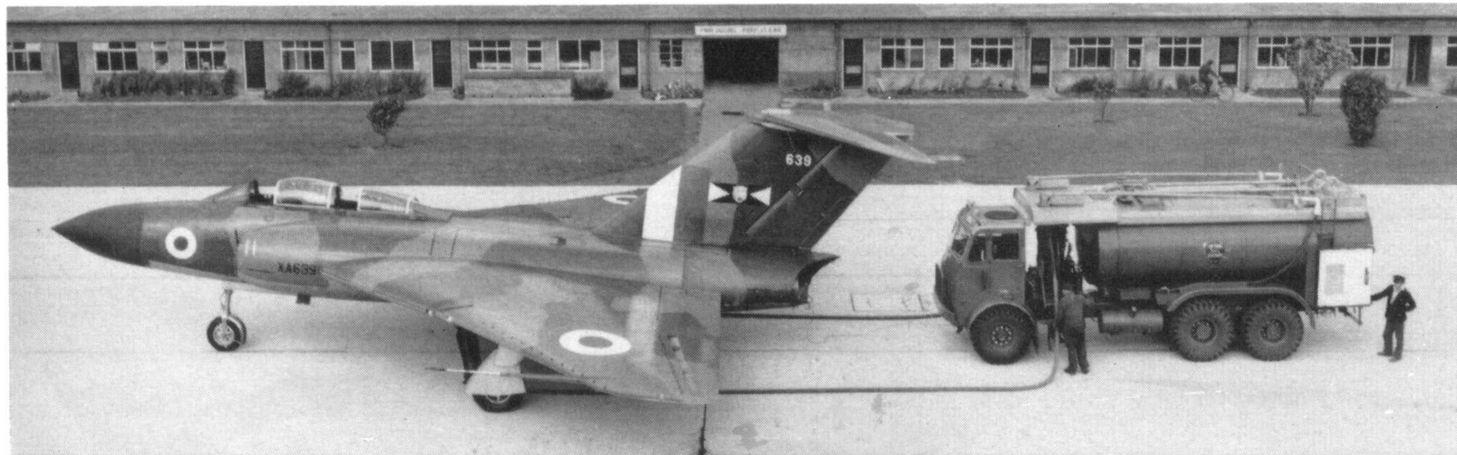
A Javelin Mk. 4 being pressure-refuelled; the twin hoses from the bowser connect to the refuelling couplings in the port and starboard wheel bays. (Photo: Min. of Defence)
