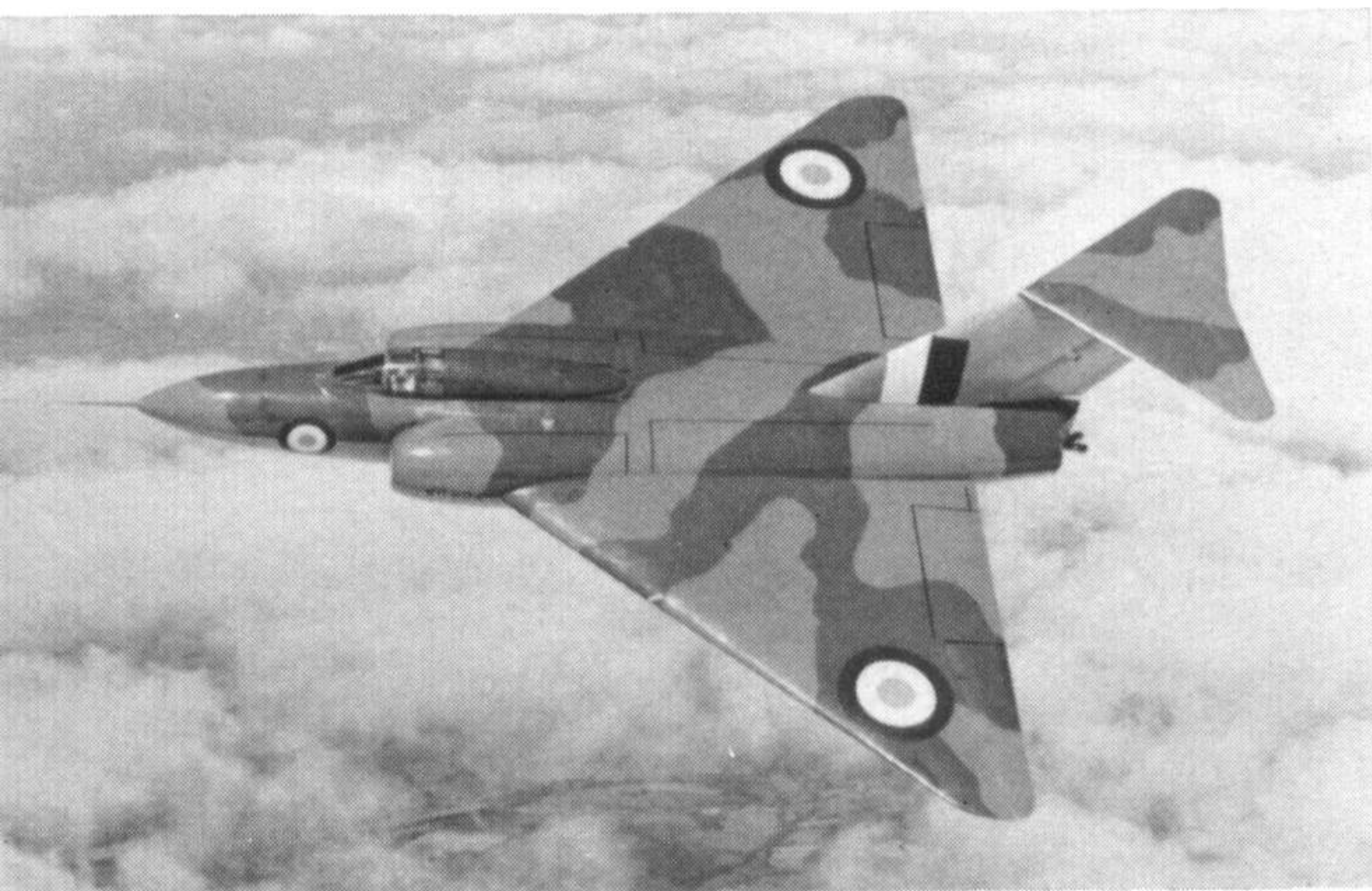
WD804, showing the original wing form with straight taper.
