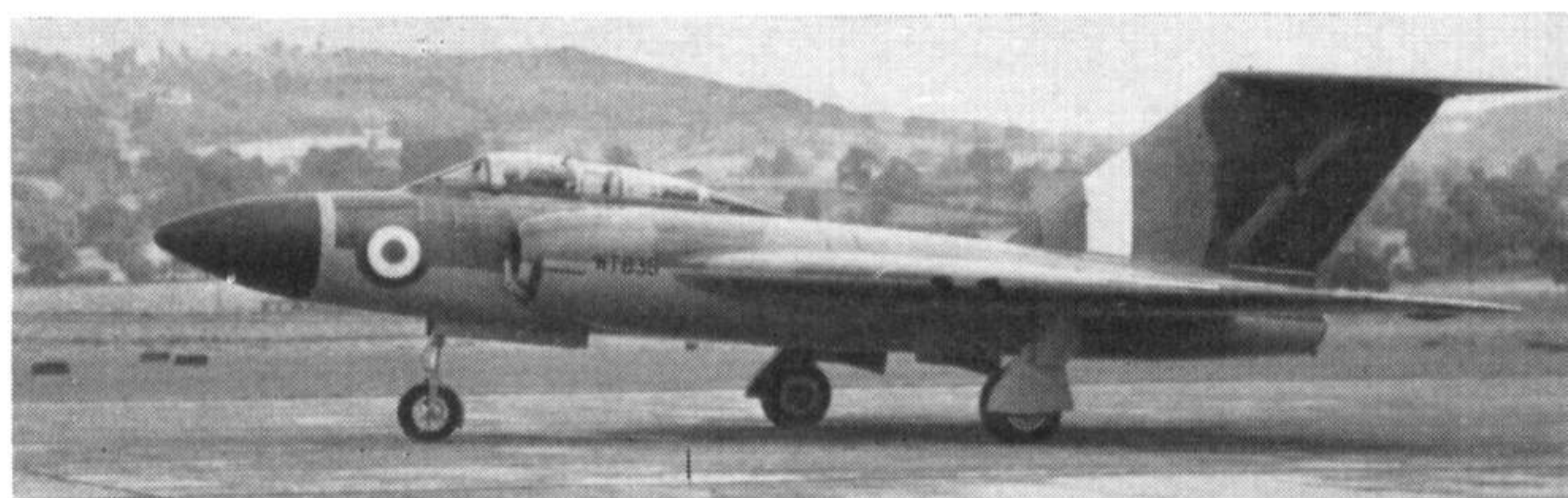
The fifth prototype WT836 on the runway at Hucclecote; this aircraft was the first to be fitted with the twin sliding hoods. The radome is of the original shape.
