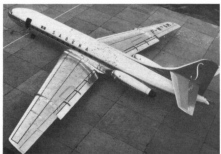
This bird's eye view of Sabena's OO-SRC (seen here before delivery) shows flap detail and the tail parachute doors. (Photo: U.S.I.A.S.)
