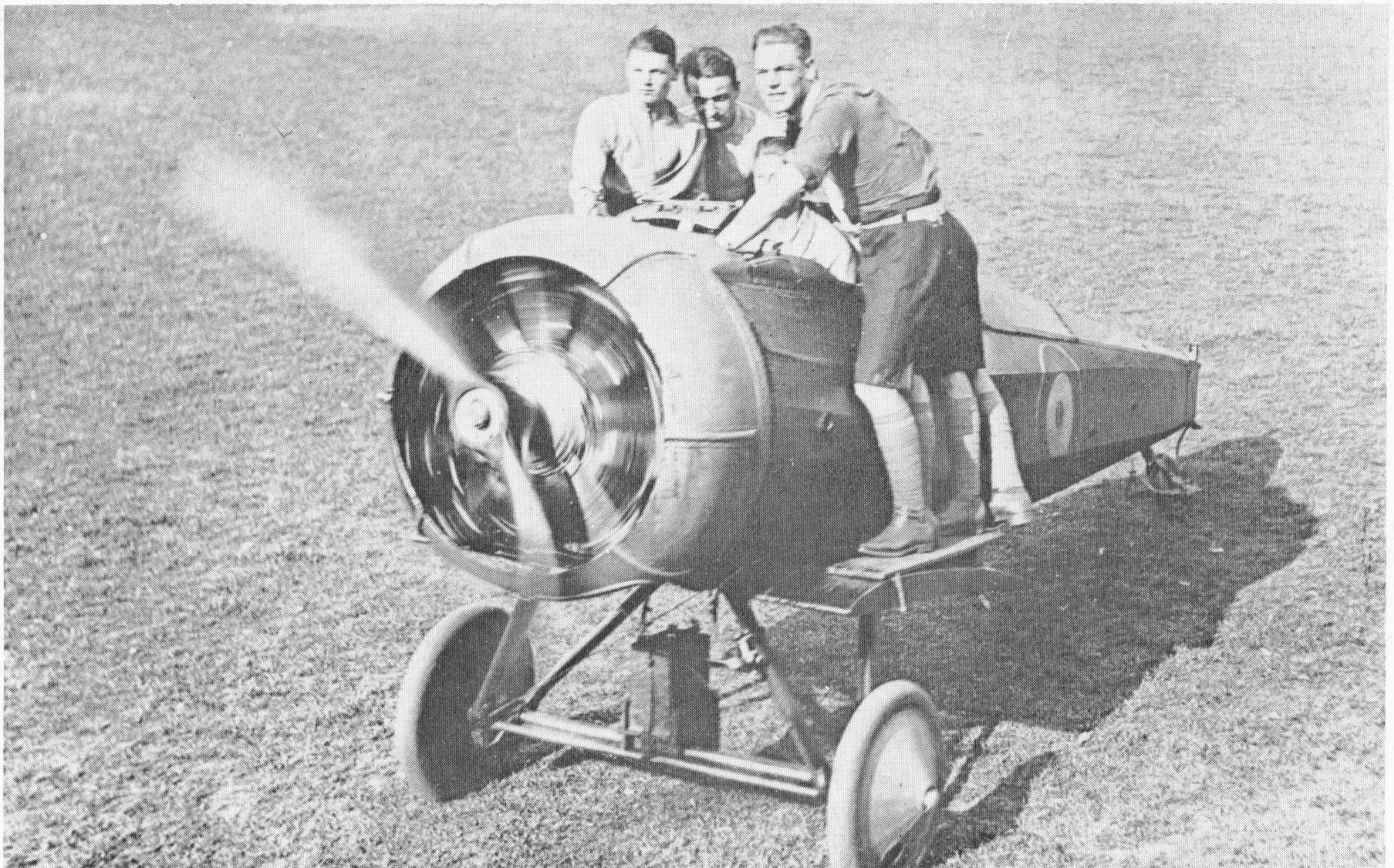
A D.H.5 fuselage in use as a taxiing trainer at No. 2 School of Military Aeronautics, Oxford. The frontal aperture of the cowling has been enlarged to aid cooling of the engine. (Photo: I.W.M. Q27249)
