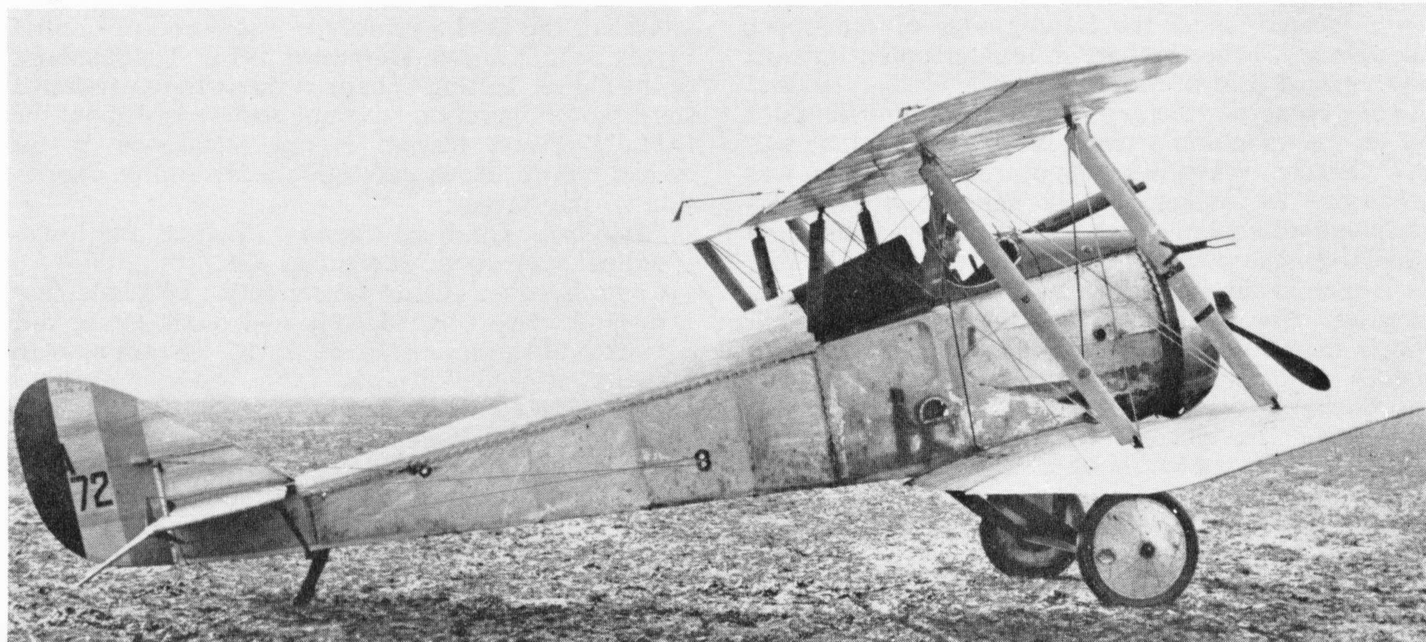
The modified prototype with enlarged rudder, strut-braced tailplane, and Vickers gun on elevating mounting. The serial number A5172 was carried on the rudder. The photograph was most probably made at Central Flying School while the D.H.5 was undergoing its official trials.
