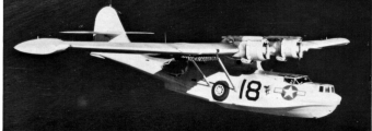
White and light grey PBV-5A of Patrol Bomber Squadron 63, the famous "Cowboys from Büttelsville", carrying retro-rockets under the wings. (Photo: U.S.N. via Donato)
