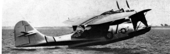
The moment of impact—a Coast Guard PB7-5A making a perfect full-stall landing. This is the technique a pilot would use for landing in the open sea. (Photo: Mitch Mayborn Collection)
