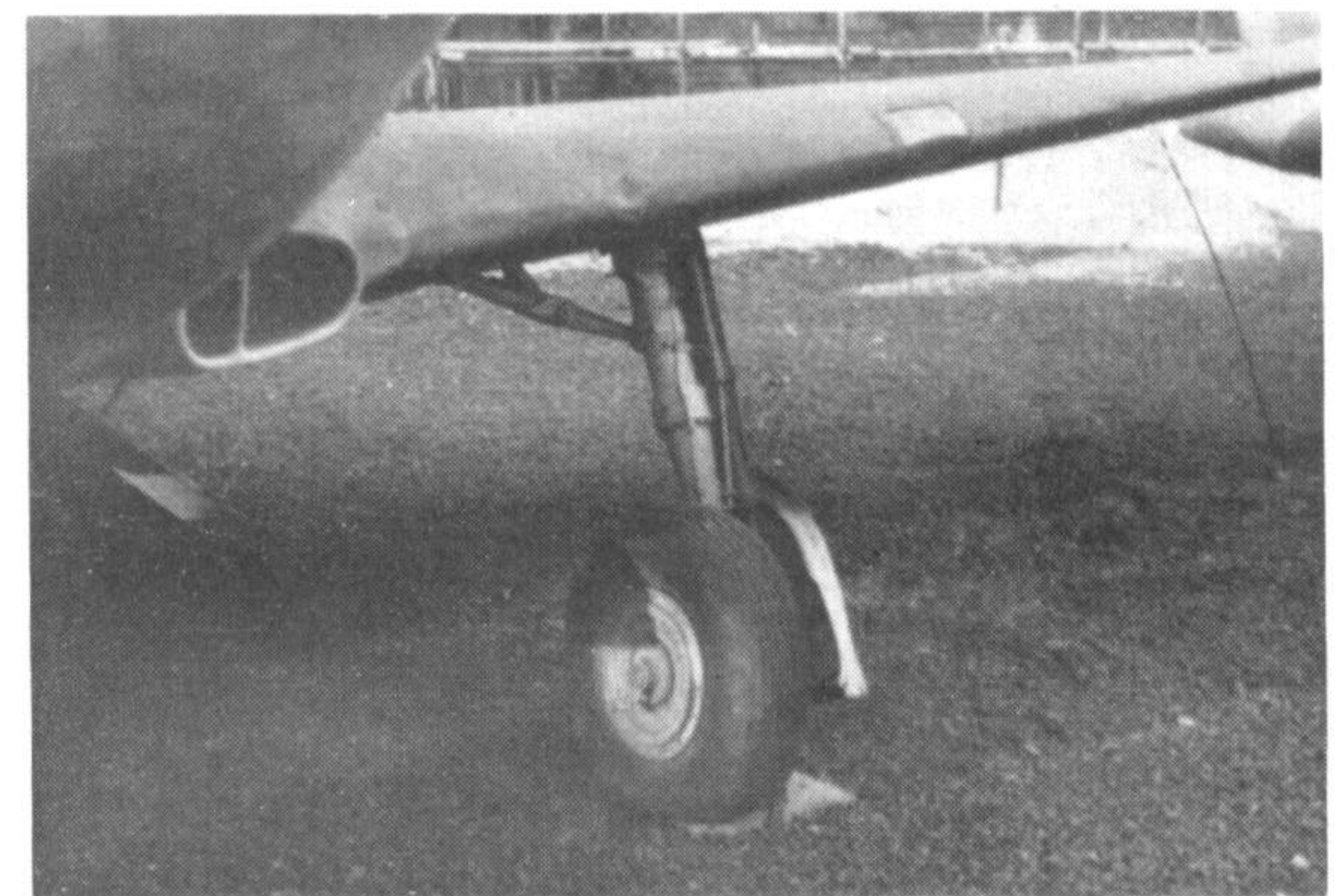
Close-ups of the Yak-9P in the Polish Armed Forces Museum, Warsaw: (top) engine cowling, showing breech and muzzle fairings of one of the machine-guns; (centre) tailplane and tailwheel; (bottom) oil cooler intake and port mainwheel leg. (Photos: the author)
