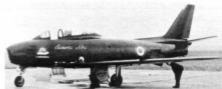
An F-86E(M), ex-Mk. 4, of the Italian Aeronautica Militare in the markings of the Lancero Neri aerobatic team.
