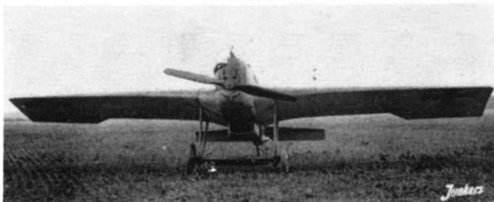
Front view of E 252/16, first of the modified J-2's; the pylon above the port wing carried pitot/static test instrumentation.
