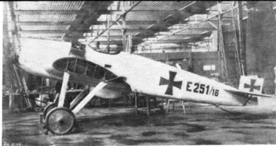
The J-2, E 251/16, immediately before wing mating; note semi-monocoque fuselage, fully-cowled engine and underlung radiator. Armament was to comprise a single synchronised Spandau partly faired into the upper starboard cowling.
