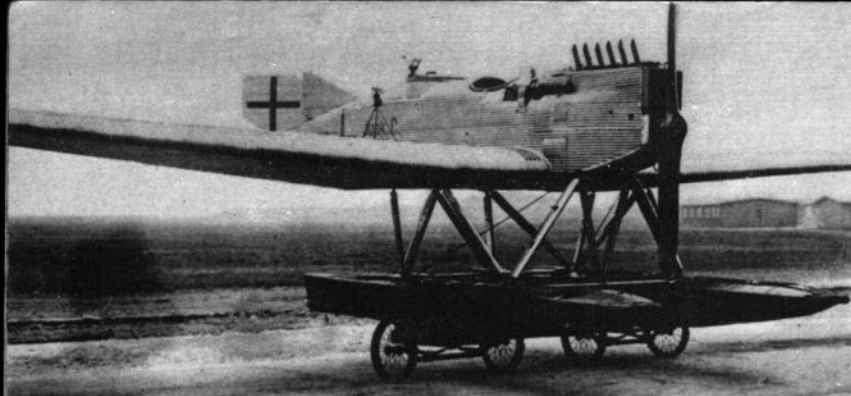
(Above) The first of three Junkers J-11 floatplanes constructed for the German Navy; note low aspect ratio rudder, and incorrect fuselage legend "Junk.C.". The correct form should have read "Junk.C3MG 7501/18". (Below) A J-11/C3MG photographed in spring, 1919, with taller, definitive, rudder. Lack of armament and presence of British Naval officer (in white cap-cover) suggests that this was one of the hundred aircraft that the German Navy was permitted to retain for mine-spotting patrols.
