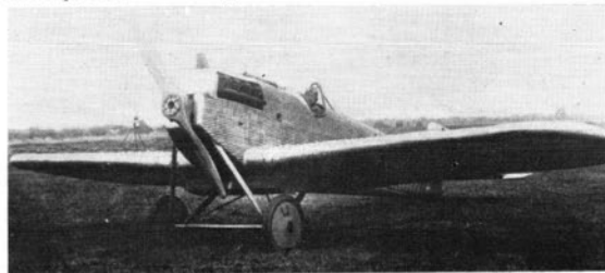
One of the early batch of long-fuselaged J-9's, this machine was fitted with a higher-powered Benz Bz IIIa engine developing 200 h.p. Note underwing radiators. (Photo: via J. M. Bruce)
