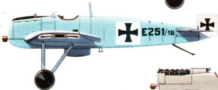
Junkers J.7, with engine installation as it appeared after January 1918.
