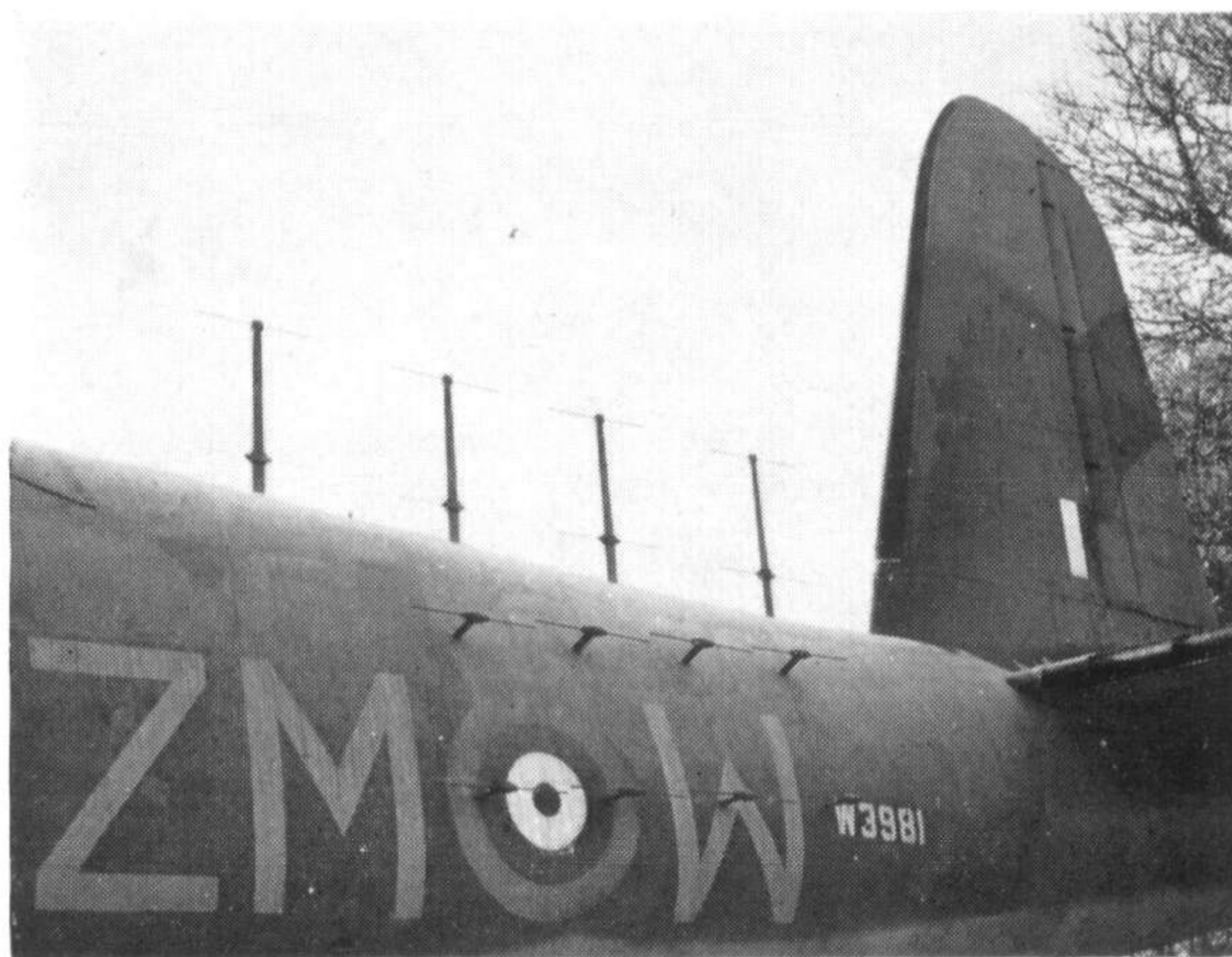
The Botha-type dorsal turret of a Mk. II and (above) ASV Mk. II radar fitted to a Sunderland Mk. II, in this case W3981 of No. 201 Sqn. (Photos: Short Bros. & Harland)
