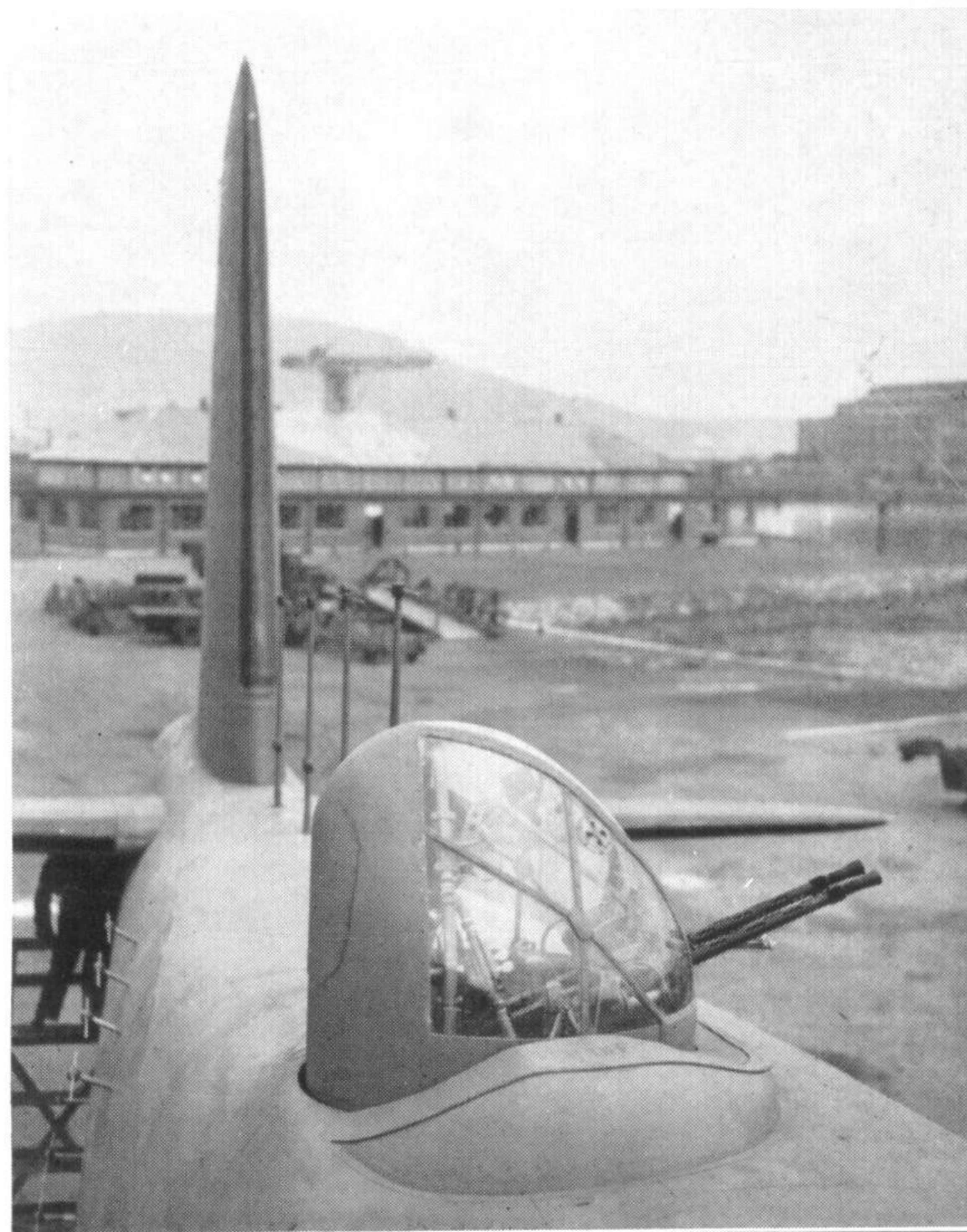
The Botha-type dorsal turret of a Mk. II and (above) ASV Mk. II radar fitted to a Sunderland Mk. II, in this case W3981 of No. 201 Sqn. (Photos: Short Bros. & Harland)
