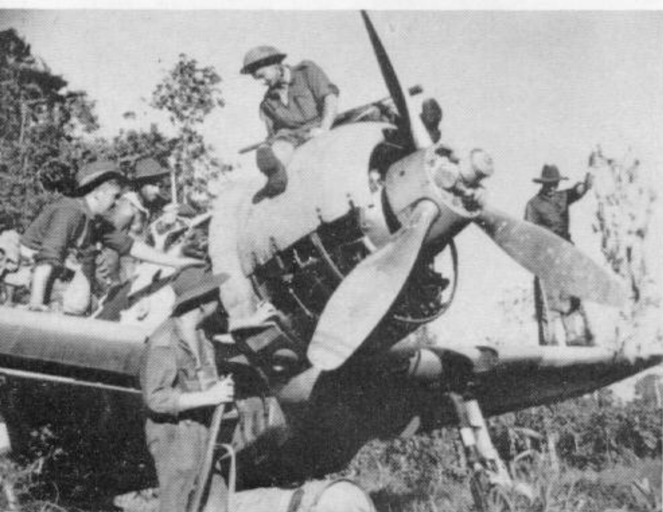
Cowling and propeller details of a disabled Model 32 Reisen captured by Australian troops at Lae, New Guinea. For some reason the cowling of this machine has not been painted the customary black. (Photo: Australian War Memorial)
